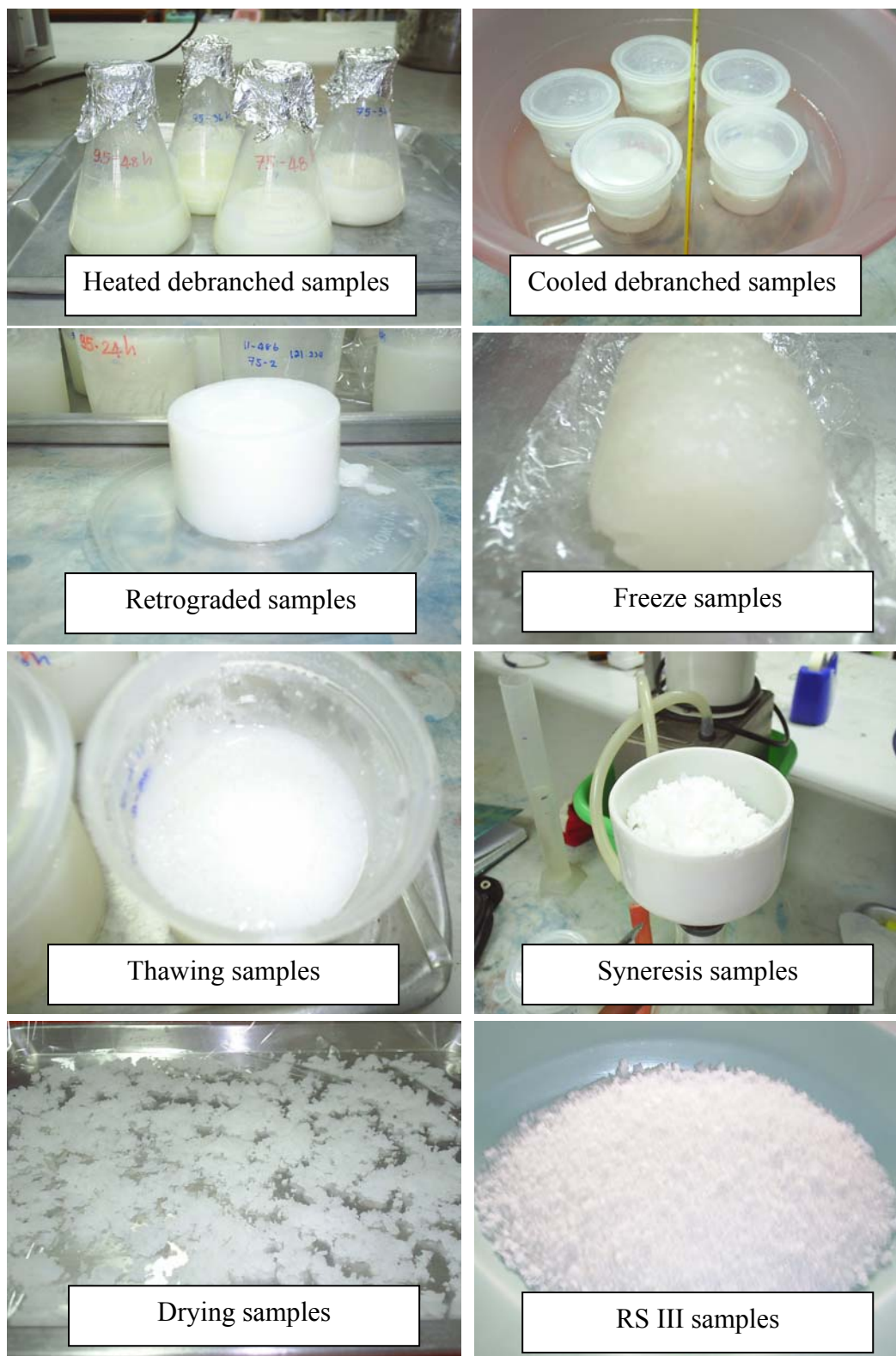
Appendix Figure C2 Visuals appearance of RS III samples with various processing Steps
