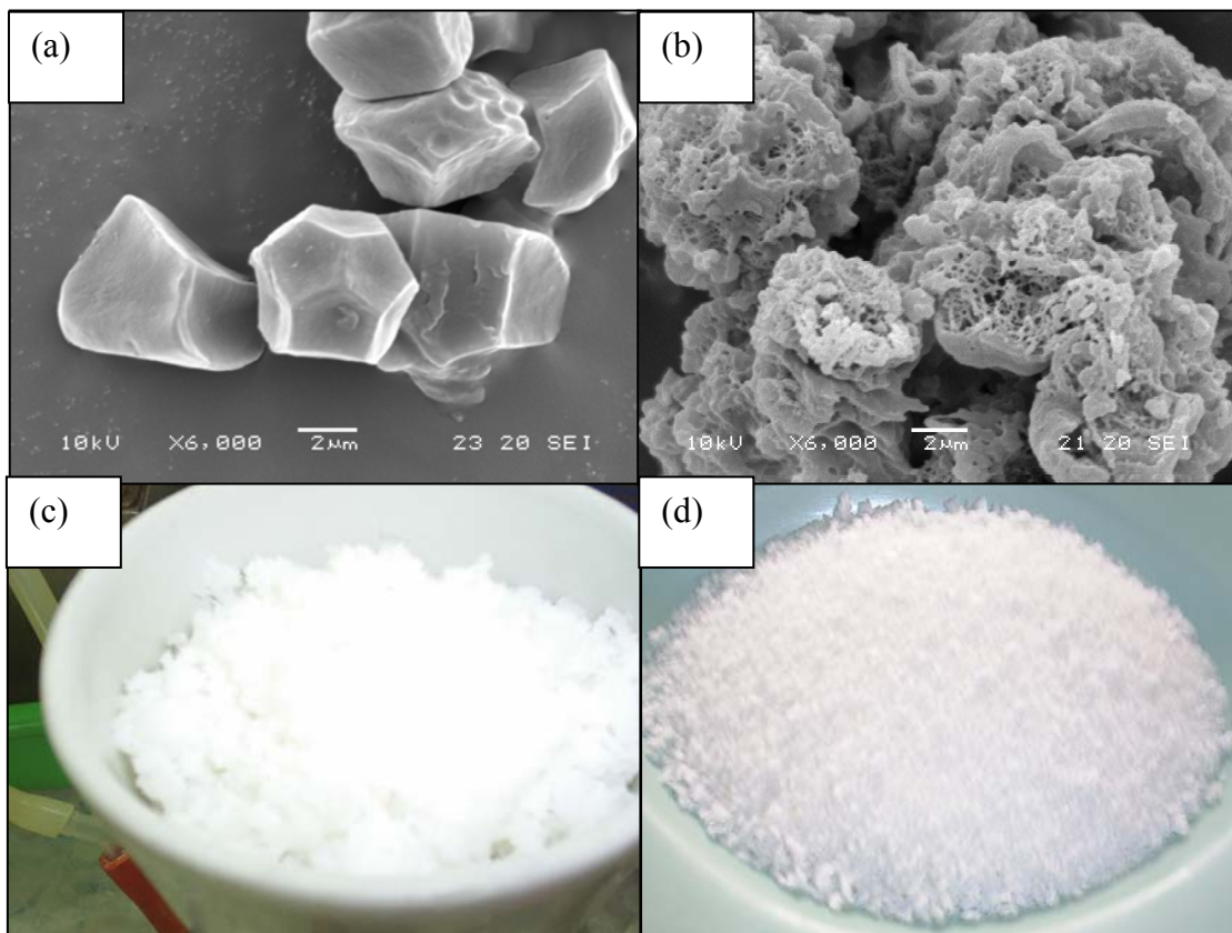
Figure 19 Scanning electron micrograph of native (a), retrogradation rice starch (b) and typical appearance of fresh (c) and dried (d) retrograded from 16-hr debranching and retrogradation of high amylose rice starch
