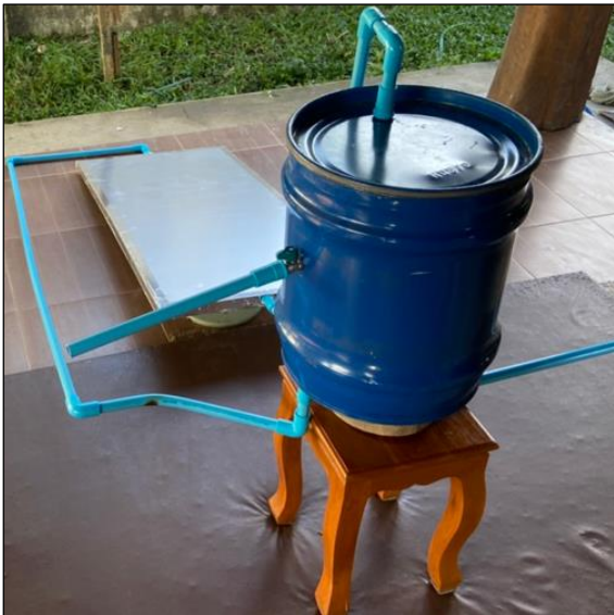
Figure 11 The proposed hot water system.
