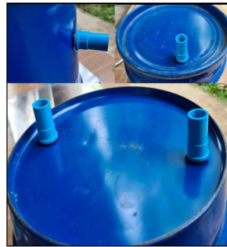
Figure 9 The holes of the hot water tank.
