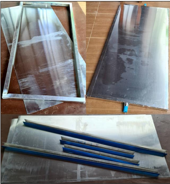
Figure 8 The proposed solar thermal panel and its built aluminum sheets.
