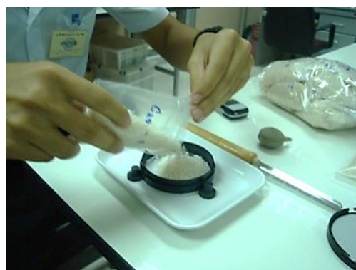
Figure 2 Pouring the rice samples into the closed cup for measuring the absorbance.
