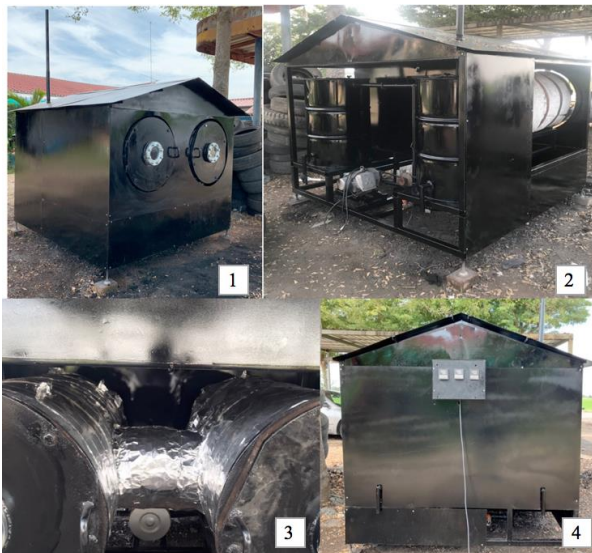
Figure 4 Carbonization reactor: 1. Carbonization chamber (Right) & Combustion chamber (Left) 2. Gas cleaning system 3. Insulation 4. Temperature monitor.
