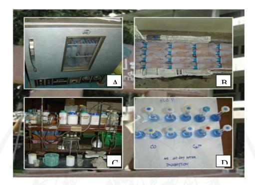
Appendix Figure 5 Setup for laboratory incubation experiment: (A) Soil samples in incubator;(B) Shaking soil samples; (C) Distillation apparatus for Nitrogen determination; and (D) Phosphorus determination by Bray II method
