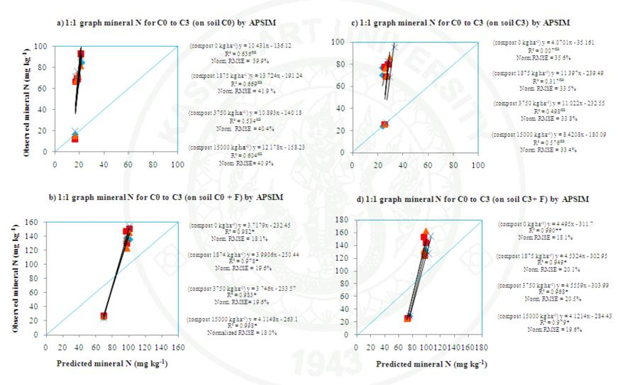
Figure 32 Relationship between simulated and observed mineral N of soil treated with 4 compost rates and 2 mineral fertilizer rates in the cases of soil with no previous compost application (a and b) and soil previously treated with 7500 kg ha<sup>-1</sup> compost (c and d) using APSIM. Compost: 0 kg ha<sup>-1</sup> (◆); 1,875 kg ha<sup>-1</sup> (●); 3,750 kg ha-1 (▲); and 15,000 kg ha<sup>-1</sup> (×).
