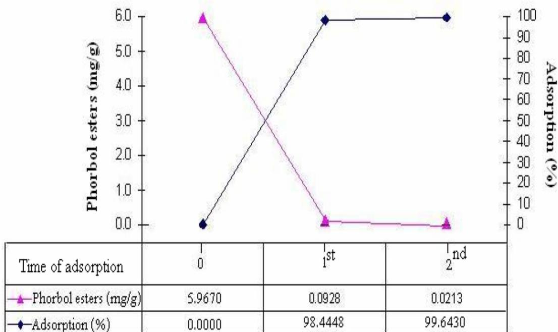
**Figure 32** One-time and two-time of adsorption capability of phorbol esters in seed oil.
