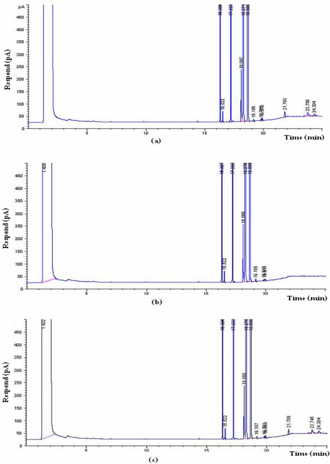
**Figure 37** Fatty acid composition chromatograms of *Jatropha* seed oil detected by GC; seed oil (a), one-time adsorption (b) and two-time adsorption (c).
