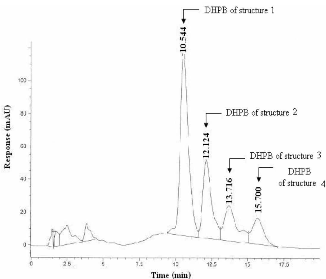
**Figure 23** Chromatogram of phorbol esters (DHPB) in *Jatropha* seed oil analyzed with photodiode array detector (PDA).
