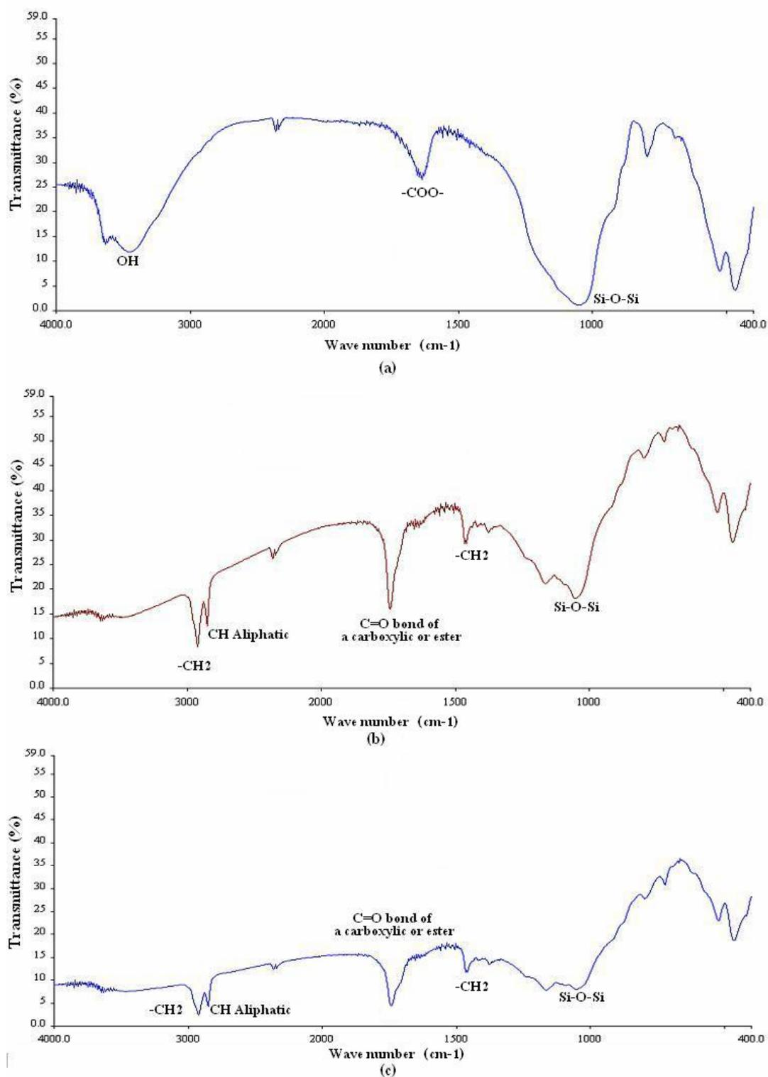
**Figure 36** Spectrums of bentonite 200 detected by Fourier transform infrared spectrophotometer (FT-IR); bentonite 200 (a), one-time adsorption (b) and two-time adsorption (c).
