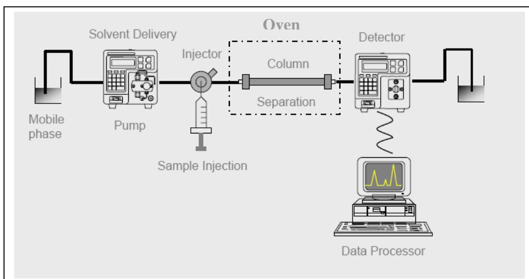
**Figure 12** Schematic diagram of an HPLC instrument.
