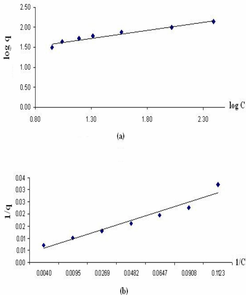
**Figure 33** Adsorption isotherms of phorbol esters from *Jatropha* seed oil by bentonite200 (the one-time); Freundlich isotherm (a) and Langmuir isotherm (b).
