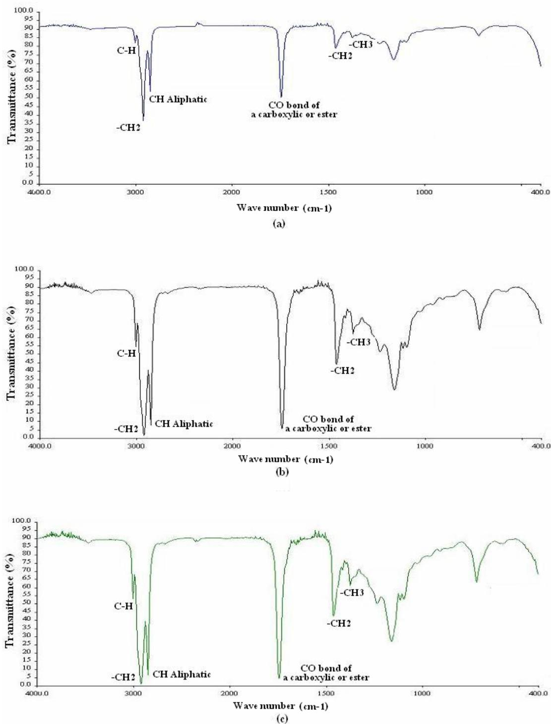
**Figure 35** Spectrums of *Jatropha* seed oil detected by Fourier transform infrared spectrophotometer (FT-IR); seed oil (a), one-time adsorption (b) and two-time adsorption (c).
