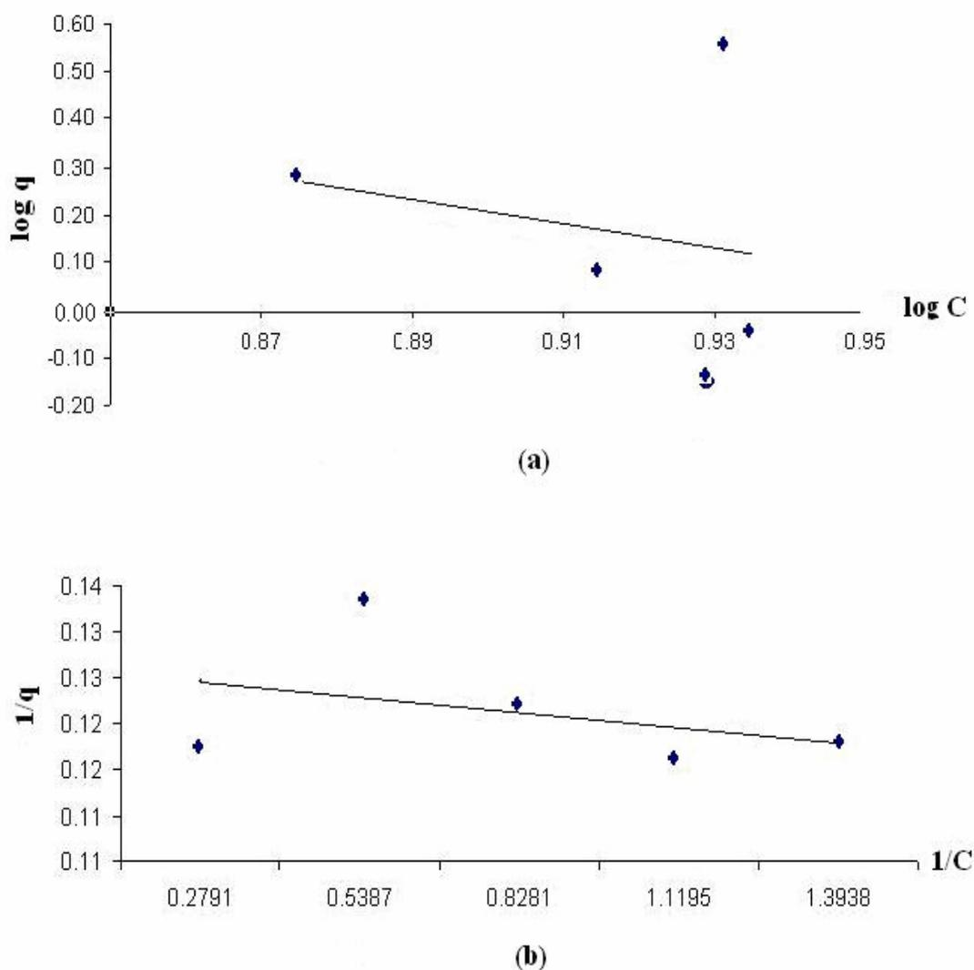
**Figure 34** Adsorption isotherms of phorbol esters by bentonite200 (the two-time); Freundlich isotherm (a) and Langmuir isotherm (b).
