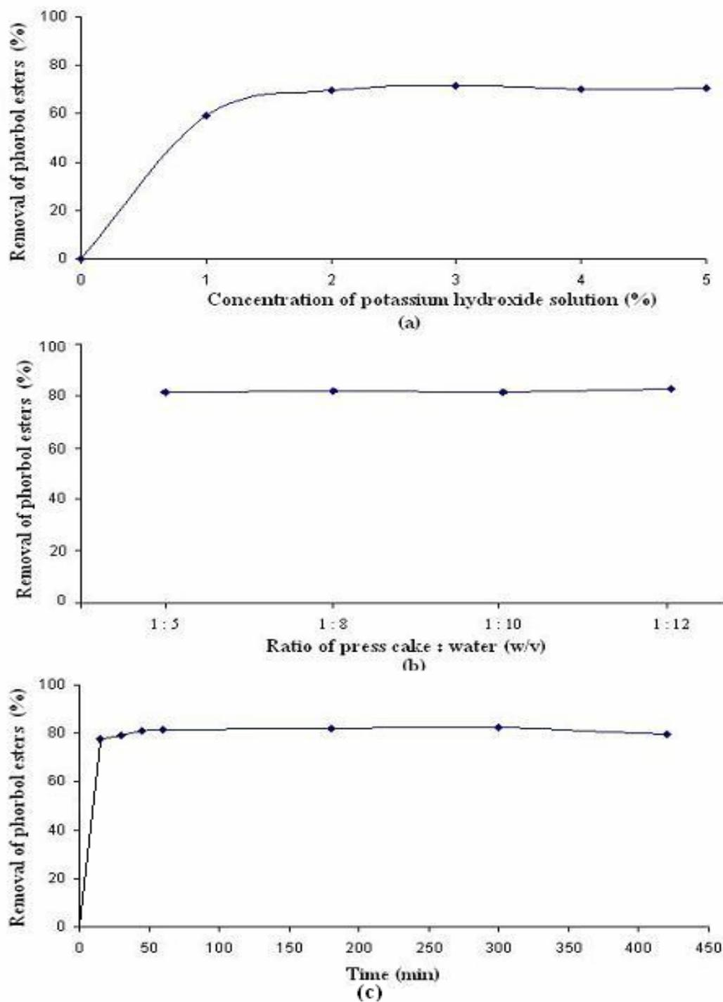
**Figure 39** The effect of KOH concentration (a), press cake to water ratio (b), stirring time (c), stirring rate (d) and temperature (e) on removal percentage of phorbol esters in press cake.
