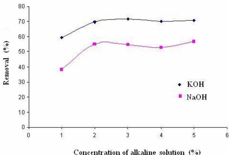
**Figure 38** Removal capabilities of phorbol esters from *Jatropha* press cake by base solution treatment; KOH and NaOH solutions.
