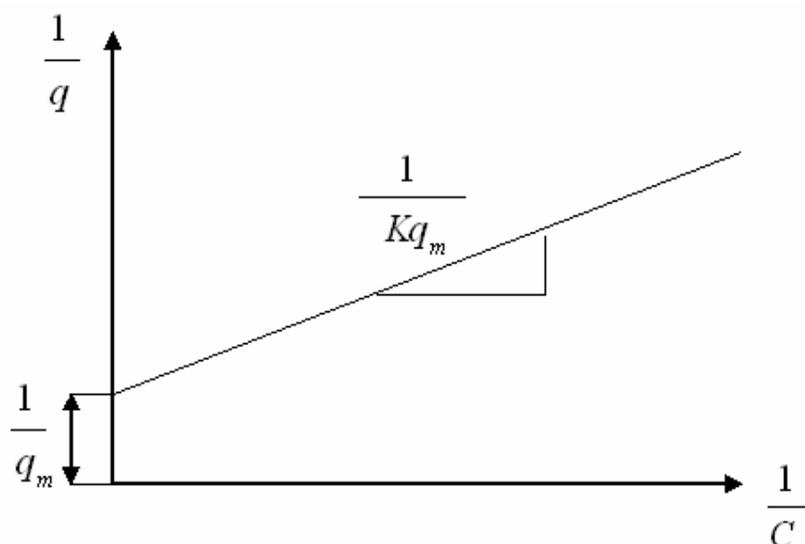
**Figure 9** Langmuir isotherm of linearization.
