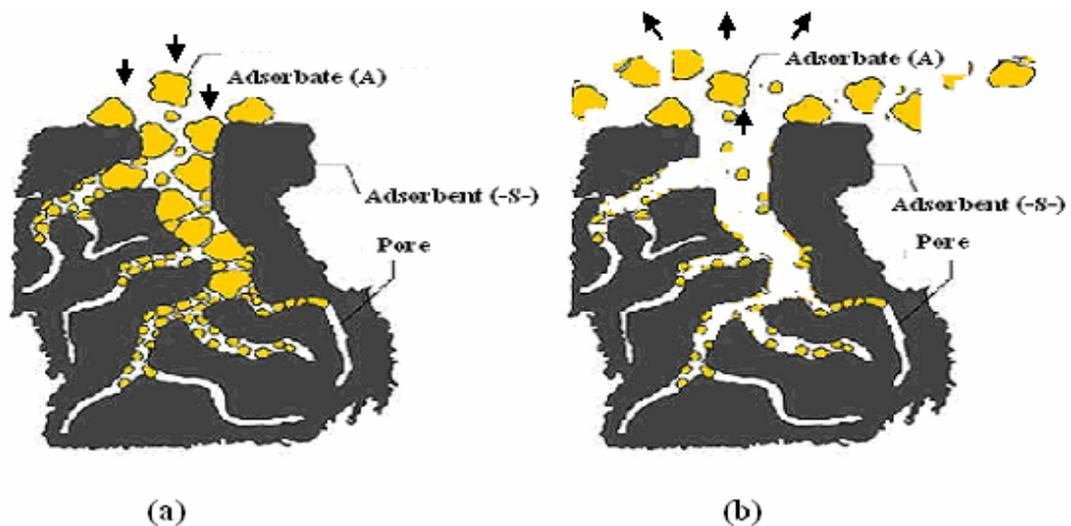
**Figure 7** Two characterizations of adsorbate on adsorbent; adsorption (a) and desorption (b).
