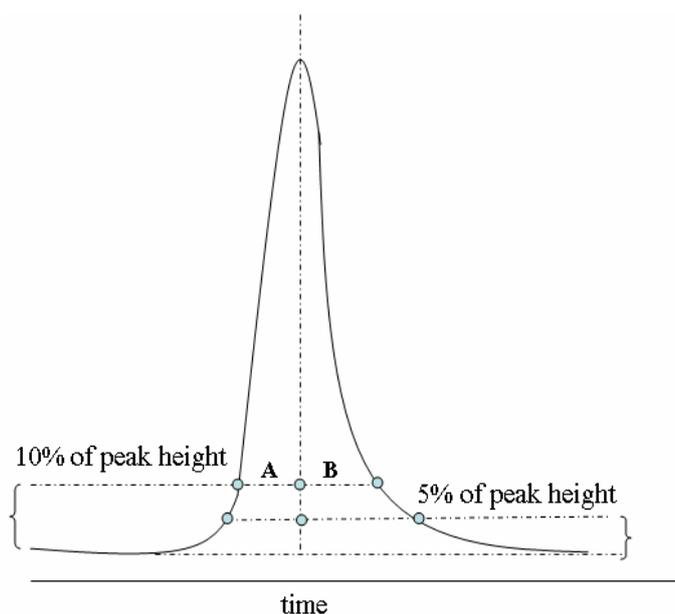
**Figure 11** Determining peak-asymmetry and peak-tailing factor. Peak asymmetry =  $B/A$  and peak tailing factor =  $(A+B)/2A$ .
