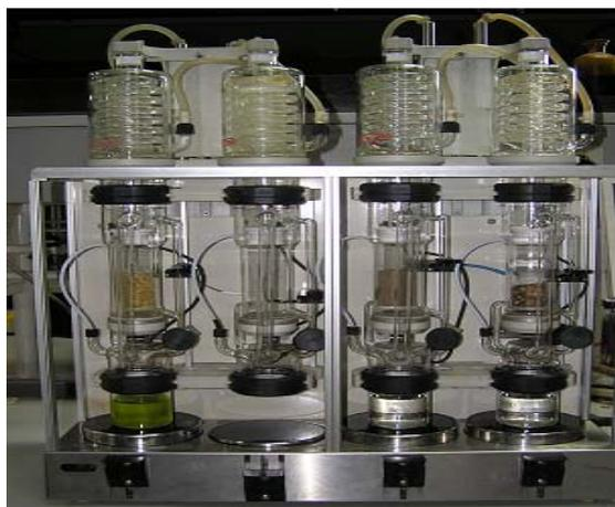
**Figure 14** Phorbol esters extraction from solid samples (i.e. kernels, bark, fruit bark, etc.) with soxhlet apparatus.
