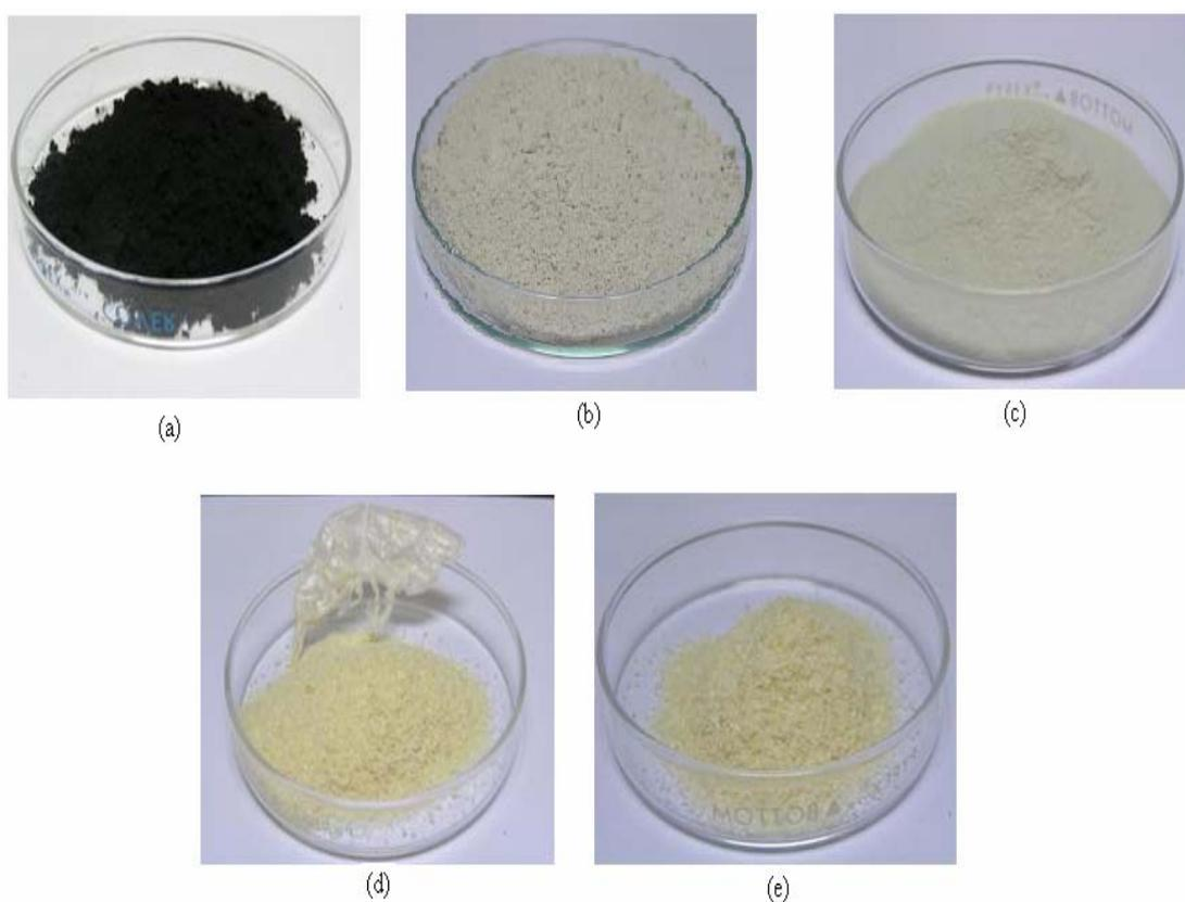
**Figure 18** The adsorbents of Activated carbon (a), Bentonite 150 (b), Bentonite 200 (c), Chitin (d) and Chitosan (e).
