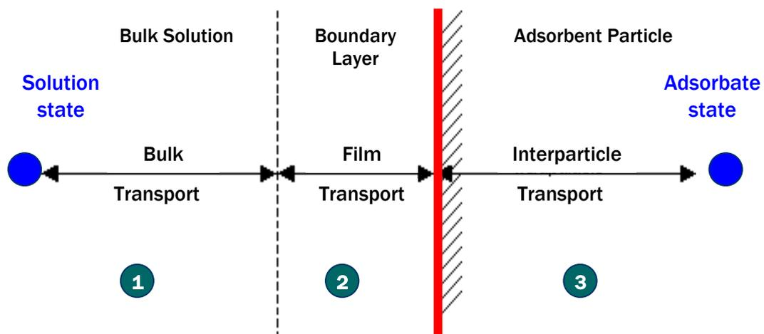
**Figure 6** Adsorption process on a porous adsorbent proceeds in three consecutive steps; (1) Bulk transport, (2) Film transport and (3) Interparticle transport.
