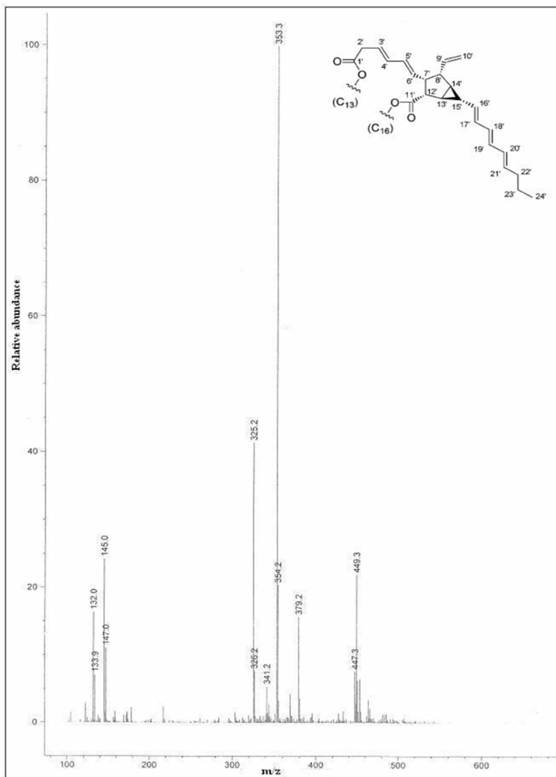
**Figure 25** Combination HPLC/PDA/MS of phorbol esters extracts on peak at the retention time of 12.124 min.
