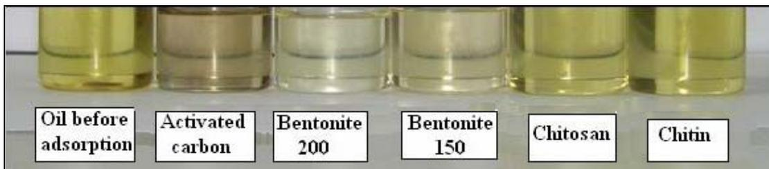
**Figure 19** Comparison of *Jatropha* seed oil before and after adsorption with adsorbents.
