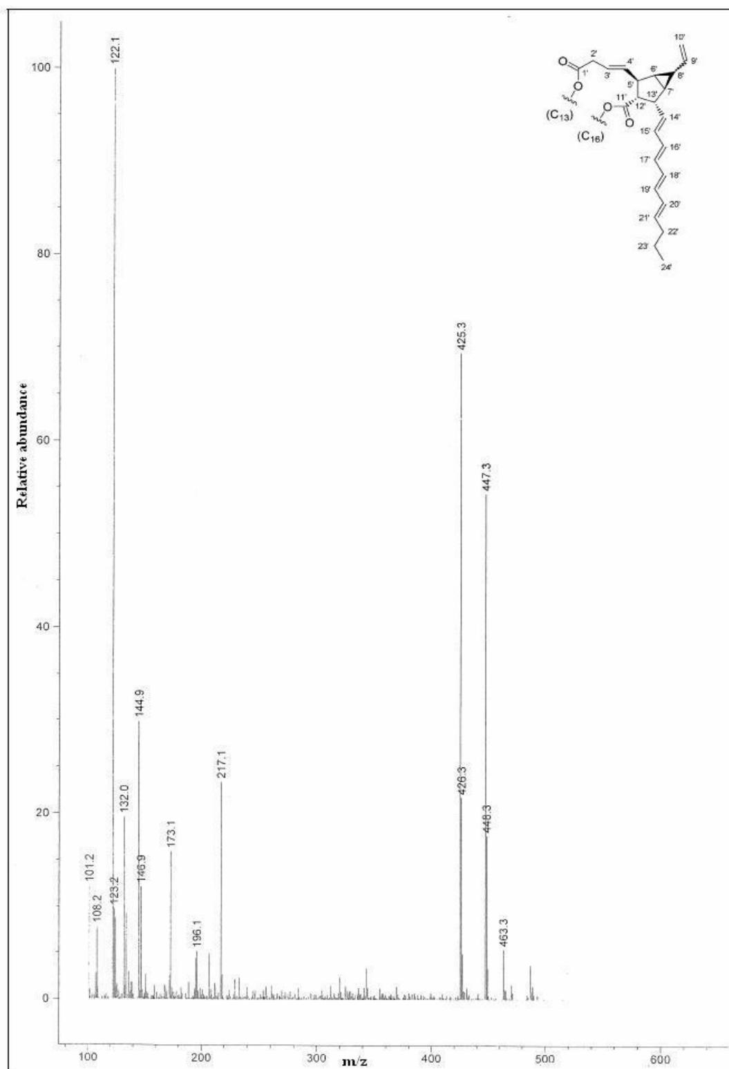
**Figure 27** Combination HPLC/PDA/MS of phorbol esters extracts on peak at the retention time of 15.700 min.
