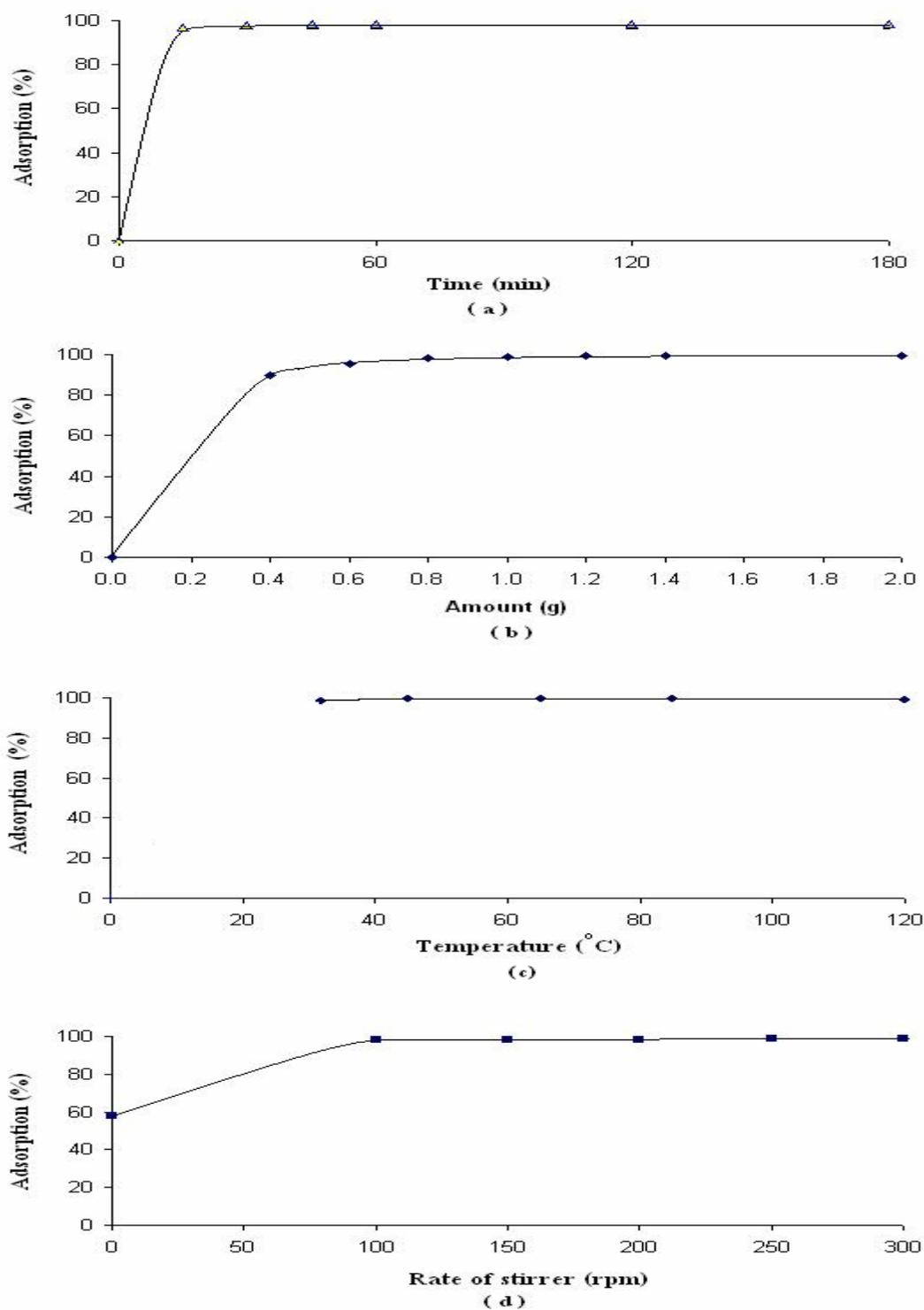
**Figure 30** The effect of stirring time (a), amount of bentonite 200 (b), temperature (c) and stirring rate (d) on one-time adsorption of phorbol esters in *Jatropha* seed oil.
