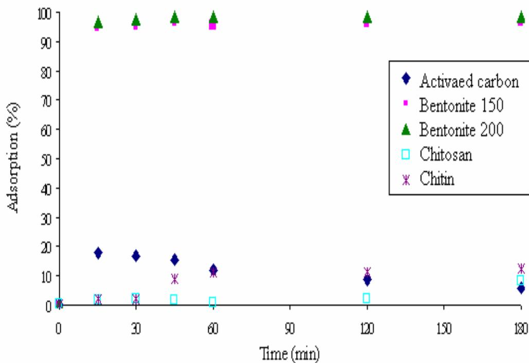
**Figure 29** Phorbol esters adsorption capability in *Jatropha* seed oil by 5 adsorbents.
