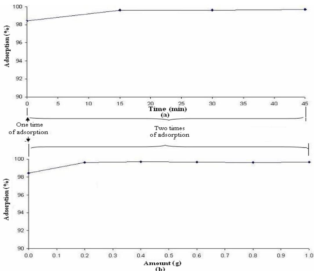
**Figure 31** The effect of stirring rate (a) and bentonite 200 amount (b) on the two-time adsorption capability of phorbol esters.
