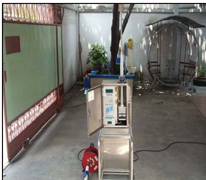
TSP High Volume Sampler
