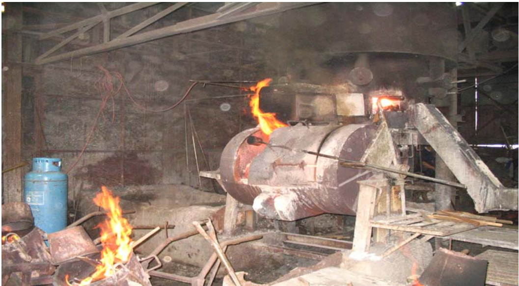
Figure 7 Cupola in small foundry factory in Bangkok area
