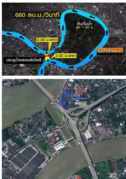
Figure 12: Lad Po man-made canal, a diversion channel for water management under Rama IX King's project (Author)
