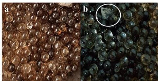
Figure 5. Photographs of deposition of heavy oil on packing at 80 °C (a) and 100 °C of reboiler temperature (b)
