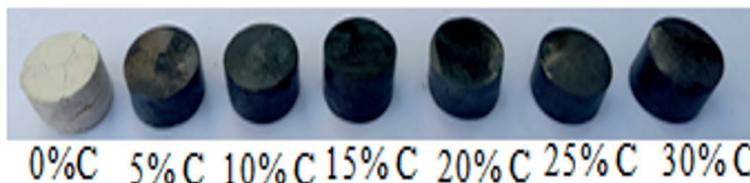
**Figure 1.** Photograph of carbon-ceramic composite electrode prepared from different carbon content
