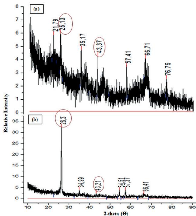
**Figure 5.** XRD pattern of carbon-ceramic composite electrode, (a) XRD pattern of electrode without carbon addition and (b) XRD pattern of electrode with 30 % wt. carbon content
