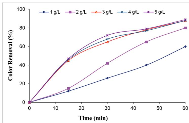
Figure 7. The influence of table salt concentration on color removal efficiency
