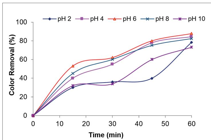
**Figure 6.** The influence of initial pH on color removal efficiency
