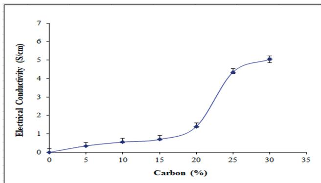
**Figure 3.** Electrically conductive carbon-ceramic composite electrodes with different carbon content
