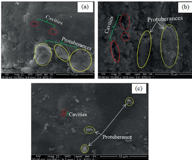
**Figure 4.** SEM micrographs of carbon-ceramic composite electrode after sintered at 900°C, (a) surface morphology of electrode without carbon addition, (b) surface morphology of electrode with 5 wt. % of carbon content and (c) surface morphology of electrode with 30 wt. % of carbon content.
