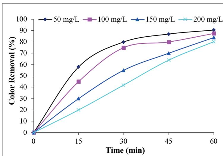
Figure 8. The influence of initial dye concentration on color removal efficiency
