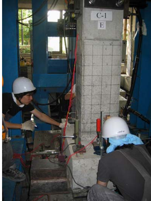
Figure 65 Specimen C1 test setup
