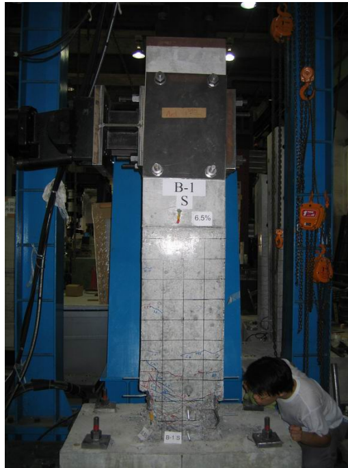
Figure 49 Specimen B1 test setup at failure
