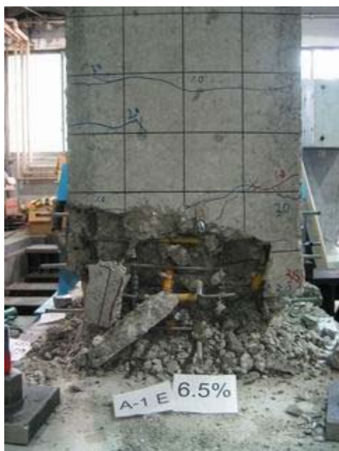
a.) Perpendicular side with lateral force
