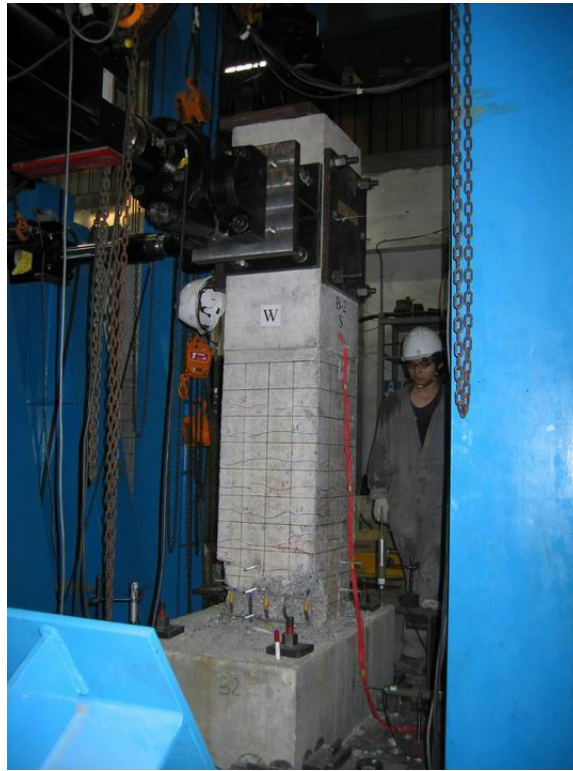
Figure 60 Specimen B2 test setup at the end of test
