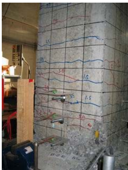
a.) Perpendicular side with lateral force
