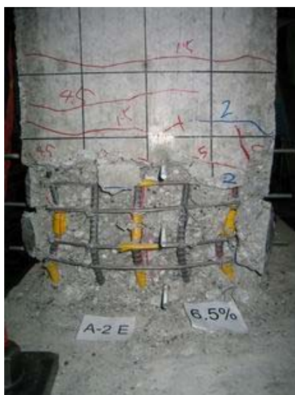
a.) Perpendicular side with lateral force
