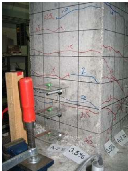
a.) Perpendicular side with lateral force
