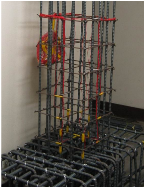
a.) Strain gauging of reinforcement
