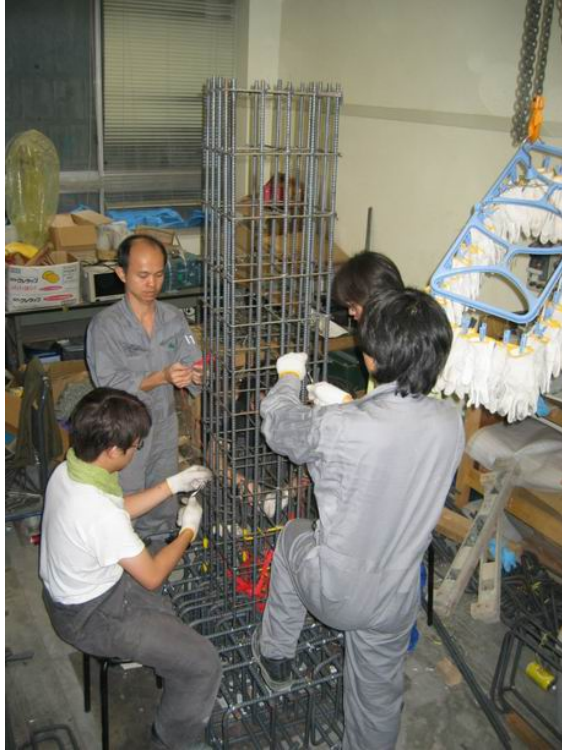
Appendix Figure 1 Constructing reinforcement case of test specimens
