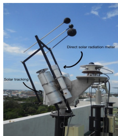
Figure 2 Direct solar radiation meter.
