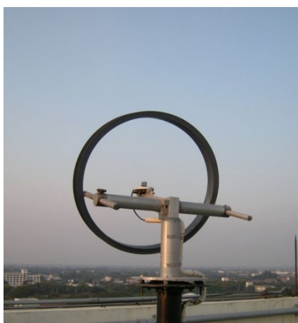
Figure 1 Diffuse solar radiation meter.
