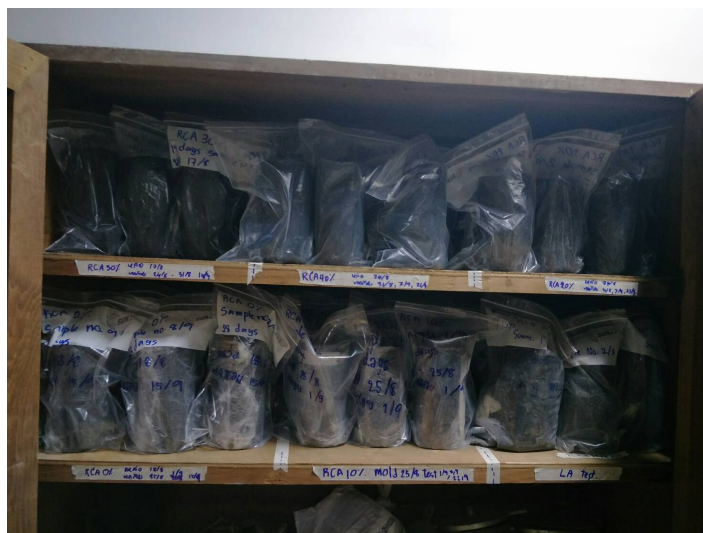
Figure 6 Curing of specimens at 7 and 14 days.
