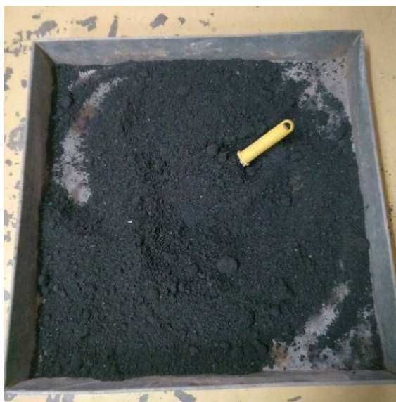
Figure 4 Low-quality crushed rocks mixed with sugar cane ash and cement becoming compactable clod-like materials.
