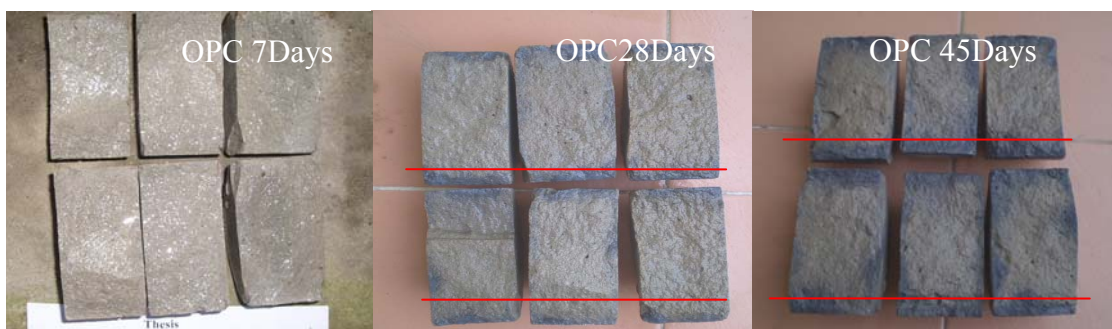
Figure 32 Chloride penetration depths of OPC mortar
