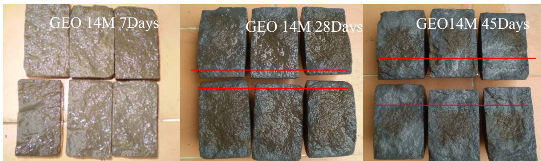
Figure 31 Chloride penetration depths of geopolymer mortar 14M
