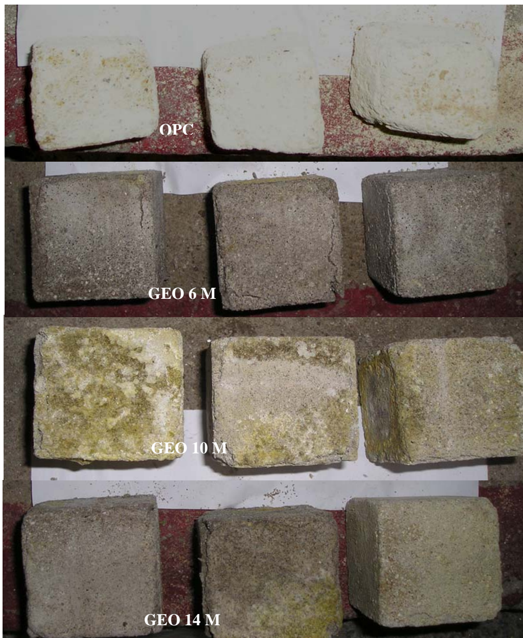
Figure 4 Geopolymer mortar and OPC mortar immersed in sulfuric acid 5% after 120 days
