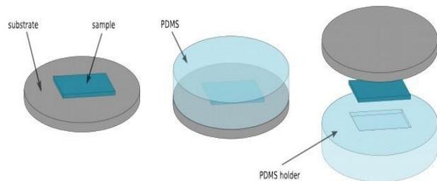
Figure 2. Schematics shows the main steps for the fabrication of the polymer mold
