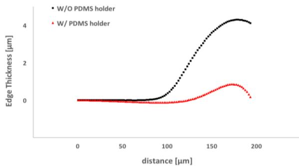
Figure 8. Profilometer measurements of the photoresist film on a square silicon sample spin-coated at 4,000 rpm with and without the PDMS holder
