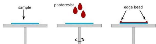
Figure 1. Edge beads formation during spin-coating
