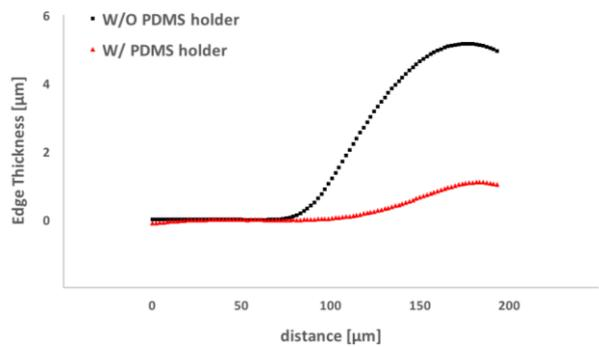
Figure 7. Profilometer measurements of the photoresist film on a square silicon sample spin-coated at 3,000 rpm with and without the PDMS holder
