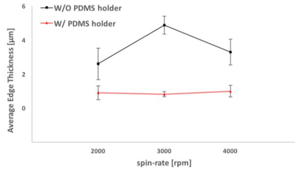
Figure 6. Average edge thickness [ $\mu\text{m}$ ] of the resist film at different spin-rate, when the process is performed with and without the PDMS holder
