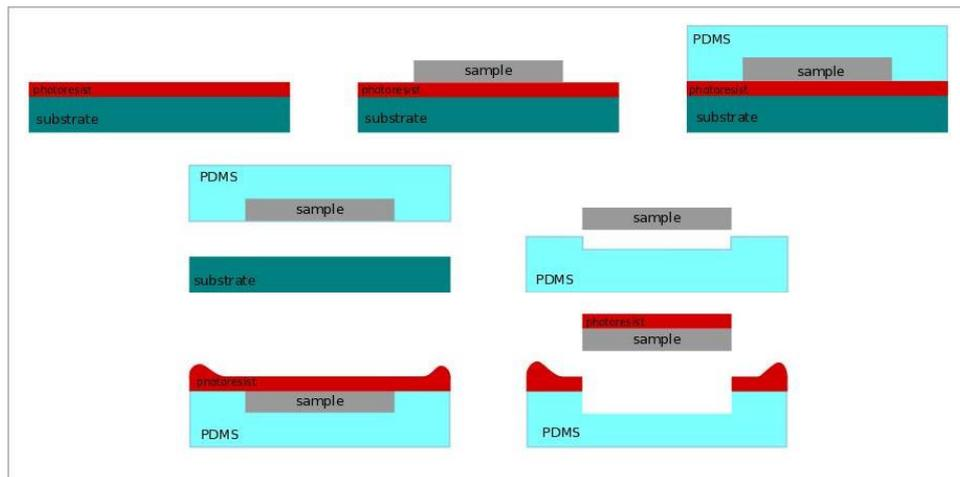
Figure 3. Flow chart of the process for the fabrication of the polymer mold
