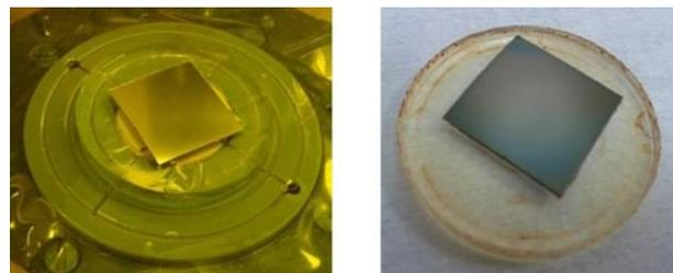
Figure 4. Silicon sample on the PDMS holder before and after the spin coating process
