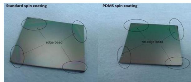
Figure 5. Film of photoresist on a silicon sample after the standard spin coating process (left) and a spin coating process performed with a PDMS holder (right)
