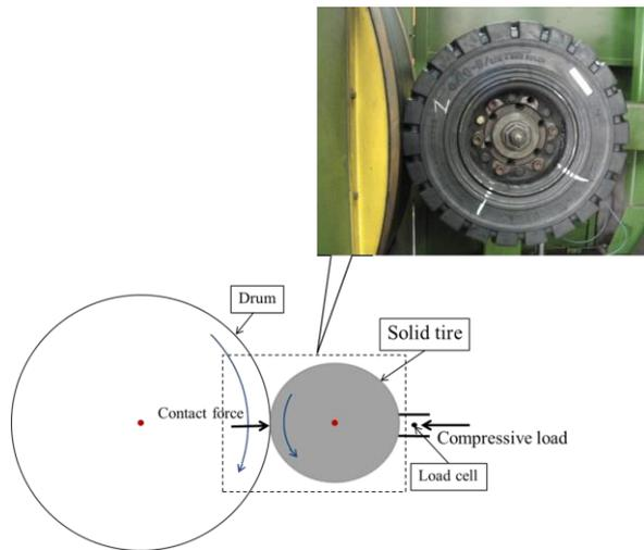
Figure 3. The drum testing of a solid tire
