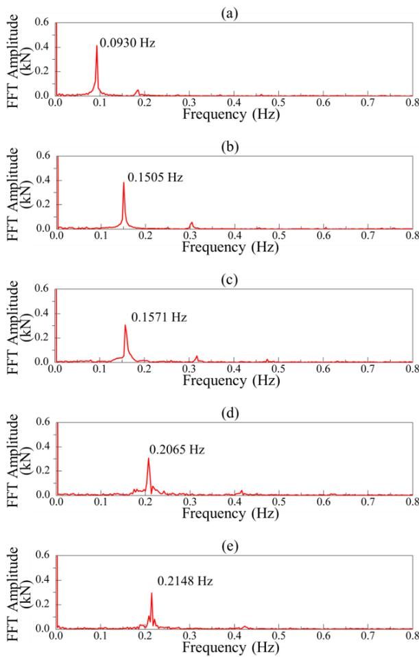
Figure 9. The vibration frequency of contact force signal at the rolling speed of: (a) 10, (b) 20, (c) 30, (d) 40 and (e) 50 km/h at 600 kg compression load
