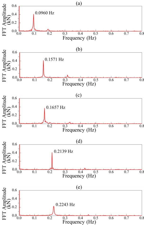
Figure 7. The vibration frequency of contact force signal at the rolling speed of: (a) 10, (b) 20, (c) 30, (d) 40 and (e) 50 km/h at 500 kg compression load
