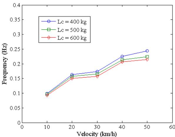
Figure 10. Frequency vs. rolling speed of solid tire at the compression loads of 400, 500 and 600 kg
