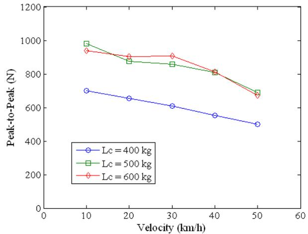
Figure 11. The peak-to-peak contact force vs. rolling speed of solid tire at the compression loads of 400, 500 and 600 kg
