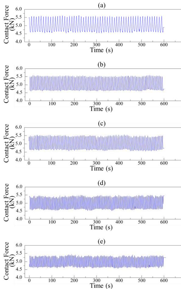
Figure 6. The contact force of solid tire at the rolling speed of: (a) 10, (b) 20, (c) 30, (d) 40 and (e) 50 km/h at 500 kg compression load
