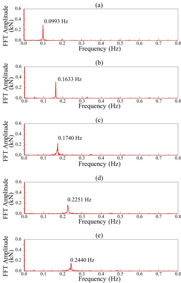
Figure 5. The vibration frequency of contact force signal at the rolling speed of: (a) 10, (b) 20, (c) 30, (d) 40 and (e) 50 km/h at 400 kg compression load
