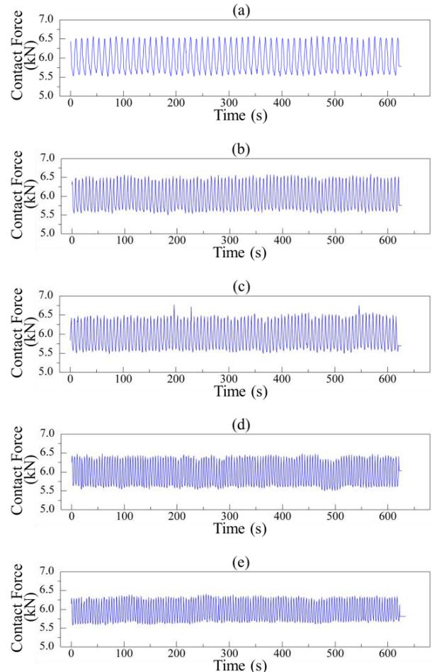
Figure 8. The contact force of solid tire at the rolling speed of: (a) 10, (b) 20, (c) 30, (d) 40 and (e) 50 km/h at 600 kg compression load.
