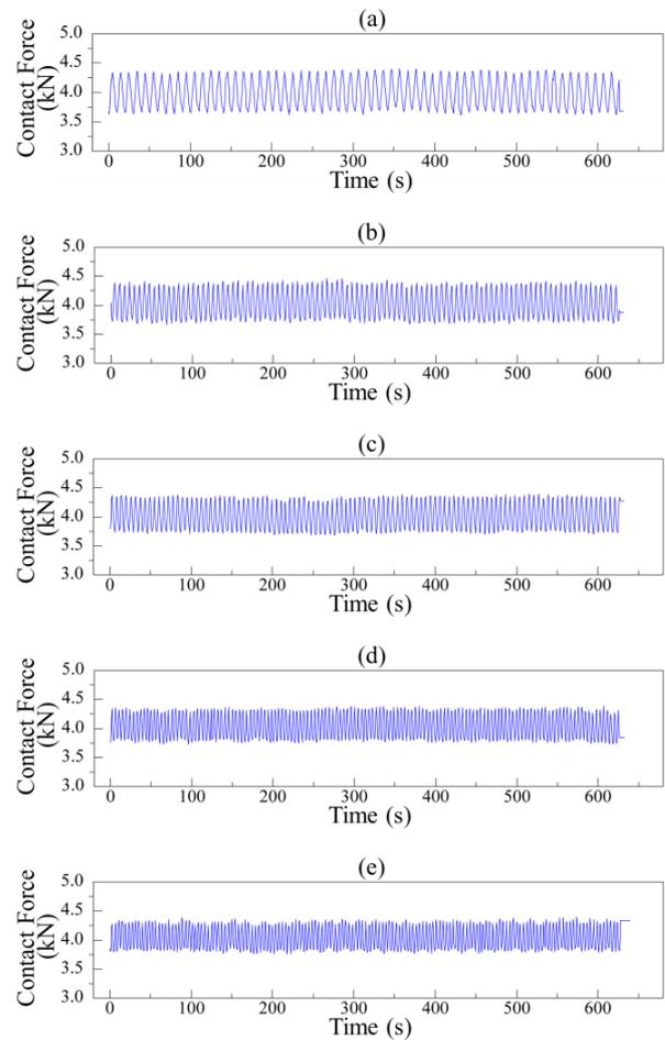
Figure 4. The contact force of solid tire at the rolling speed of: (a) 10, (b) 20, (c) 30, (d) 40 and (e) 50 km/h at 400 kg compression load
