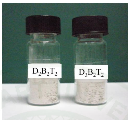
Figure 59 Examples of white powder PLA obtained with 10 kg of LA by DMPC using catalyst B.
