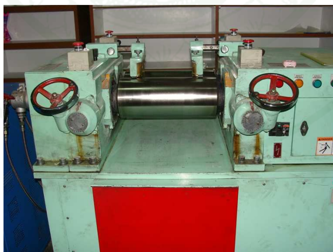
Figure 28 Two roll mill (Model YFCR 6, Chor. Sri-Anan Co. Ltd., Thailand).
