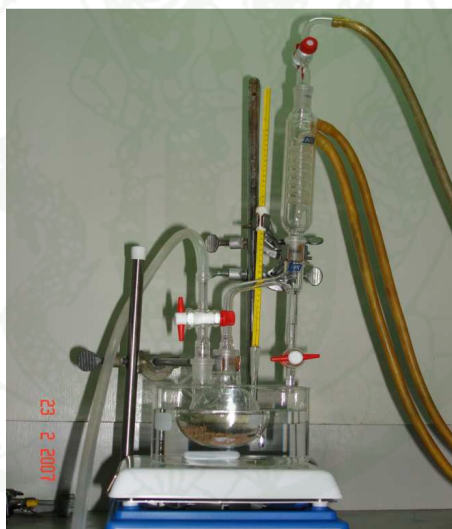
Figure 31 System setup showing the Dean-Stark trap for carrying the SP with 100 g of LA.
