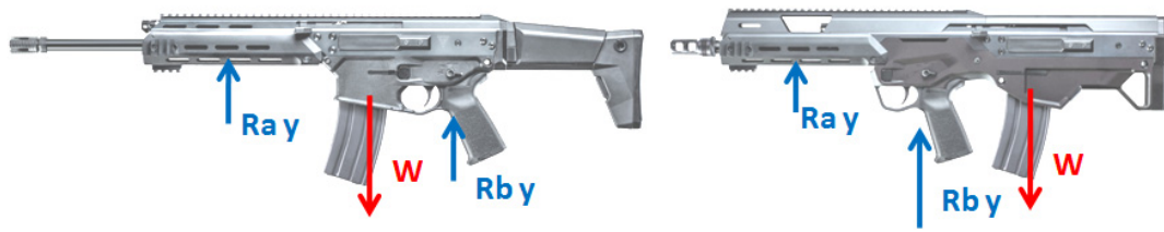
Figure 5 Reaction at hand guard and handgrip in Classic and Bullpup type
