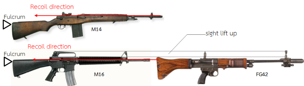
Figure 2 Moment reduction design in M16
