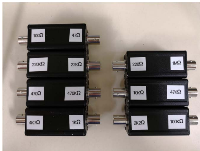
Figure 4. A set of resistor boxes with various resistors inside. It is important to cover the range of the resistance from 50\ \Omega to 1\ \text{M}\Omega .
