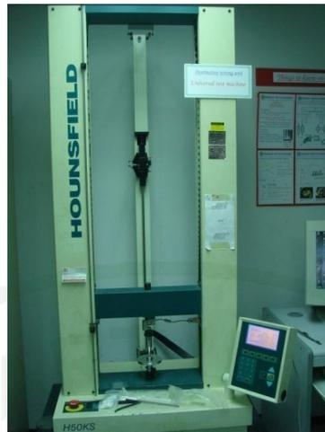
**Figure 21** Universal testing machine.
