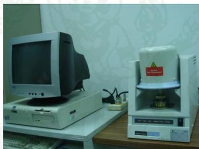
**Figure 17** Differential thermal analyzer.
