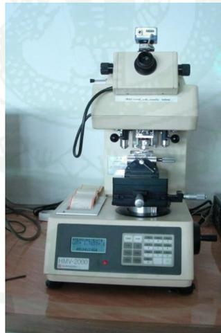
**Figure 22** Vickers microhardness tester.
