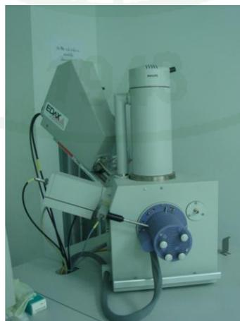
**Figure 25** Scanning electron microscope.
