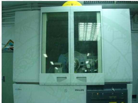
**Figure 26** X-rays diffractometer.
