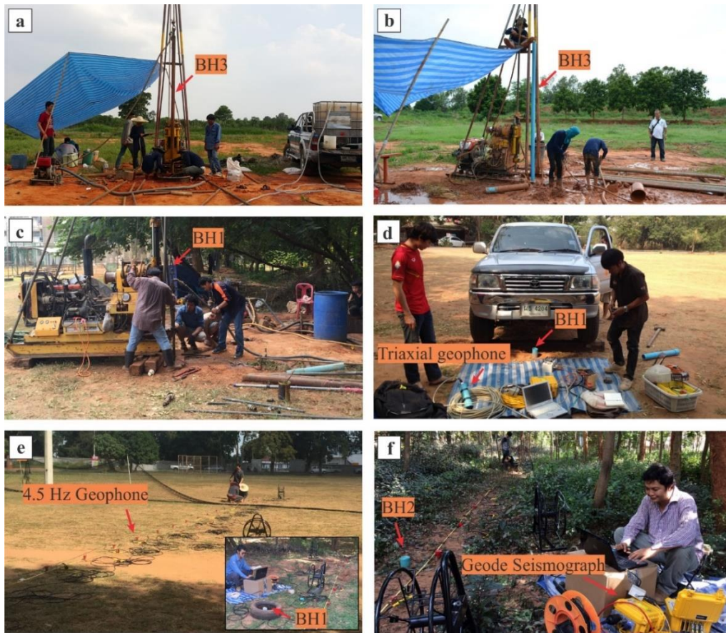
Figure 4. Operation of downhole and MASW techniques, (a-c) borehole drilling and set up, (d) downhole testing, (e) active MASW data acquisition at BH1, and (f) passive MASW data acquisition at BH2
