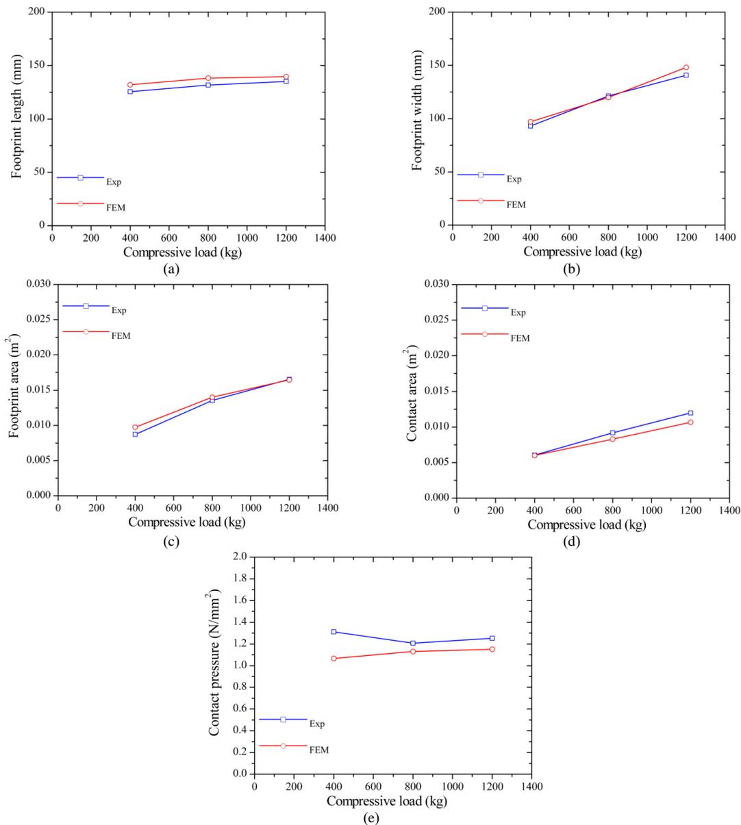
Figure 10. The footprint of compressed solid tyre: (a) footprint length, (b) footprint width, (c) footprint area, (d) contact area, and (e) contact pressure under various compressive loads
