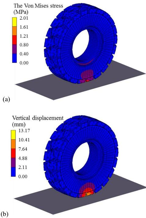
Figure 6. The simulation results, (a) Von Mises stress, and (b) vertical displacement, in compression test of solid tire at 12.0 kN load
