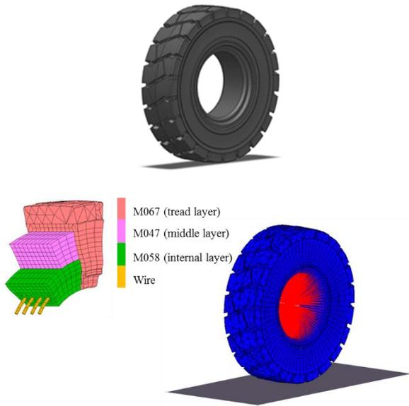
Figure 4. The KOMACHI solid tire model (a) 3-D model, and (b) finite element model
