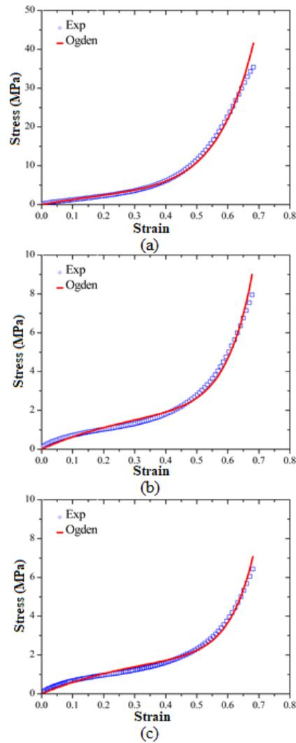
Figure 5. The curve fitting results using the Ogden model for rubber compounds (a) M058, (b) M047, and (c) M067
