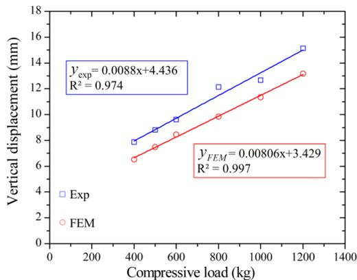
Figure 7. The vertical displacement vs. compression load in compression test of solid tires
