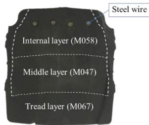
Figure 1. The cross-section of solid tire
