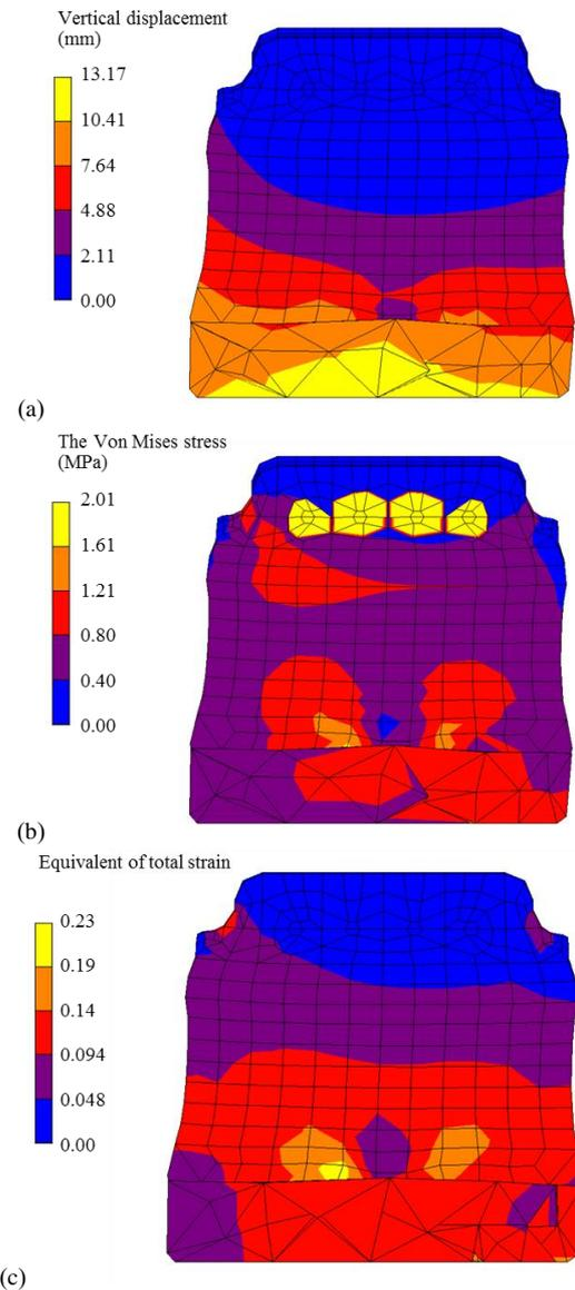
Figure 8. The simulation results, (a) vertical displacement, (b) stress, and (c) strain in compression test of a solid tire at 12.0 kN load
