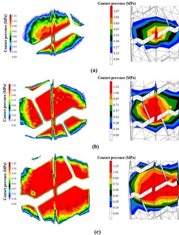
Figure 9. The footprint result comparison of experimental (left) and FEM simulation (right) in compression test of solid tire at (a) 4.0, (b) 8.0, and (c) 12.0 kN
