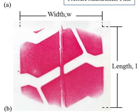
Figure 3. The tire stiffness testing: (a) compression test of a solid tire using the stiffness tester (EKTRON, model PL-2003) and (b) footprint on pressure measurement film
