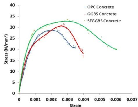
Figure 2. Stress-strain curves.
