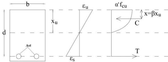
Figure 3. Stress block parameters.
