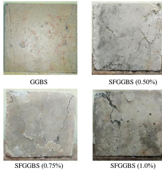
Figure 1. Failure patterns for GGBS and SFGGBS concrete.
