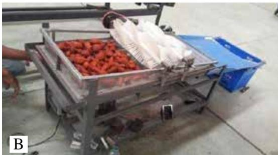
**Figure 3** (A) Thorns removing by conventional method (B) Testing brush rollers speed and tilt tray angle of experimental prototype of thorns removing machine
