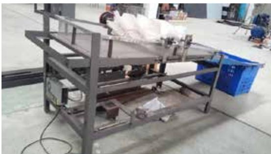
**Figure 2** The experimental prototype of salacca thorns removing machine
