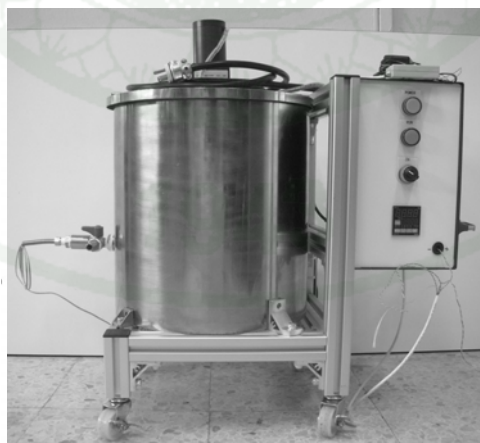
Figure 9 The hot-bath of the non-minimum phase pilot process
