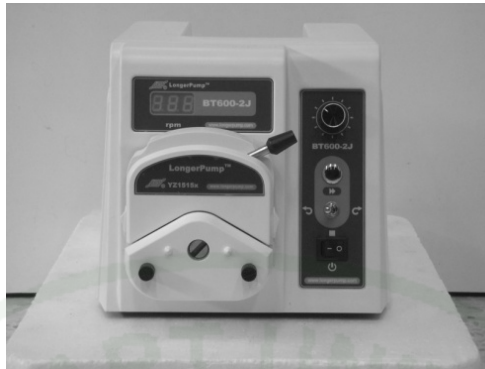
Figure 11 The peristaltic pump used in the non-minimum phase pilot process
