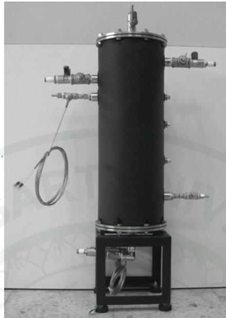
Figure 8 The exchanger unit of the non-minimum phase pilot process
