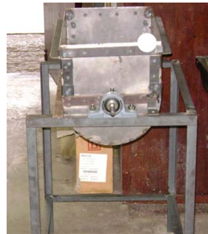
Figure 24 Development of corn roaster model.
