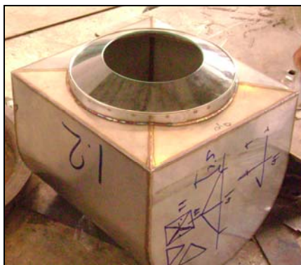
Figure 7 Fabrication of chamber and lid.
