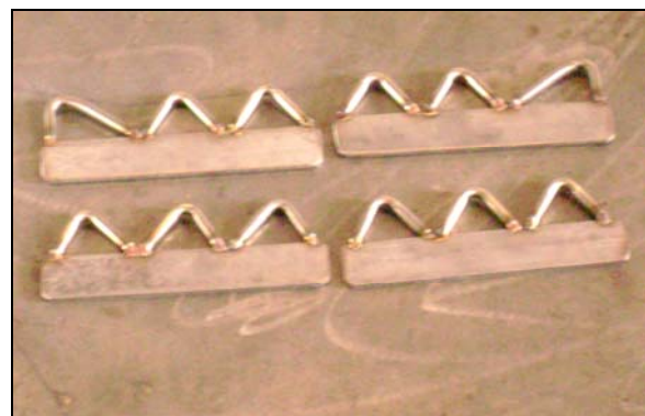
Figure 8 Fabrication of agitation fins.
