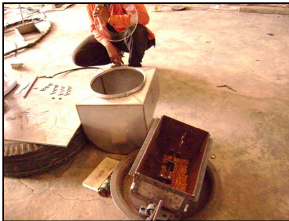
Figure 23 The roaster chamber with lid being fabricated in the workshop.
