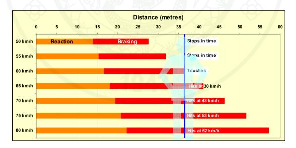
Figure 4 Stopping distance at different speeds
