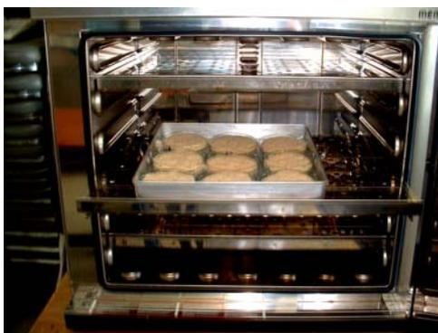
Figure 26 Presented the method of control moisture content in wood powder by drying in oven at 50°C.
