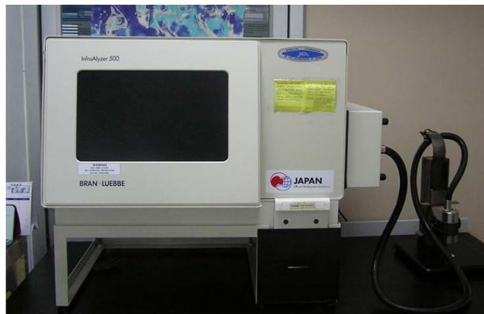
Figure 19 Near Infrared Spectroscopic Instrument of InfraAlyzer 500 (Bran+Luebbe)
