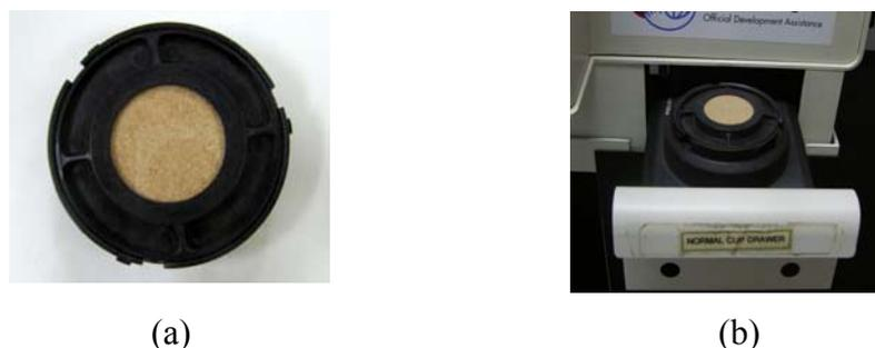
**Figure 27** Closed cup packing (a) and sample holder using in the near infrared spectrometer Infra-Alyzer 500 (Bran+Luebbe) (b).
