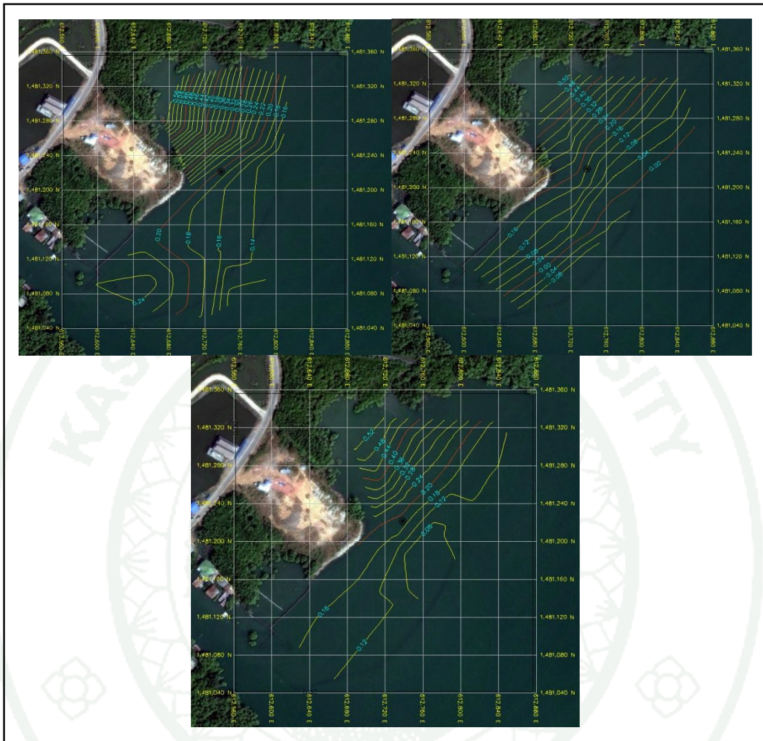
Figure 38 Contours of measured sediments at non protected area during each period of prevailing wind direction.
