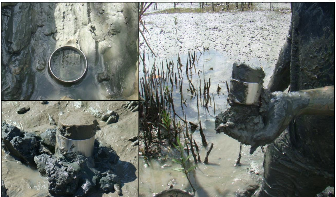
Figure 22 Soil sampling by soil cores for analyses in laboratory.
