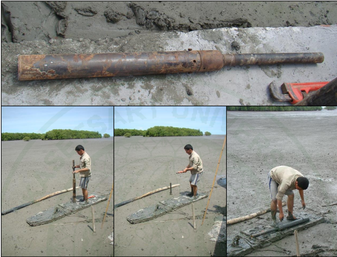
Figure 23 Soil sampling by thin wall tube for analyses in laboratory.
