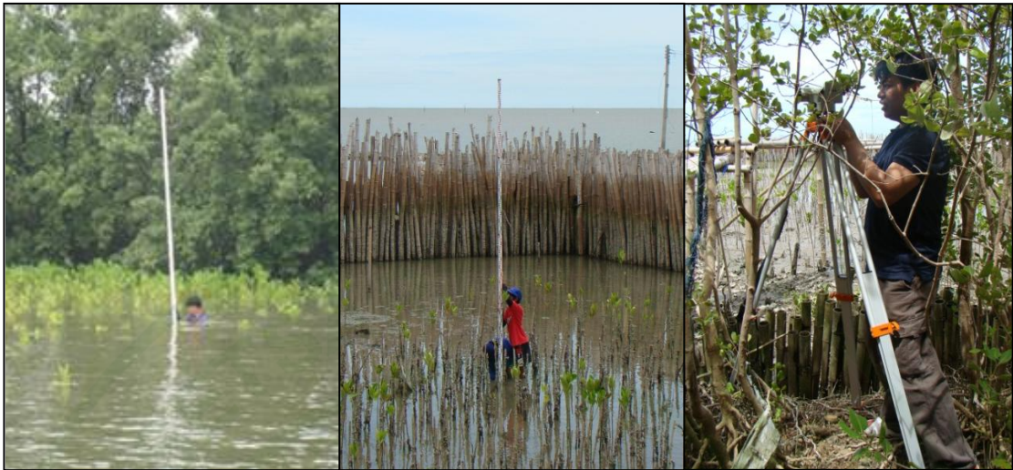
Figure 21 Sediment erosion and deposition measuring by leveling telescope.
