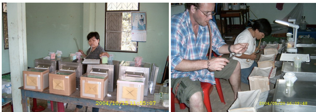
Figure 17: Exito-repellency test chamber were designed to compare two field populations of the wild caught species in contact and non-contact exposures using insecticide treated papers.
