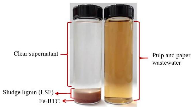
**Figure 1.** Separation of wastewater into layers: Fe-BTC powder at the bottom, LSF in the middle, and clear supernatant at the top
