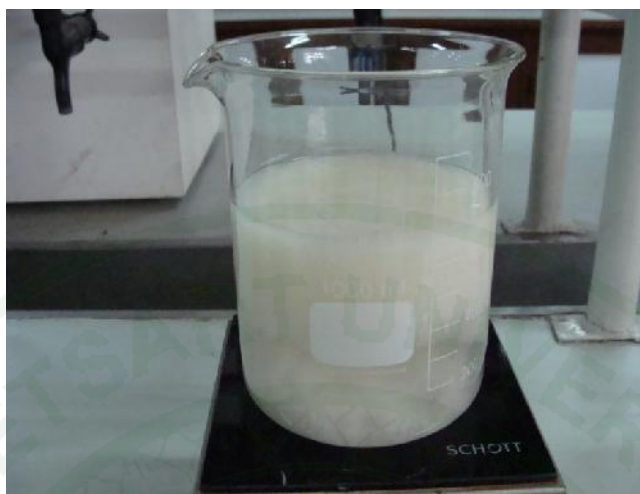
Figure 23 Delignification of rice straw with \text{H}_2\text{O}_2 .
