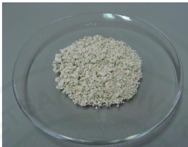
Figure 33 Dried pure \alpha -cellulose obtained from rice straw.
