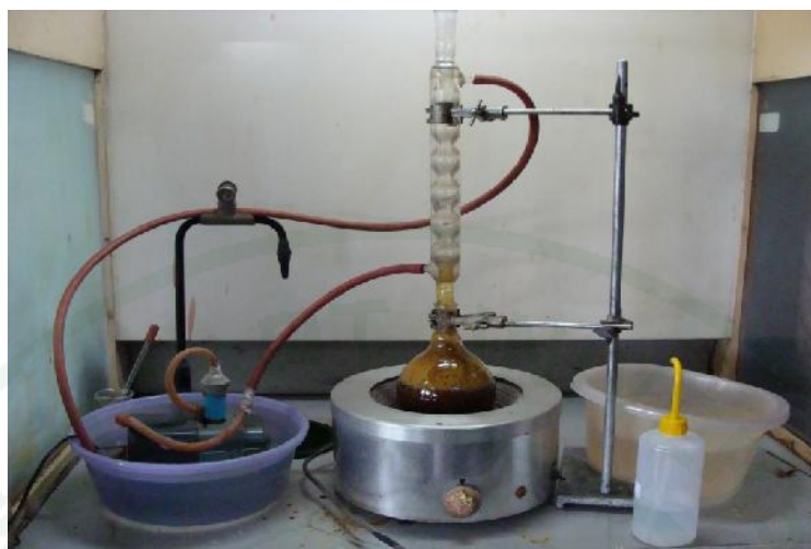
Figure 20 Alkali treatment of pretreatment rice straw residues.
