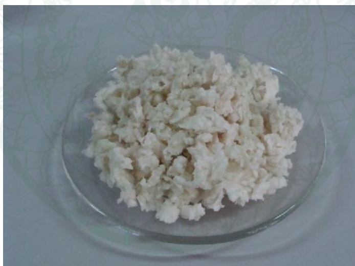
Figure 30 Rice straw residues obtained from bleaching with 1% NaOCl.
