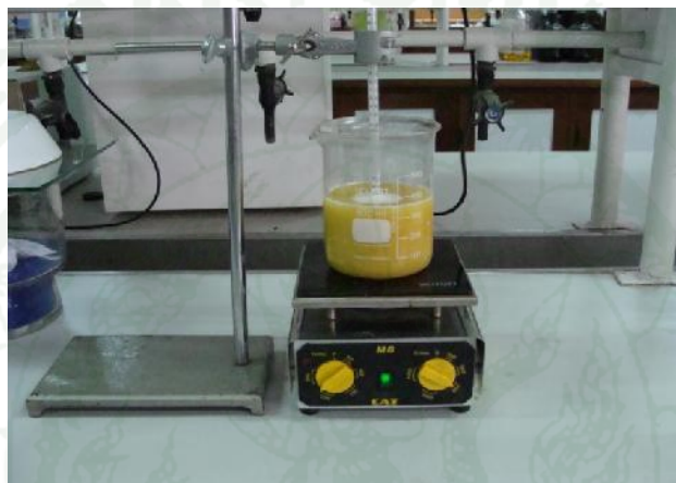
Figure 22 Alkali extraction of rice straw.
