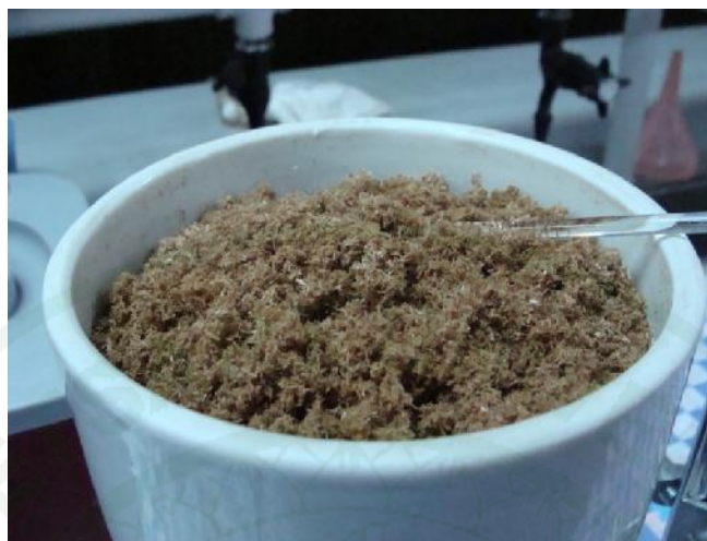
Figure 28 Rice straw residues obtained from pretreatment.
