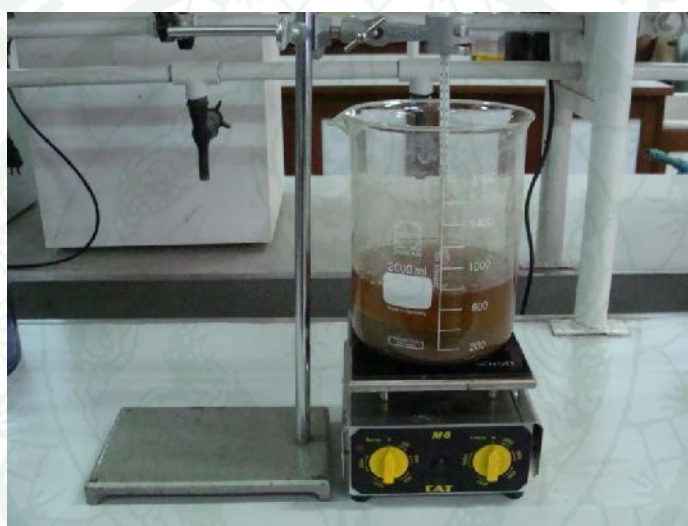
Figure 19 Pretreatment of lignocellulosic rice straw fibers.
