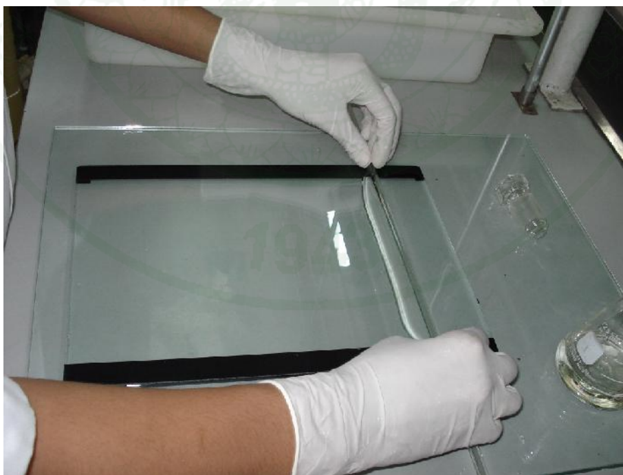
Figure 24 Casting of PLA/rice straw biocomposites on a glass plate.
