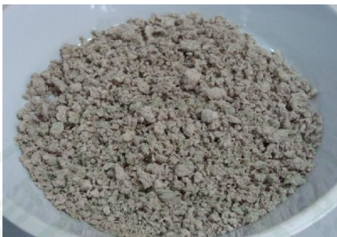
Figure 29 Rice straw residues obtained from alkali treatment.
