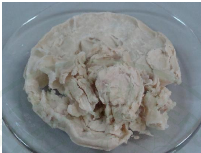
Figure 31 Rice straw residues obtained from alkali extraction.
