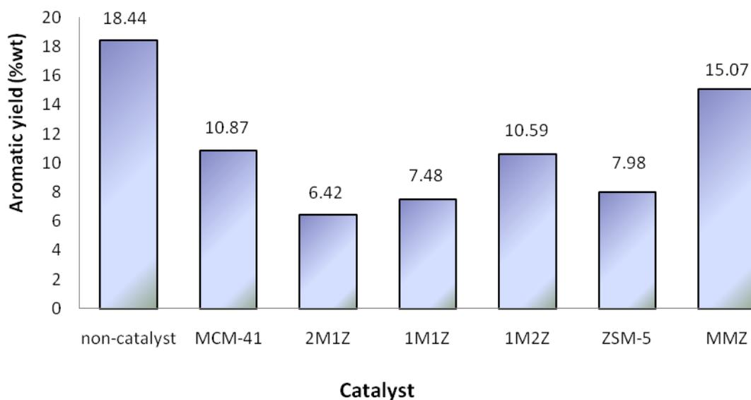
**Figure 11** Aromatic fraction in the organic phase of bio-oil (%wt) from non-catalyst reaction and bio-oil upgraded by MCM-41, HZSM-5, MMZ and the blend of MCM-41 and HZSM-5 with the ratios of 1:1 (1M1Z), 1:2(1M2Z) and 2:1(2M1Z)
