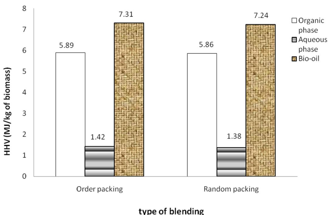
**Figure 20** Total energy output of bio-oils upgraded by different sequences of catalysts packing; order packing and random packing
