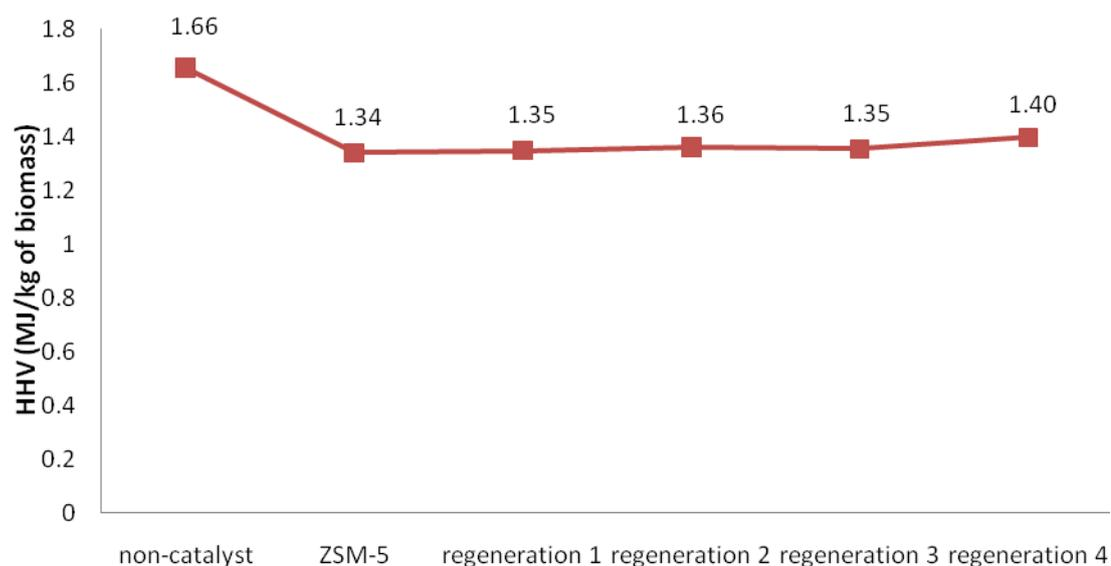
**Figure 46** Total energy output (MJ/kg of biomass) of aqueous phase of bio-oils upgraded by fresh and regenerated HZSM-5 at 673K
