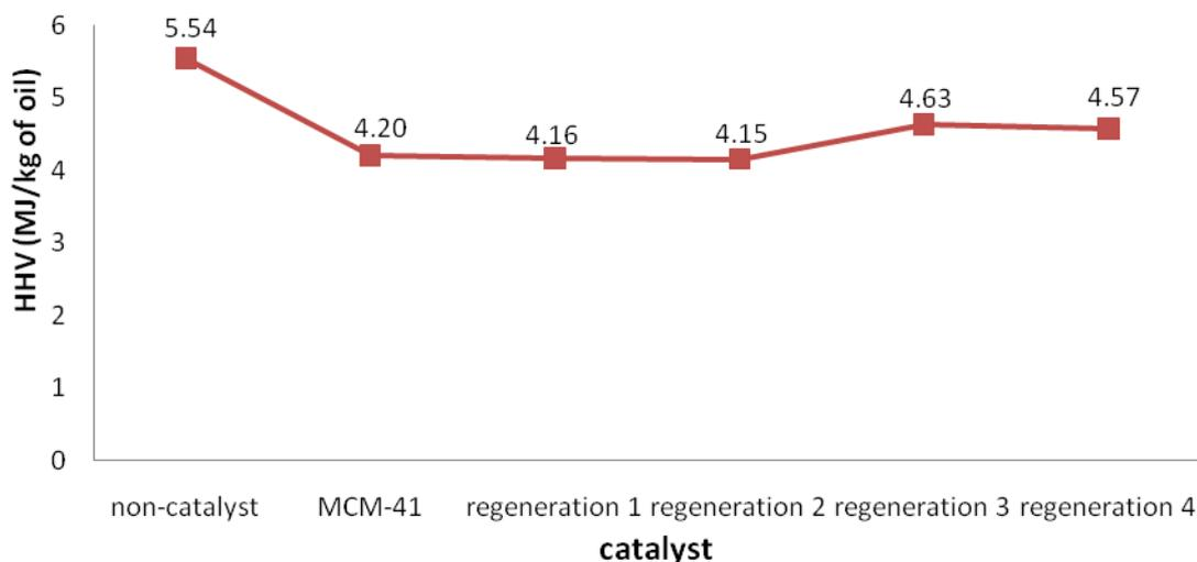
**Figure 31** High heating values (HHV) (MJ/kg) of aqueous phase of bio-oils upgraded by fresh and regenerated MCM-41 at 673K
