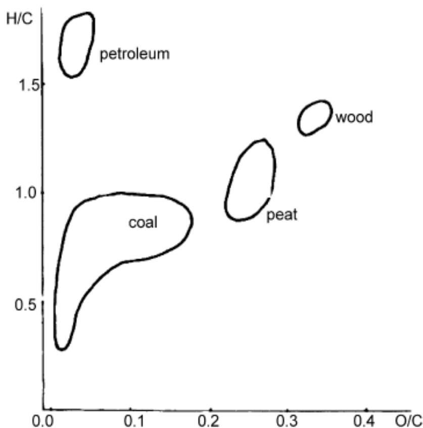
**Figure 1** The elemental content of coal, petroleum and wood
