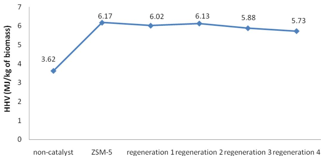
**Figure 45** Total energy output (MJ/kg of biomass) of organic phase of bio-oils upgraded by fresh and regenerated HZSM-5 at 673K
