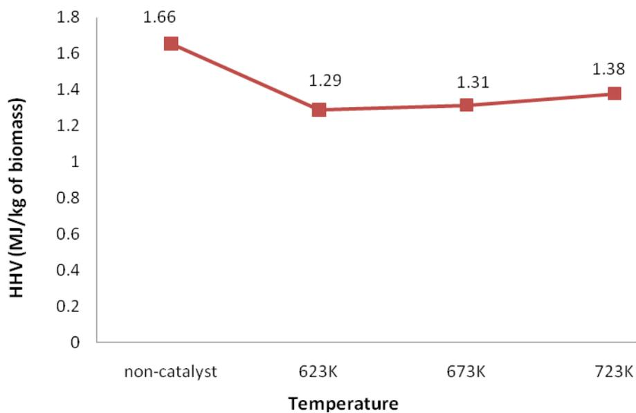
**Figure 28** Total energy output (MJ/kg of biomass) of aqueous phase of bio-oils upgraded at different temperatures; 623, 673 and 723K
