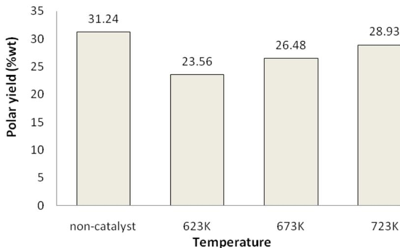
**Figure 25** Polar fractions (%wt) from organic phases of bio-oils upgraded by different temperatures; 623, 673 and 723K
