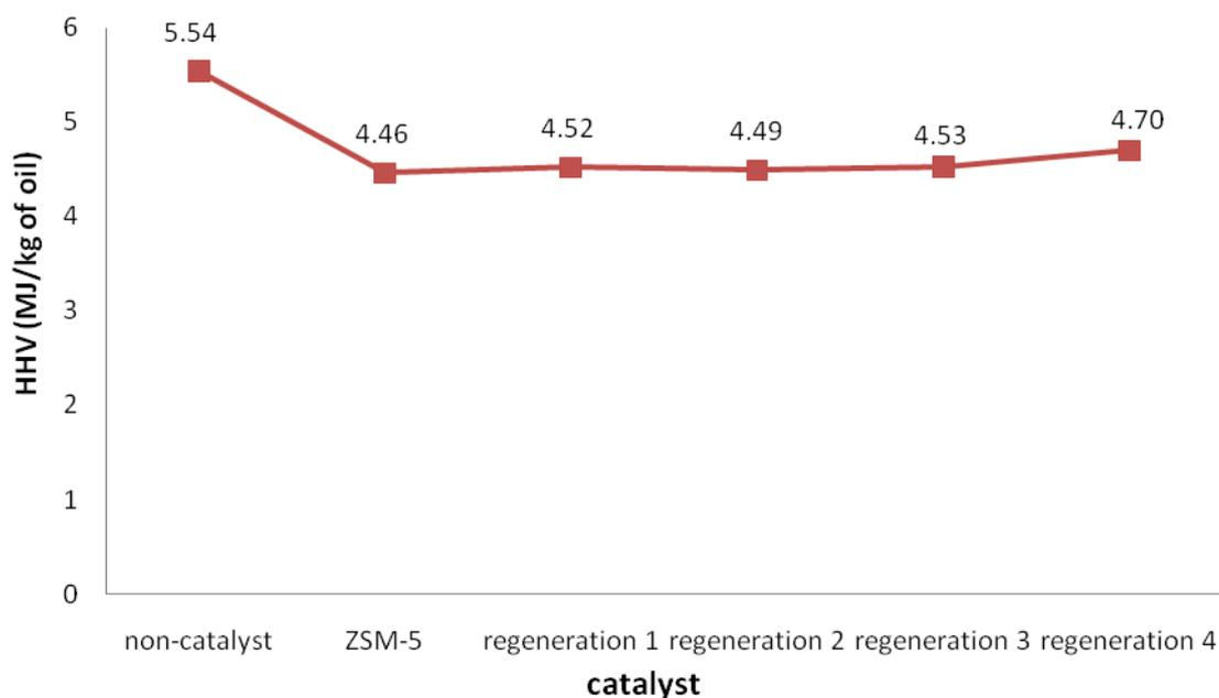
**Figure 40** High heating values (HHV) (MJ/kg) of aqueous phase of bio-oils upgraded by fresh and regenerated HZSM-5 at 673K
