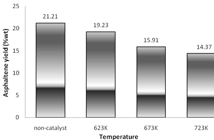
**Figure 26** Asphaltene fractions (%wt) from organic phases of bio-oils upgraded by different temperatures; 623, 673 and 723K
