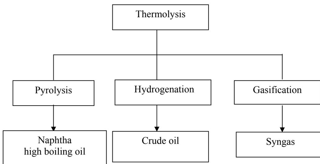
**Figure 2** Overview of the main form of biomass feedstock by thermolysis.
