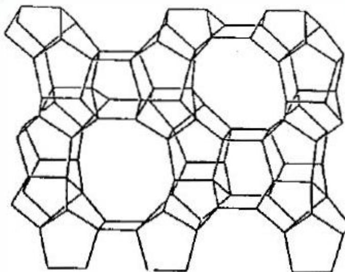
**Figure 6** Structure of HZSM-5
