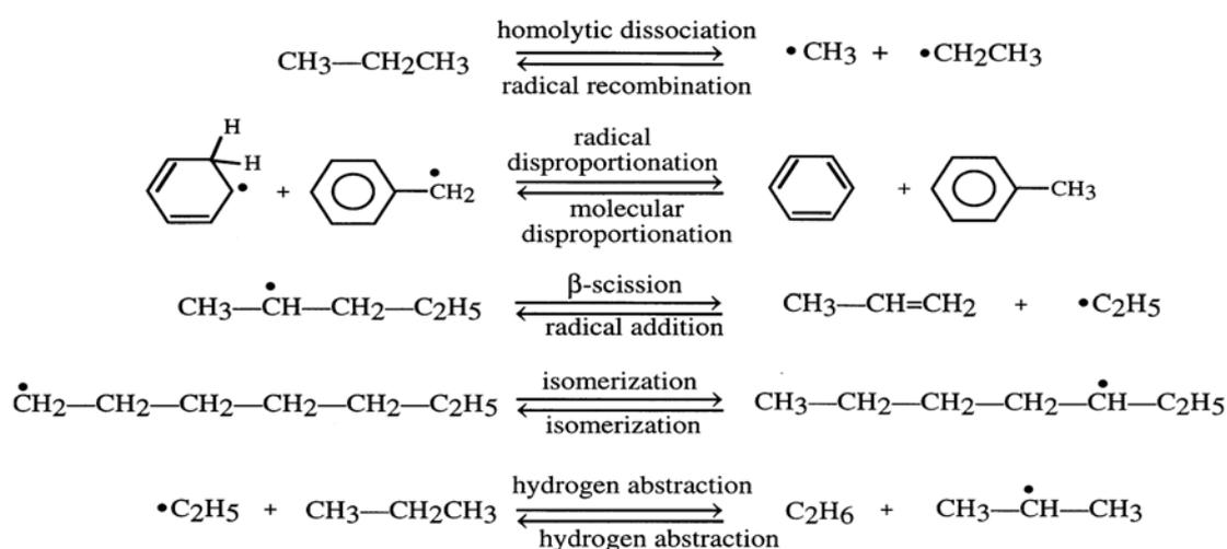
**Figure 3** Main reaction families for hydrocarbon pyrolysis.
