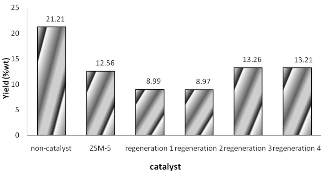
**Figure 44** Asphaltene fractions (%wt) of organic phases of bio-oils upgraded by fresh and regenerated HZSM-5 at 673K
