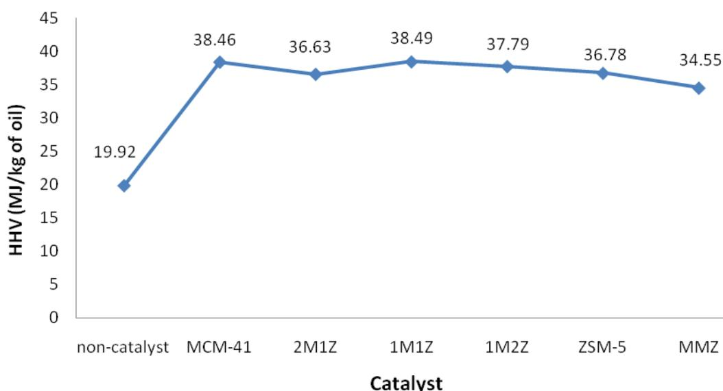
**Figure 8** High heating values (HHV) (MJ/kg) of bio-oil from non-catalyst reaction and bio-oil upgraded by MCM-41, HZSM-5, MMZ and the blend of MCM-41 and HZSM-5 with the ratios of 1:1 (1M1Z), 1:2(1M2Z) and 2:1(2M1Z) for organic phase.
