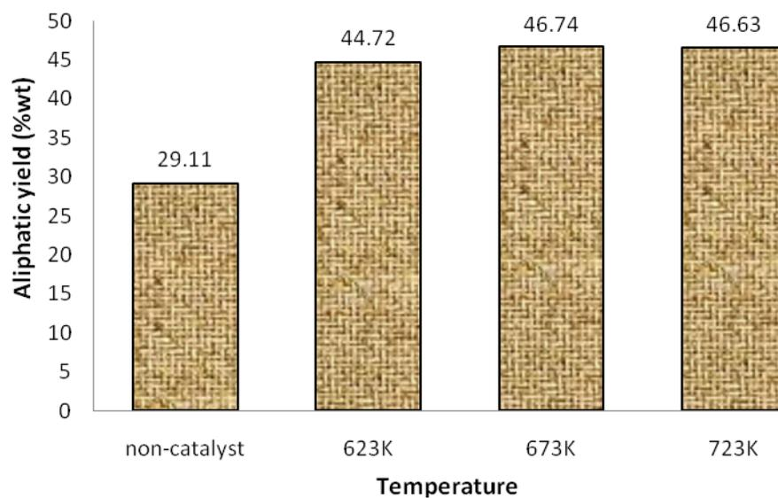
**Figure 23** Aliphatic fractions (%wt) from organic phases of bio-oils upgraded by different temperatures; 623, 673 and 723K
