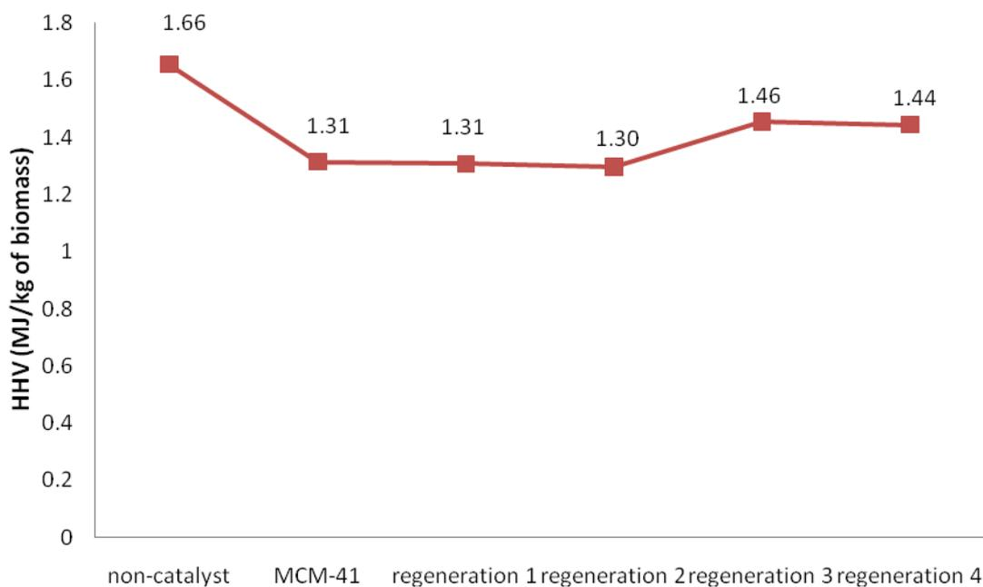
**Figure 37** Total energy output (MJ/kg of biomass) of aqueous phase of bio-oils upgraded by fresh and regenerated MCM-41 at 673K
