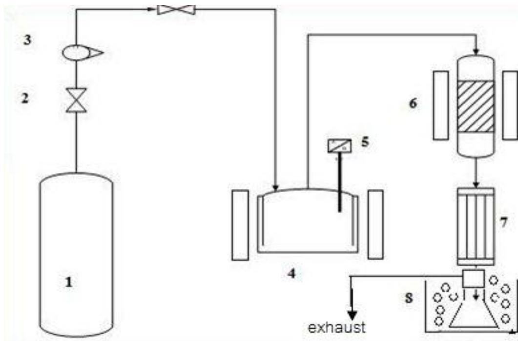
**Figure 7** Schematic diagram of experimental setup for pyrolysis of soybean cake:
