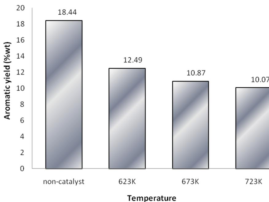
**Figure 24** Aromatic fractions (%wt) from organic phases of bio-oils upgraded by different temperatures; 623, 673 and 723K
