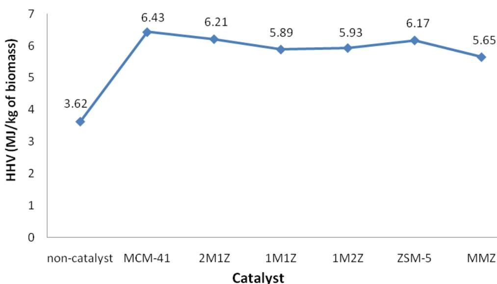
**Figure 14** Total energy output for the organic phase of bio-oil (MJ/kg of biomass) from non-catalyst reaction and bio-oil upgraded by MCM-41, HZSM-5, MMZ and the blend of MCM-41 and HZSM-5 with the ratios of 1:1 (1M1Z), 1:2(1M2Z) and 2:1(2M1Z)
