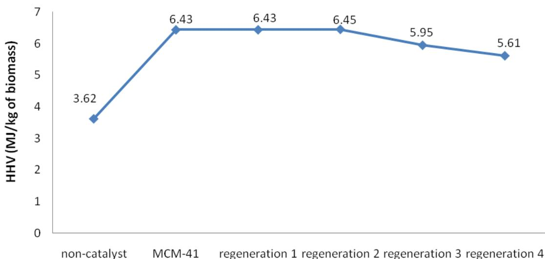
**Figure 36** Total energy output (MJ/kg of biomass) of organic phase of bio-oils upgraded by fresh and regenerated MCM-41 at 673K
