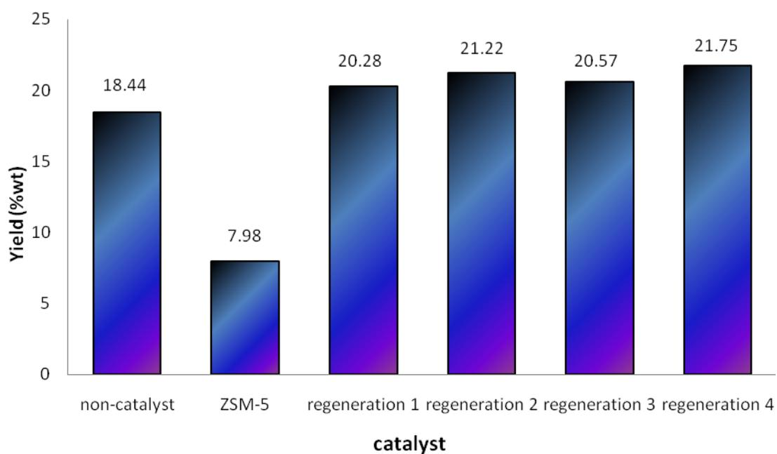
**Figure 42** Aromatic fractions (%wt) of organic phases of bio-oils upgraded by fresh and regenerated HZSM-5 at 673K
