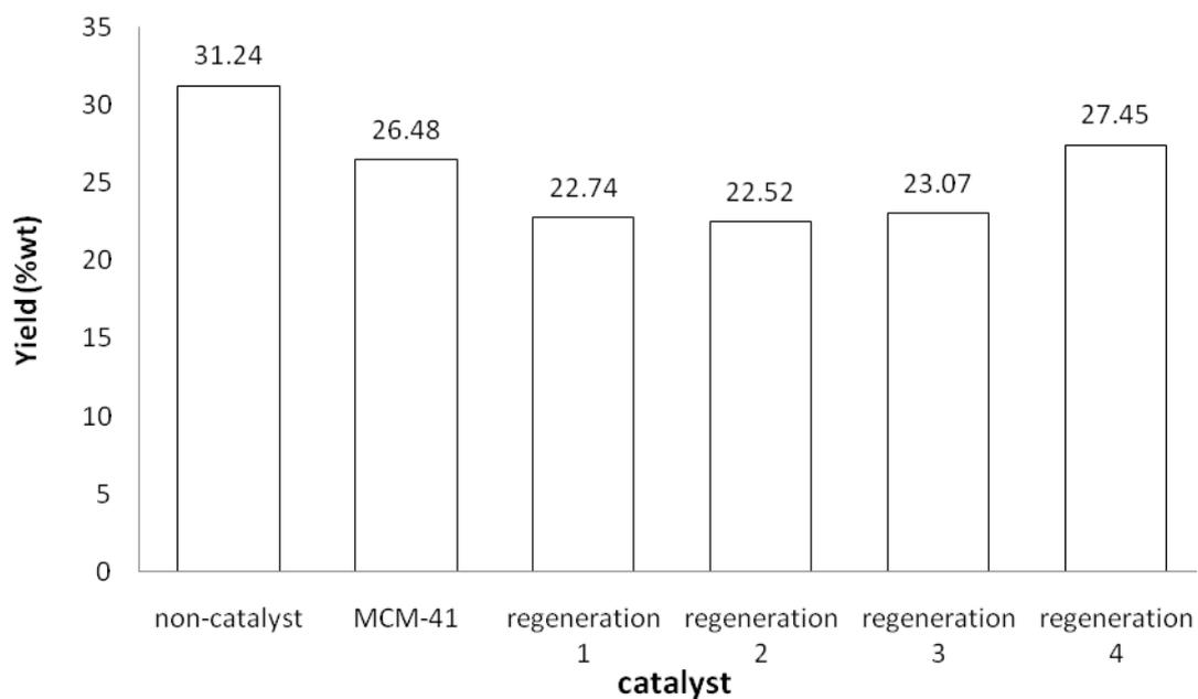
**Figure 34** Polar fraction (%wt) of organic phase of bio-oils upgraded by fresh and regenerated MCM-41 at 673K
