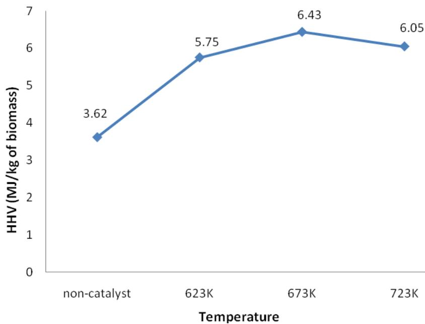
**Figure 27** Total energy output (MJ/kg of biomass) of organic phase of bio-oils upgraded at different temperatures; 623, 673 and 723K
