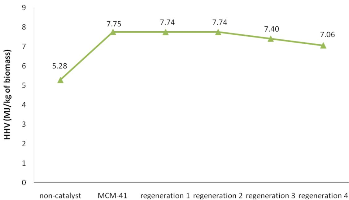
**Figure 38** Total energy output (MJ/kg of biomass) of bio-oils (both organic and aqueous phase) upgraded by fresh and regenerated MCM-41 at 673K
