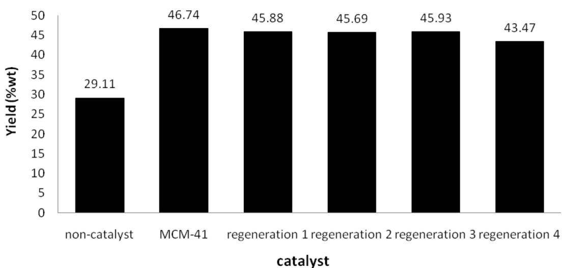
**Figure 32** Aliphatic fraction (%wt) of organic phase of bio-oils upgraded by fresh and regenerated MCM-41 at 673K
