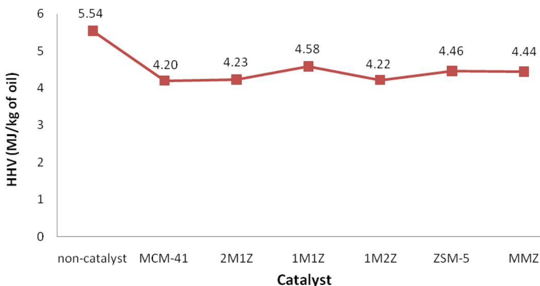
**Figure 9** High heating values (HHV) (MJ/kg) of bio-oil from non-catalyst reaction and bio-oil upgraded by MCM-41, HZSM-5 and the blend of MCM-41 and HZSM-5 with the ratios of 1:1 (1M1Z), 1:2(1M2Z) and 2:1(2M1Z) for aqueous phase.
