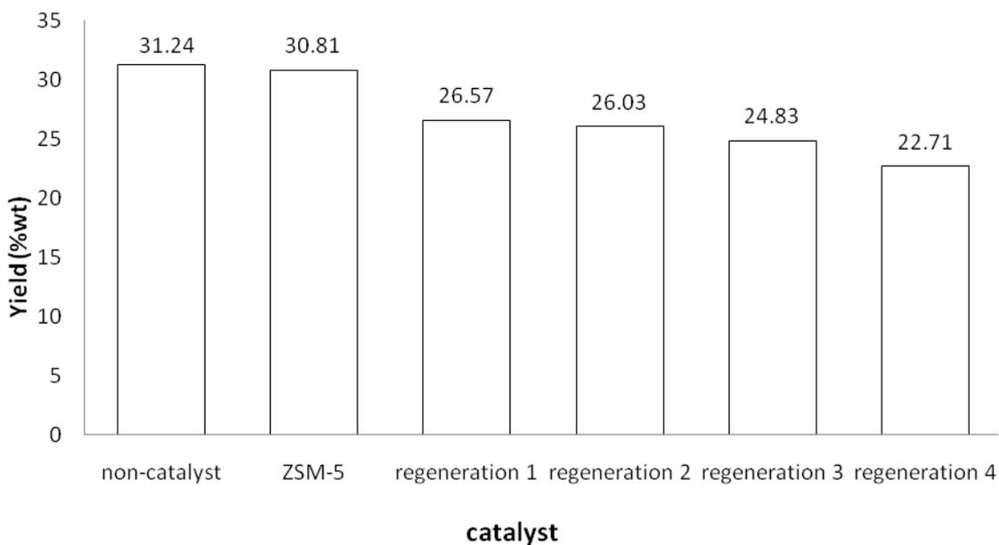
**Figure 43** Polar fractions (%wt) of organic phases of bio-oils upgraded by fresh and regenerated HZSM-5 at 673K
