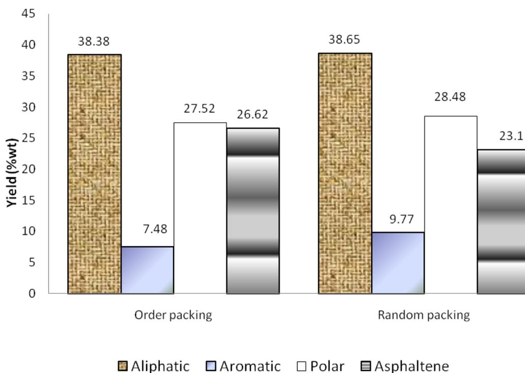
**Figure 19** Chemical class composition from organic phases of bio-oils upgraded by different sequences of catalysts packing; order packing and random packing
