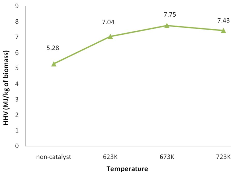
**Figure 29** Total energy output (MJ/kg of biomass of bio-oils (both of organic and aqueous phase) upgraded at different temperatures; 623, 673 and 723K
