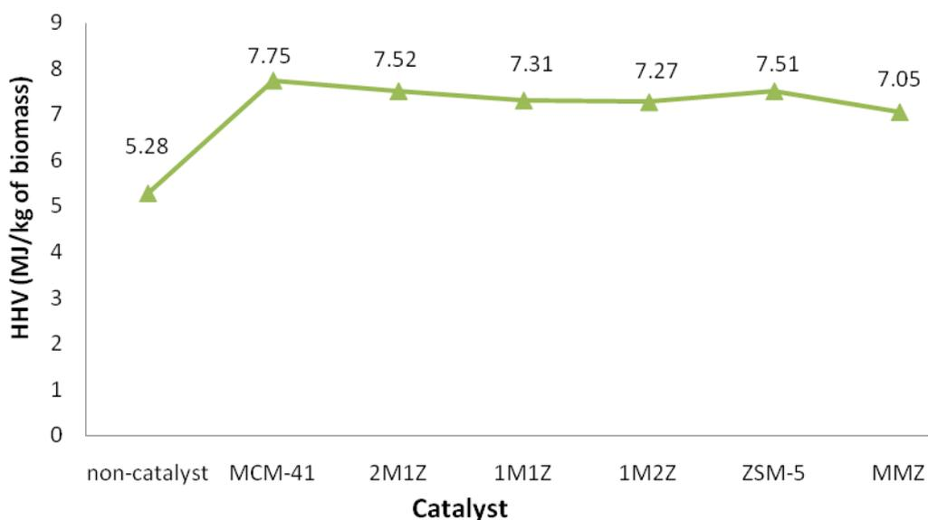
**Figure 16** Total energy output from bio-oils (both of organic and aqueous phases) from non-catalyst reaction and bio-oil upgraded by MCM-41, HZSM-5, MMZ and the blend of MCM-41 and HZSM-5 with the ratios of 1:1 (1M1Z), 1:2(1M2Z) and 2:1(2M1Z)
