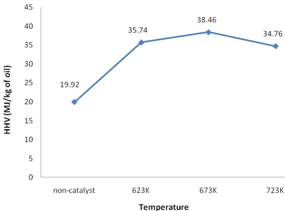
**Figure 21** High heating values (HHV) (MJ/kg) of organic phase of bio-oils upgraded by different temperatures; 623, 673 and 723K
