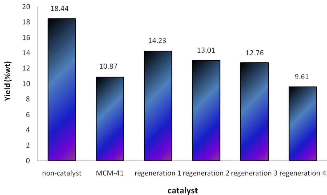
**Figure 33** Aromatic fraction (%wt) of organic phase of bio-oils upgraded by fresh and regenerated MCM-41 at 673K
