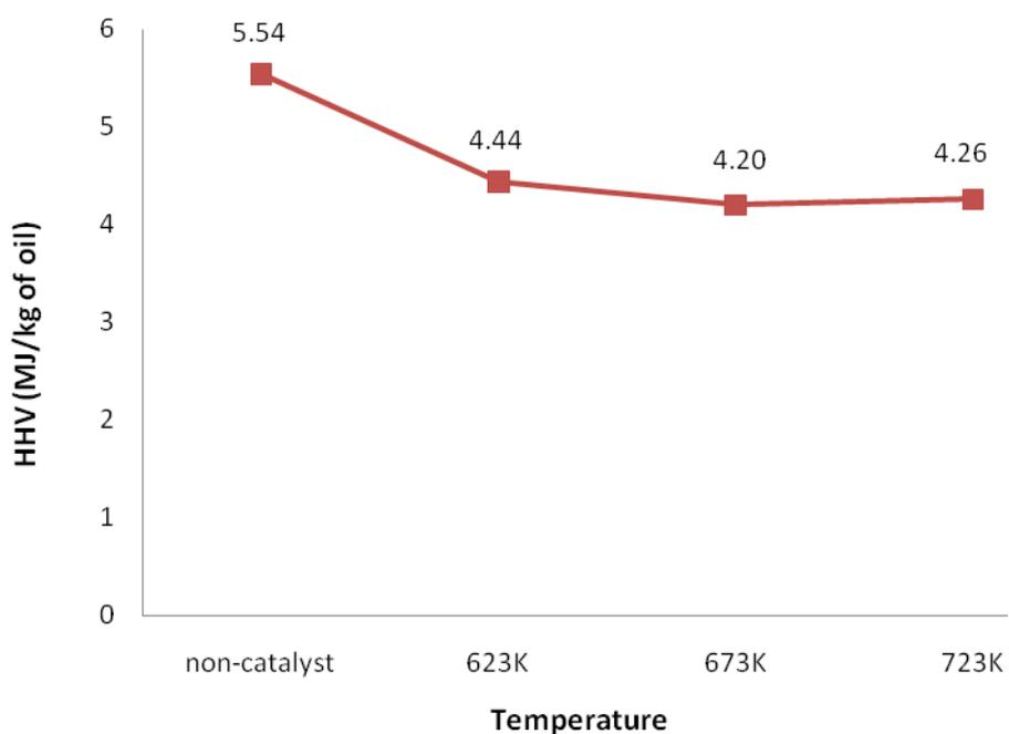
**Figure 22** High heating values (HHV) (MJ/kg) of aqueous phase of bio-oils upgraded by different temperatures; 623, 673 and 723K
