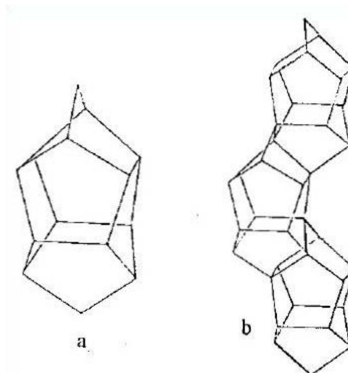
**Figure 5** HZSM-5 building unit (a) Secondary Building Units (SBUs) of HZSM-5
