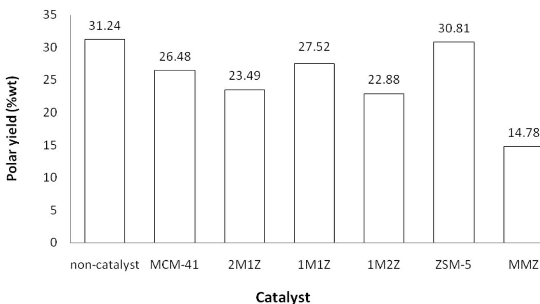
**Figure12** Polar fraction in the organic phase of bio-oil (%wt) from non-catalyst reaction and bio-oil upgraded by MCM-41, HZSM-5, MMZ and the blend of MCM-41 and HZSM-5 with the ratios of 1:1 (1M1Z), 1:2(1M2Z) and 2:1(2M1Z)
