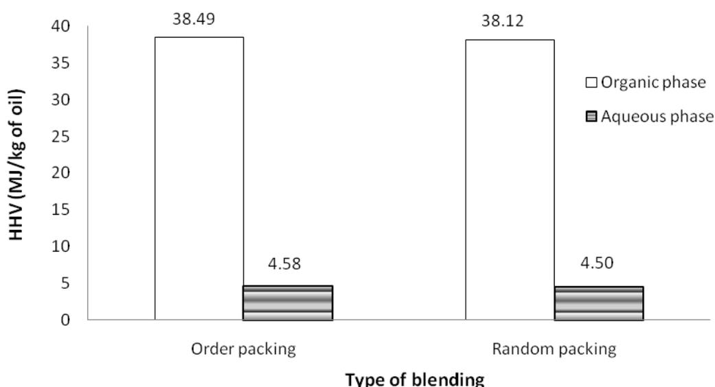
**Figure 18** High heating values (HHV) (MJ/kg) of bio-oils upgraded by different sequences of catalysts packing; order packing, random packing and order packing of MMZ with MCM-41
