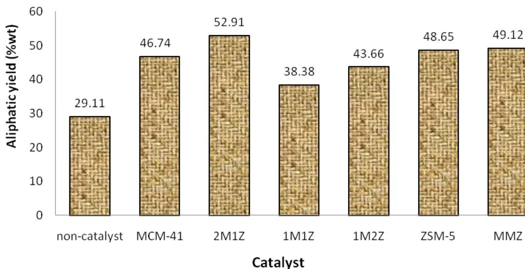
**Figure 10** Aliphatic fraction in the organic phase of bio-oil (%wt) from non-catalyst reaction and bio-oil upgraded by MCM-41, HZSM-5, MMZ and the blend of MCM-41 and HZSM-5 with the ratios of 1:1 (1M1Z), 1:2(1M2Z) and 2:1(2M1Z)
