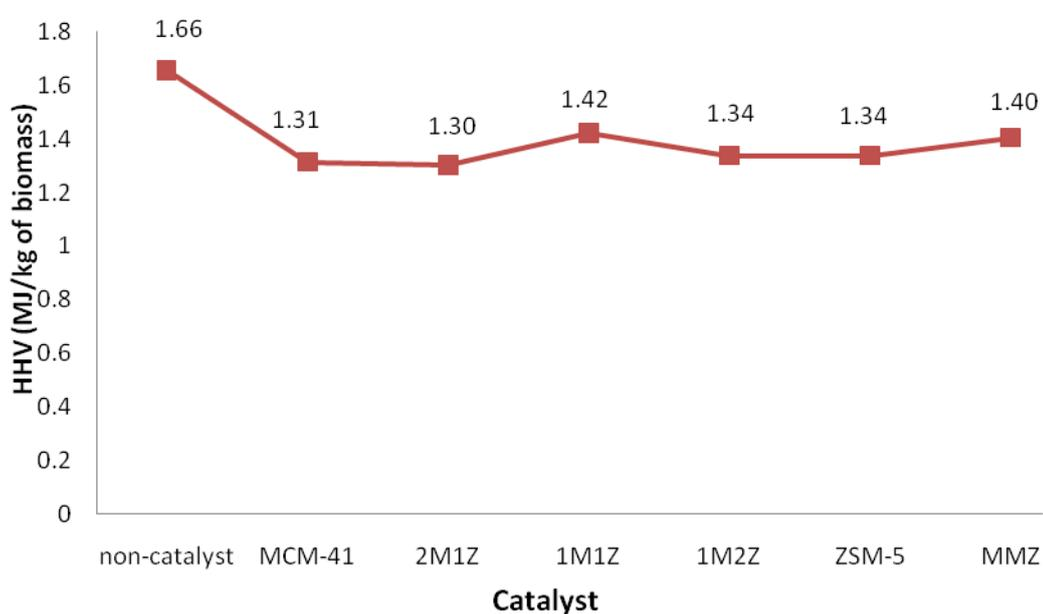
**Figure 15** Total energy output for the aqueous phase of bio-oil (MJ/kg of biomass) from non-catalyst reaction and bio-oil upgraded by MCM-41, HZSM-5, MMZ and the blend of MCM-41 and HZSM-5 with the ratios of 1:1 (1M1Z), 1:2(1M2Z) and 2:1(2M1Z)
