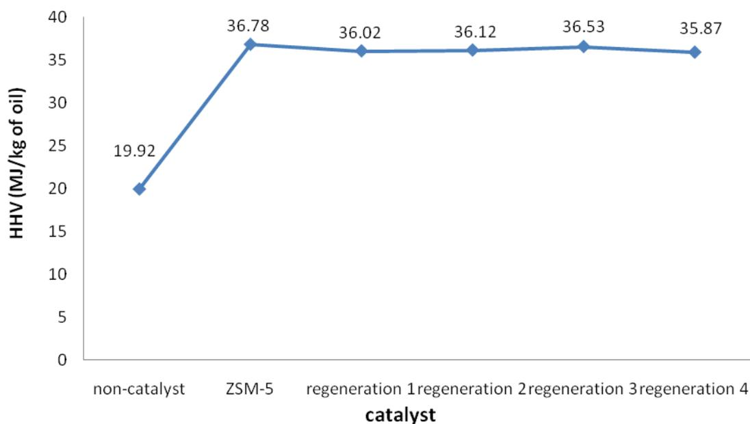
**Figure 39** High heating values (HHV) (MJ/kg) of organic phase of bio-oils upgraded by fresh and regenerated HZSM-5 at 673K
