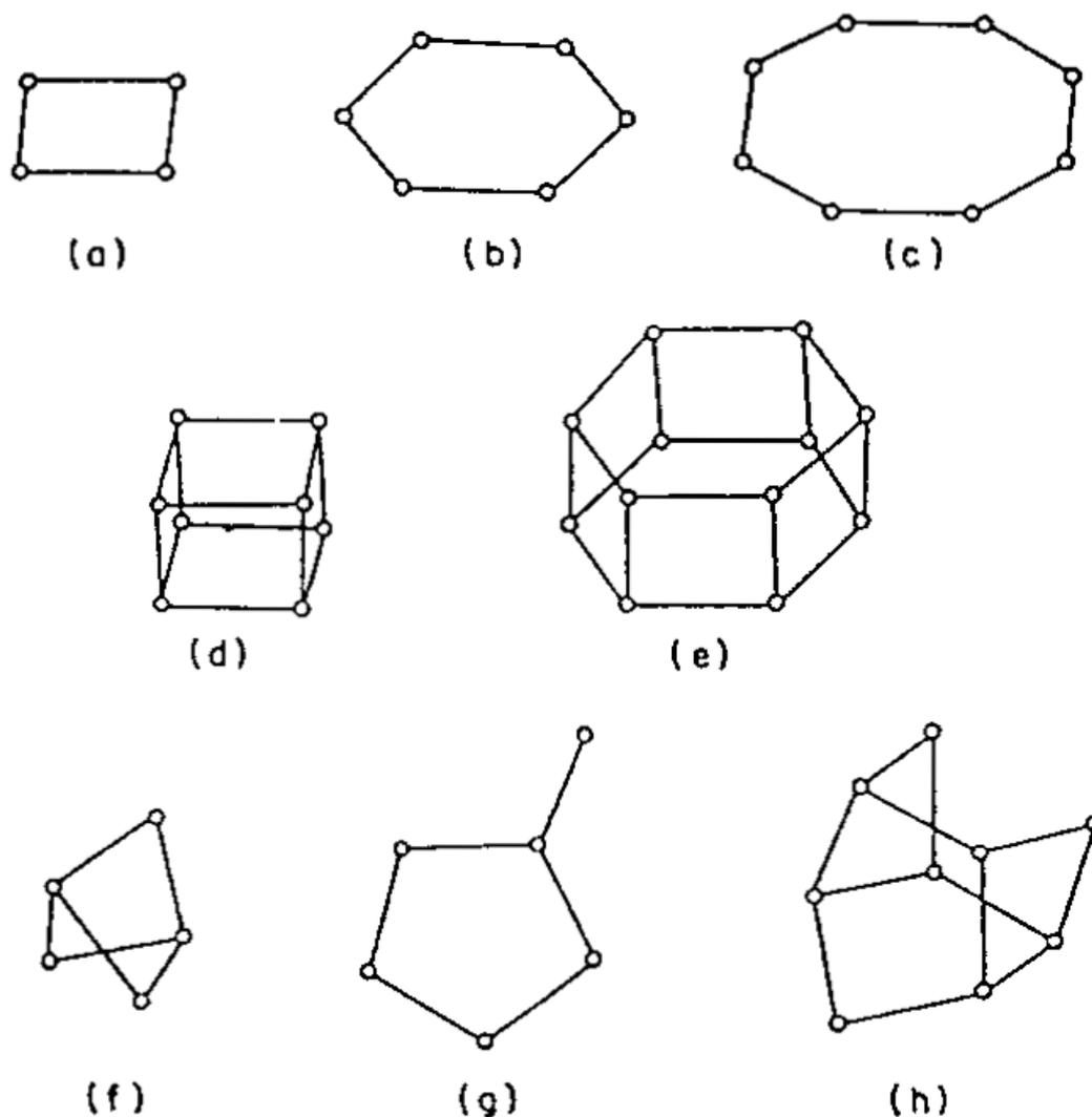
**Figure 4** Secondary building Units (SBUs) of zeolite structure (a) single four rings (S4R), (b) single six rings (S6R), (c) single eight rings (S8R) (d) double four rings (D4R) (e) double six rings (D6R) (f) complex 4-1 (g) complex 5-1 (h) complex 4-1-1
