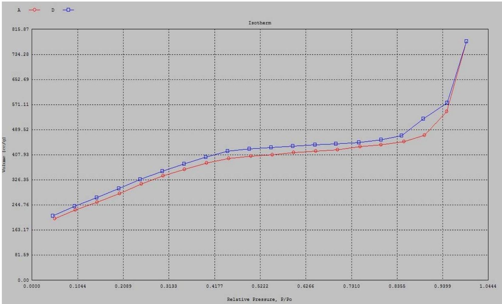
Appendix Figure C1 Adsorption and desorption isotherm of MCM-41
