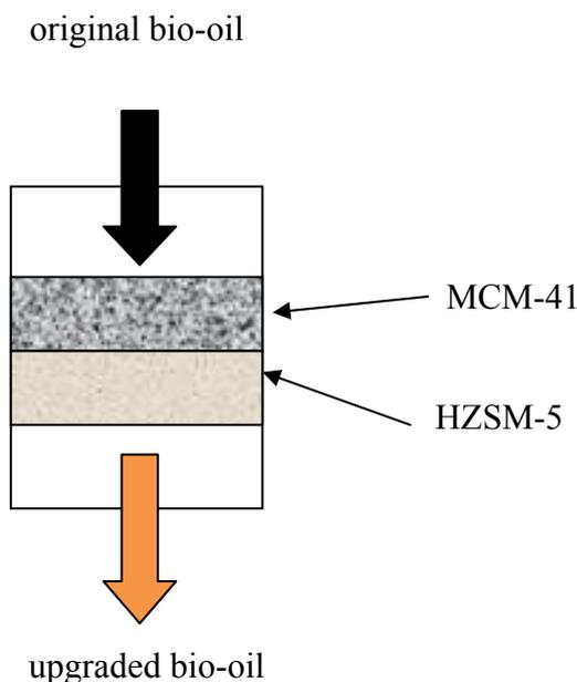
**Figure 17** Order packing of MCM-41 followed by HZSM-5 in a pack bed tube reactor
