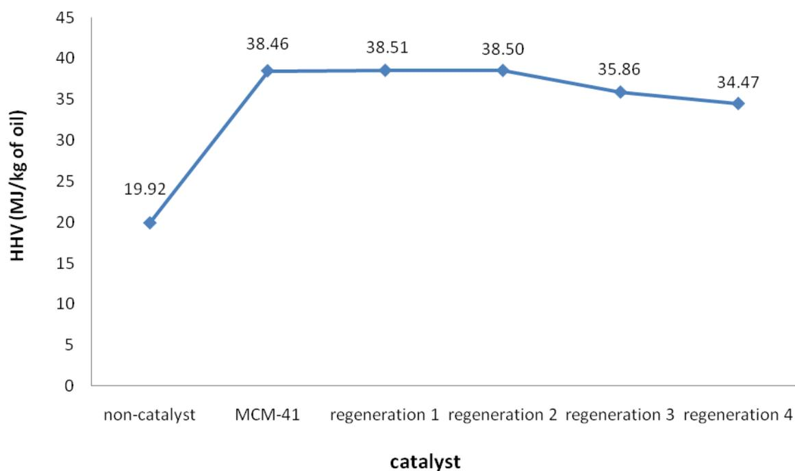
**Figure 30** High heating values (HHV) (MJ/kg) of organic phase of bio-oils upgraded by fresh and regenerated MCM-41 at 673K
