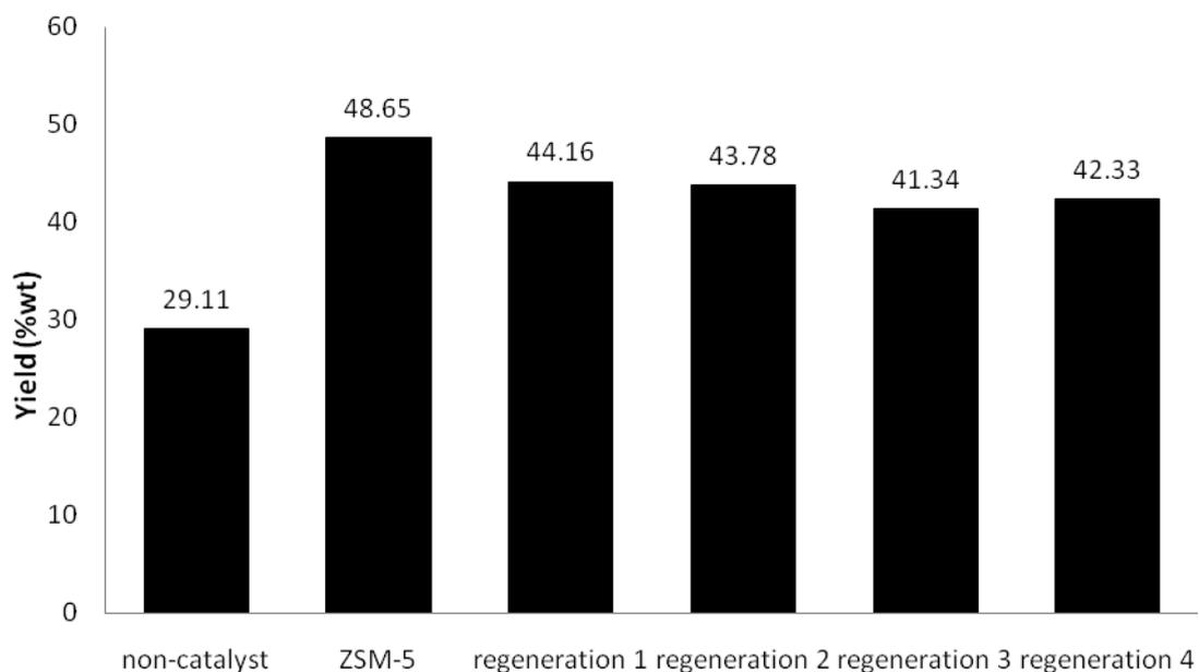
**Figure 41** Aliphatic fractions (%wt) of organic phases of bio-oils upgraded by fresh and regenerated HZSM-5 at 673K
