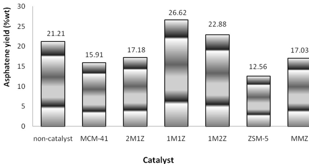
**Figure13** Asphaltene fraction in the organic phase of bio-oil (%wt) from non-catalyst reaction and bio-oil upgraded by MCM-41, HZSM-5, MMZ and the blend of MCM-41 and HZSM-5 with the ratios of 1:1 (1M1Z), 1:2(1M2Z) and 2:1(2M1Z)
