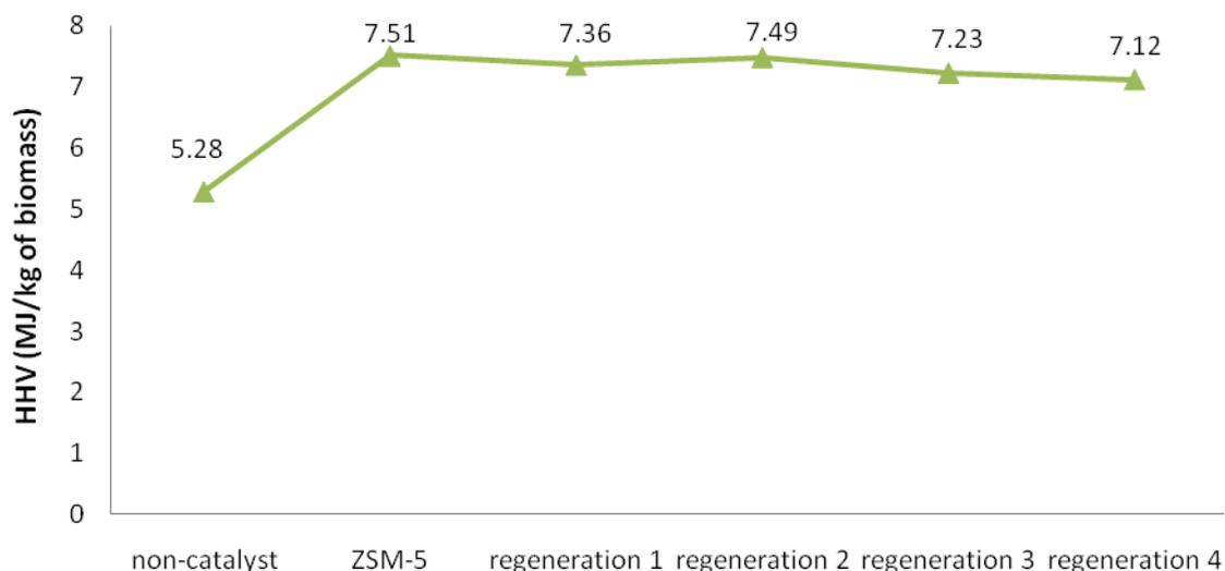
**Figure 47** Total energy output (MJ/kg of biomass) of bio-oils (both of organic and aqueous phase) upgraded by fresh and regenerated HZSM-5 at 673K
