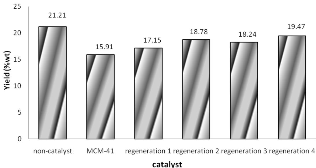
**Figure 35** Asphaltene fraction (%wt) of organic phase of bio-oils upgraded by fresh and regenerated MCM-41 at 673K
