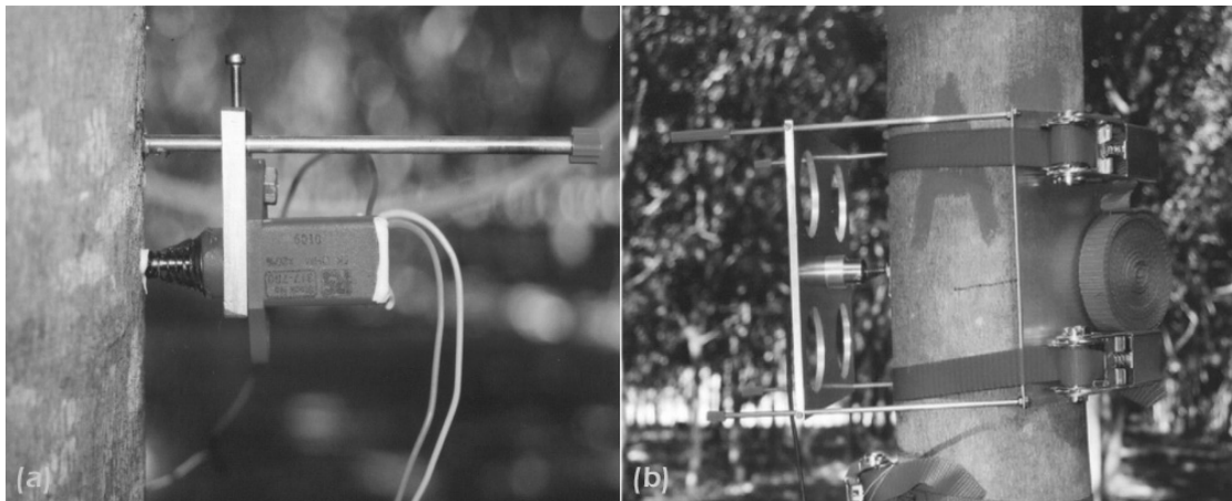
Figure 2 The feature of the two sensors for monitoring trunk radial increment
