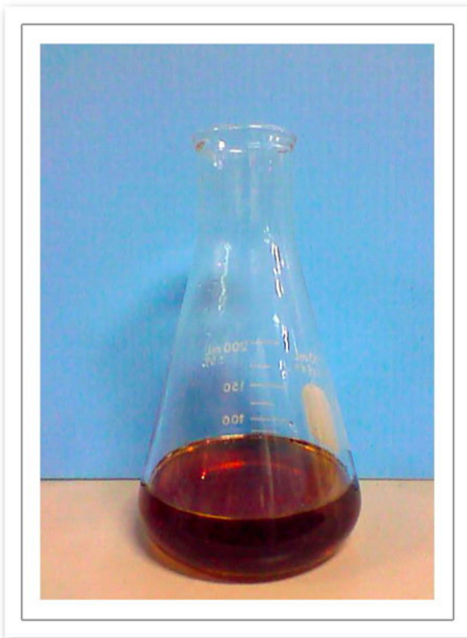
Figure 15 A trap grease biodiesel from two-step catalyzed process.
