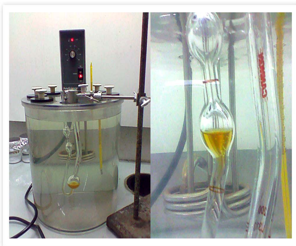
Figure 8 Kinematic viscosity of trap grease biodiesel using Ubbelohde glass capillary viscometer
