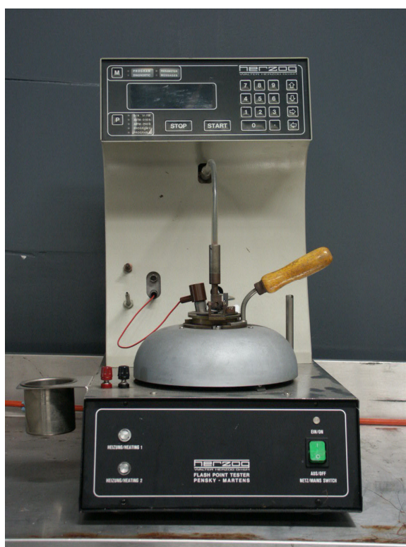
Figure 7 Pensky-Martens closed flash tester
