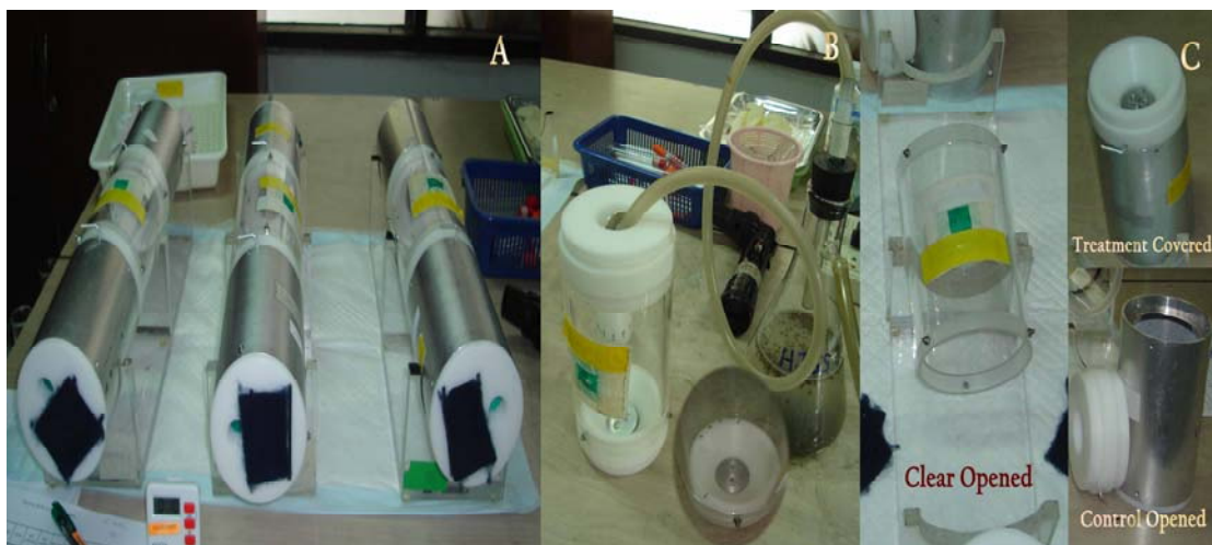
Figure 17 Spatial repellency assay procedures: test preformed (A) a metal chamber containing treated netting is attached to clear cylinder that is attached to a metal chamber housing a solvent-treated netting strip, (B) mosquitoes aspirated from clear chamber at end of 10 min assay, (C) the control chamber and clear cylinder are allowed to ventilate for 3 min between each replicate.
