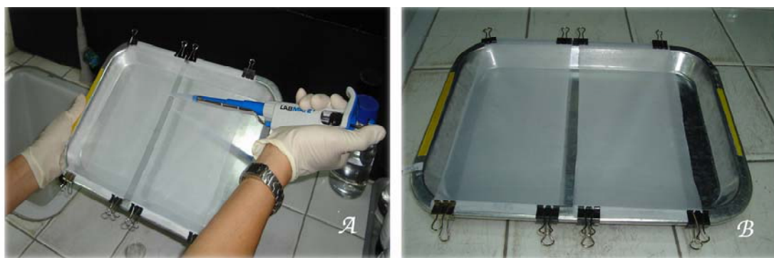
Figure 14 Insecticide impregnation of netting strips for the high-throughput screening system assay. (A) chemical application of 1.5 ml solution using a micropipette, (B) netting strips are allow to dry for 15 min before use in assay.
