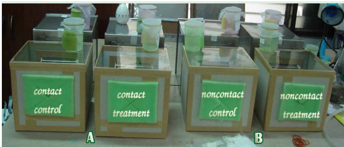
Figure 13 Excito-repellency assay showing one test series that consisted of (A) contact, (B) noncontact trial.
