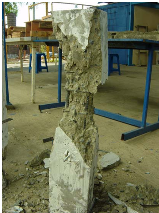
Figure 23 Covering spalling at ultimate load RB6(7.5)
