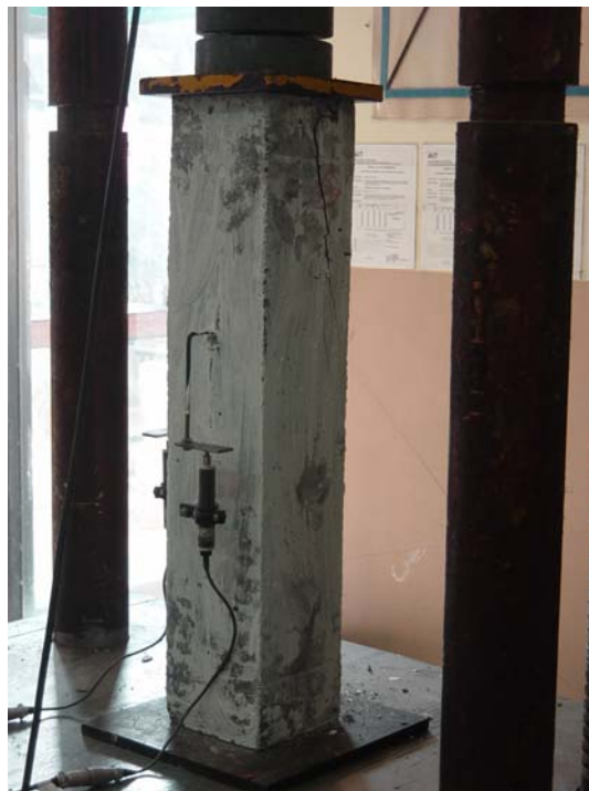
Figure 21 Tiny cracks occurring at 70 – 80 % of peak load (RB6(7.5))
