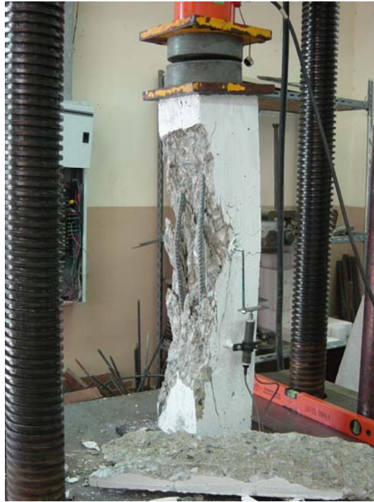
Figure 20 Column exploded after reaching ultimate load (No Tie bar column)
