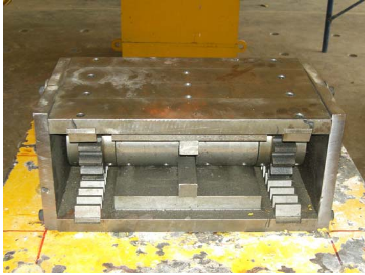
Appendix Figure C11 Hinge and roller support
