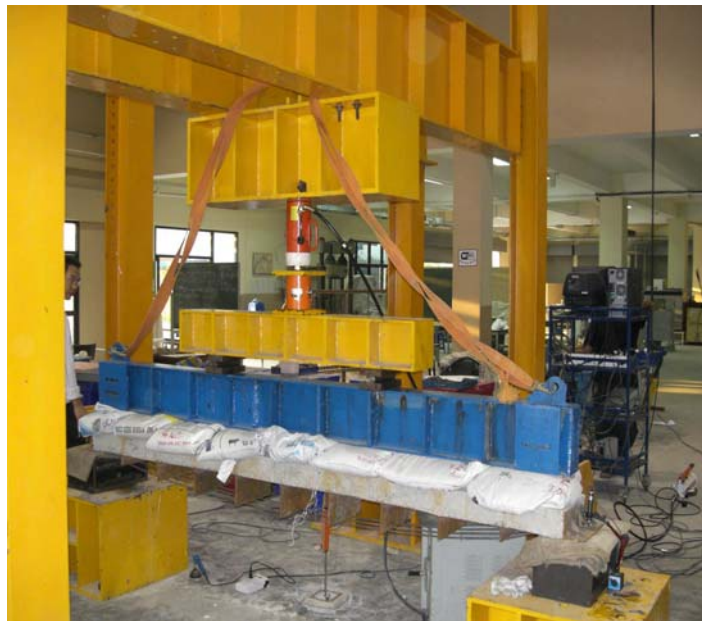
Appendix Figure C8 Set-up specimen for testing
