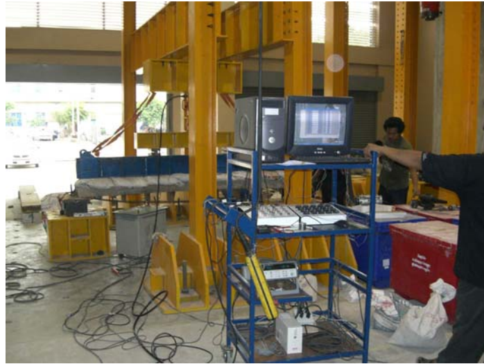
Appendix Figure C9 Strain and deflection read by the computer
