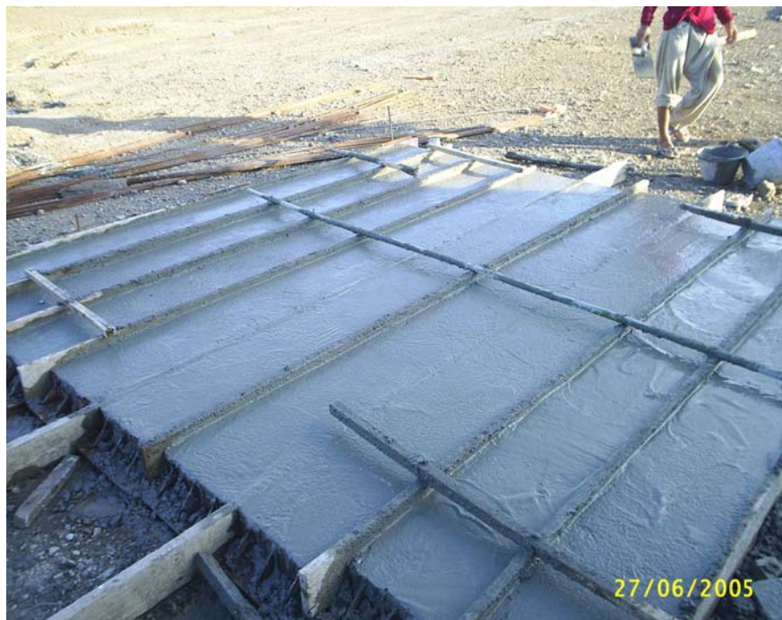
Appendix Figure C6 Specimens' preparation before curing
