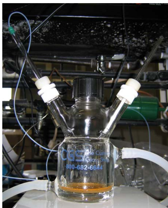
Figure 8 Purge and trap vessel for dynamic headspace sampling of chili paste
