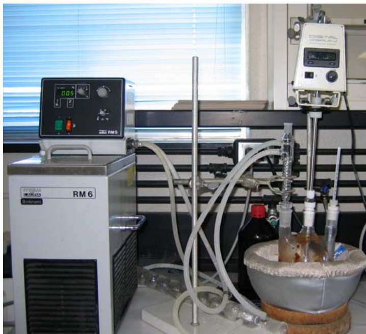
Figure 7 Apparatus used for heating of chili paste
