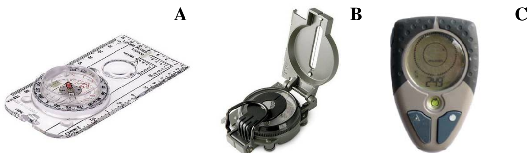
Figure 3 Base-plate map compass (A), lensatic sighting compass (B) and digital compass (C)
