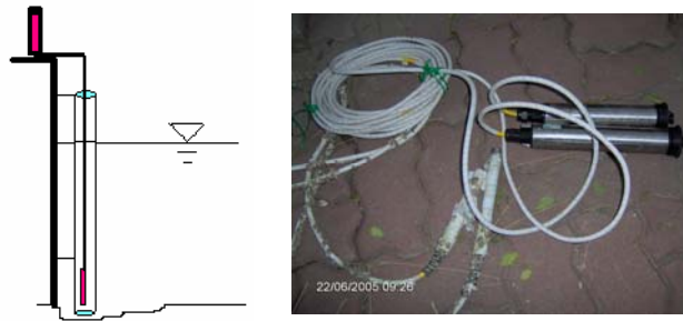
Figure 3 Observing seawater level design by using Global water WL 15 Water Logger
