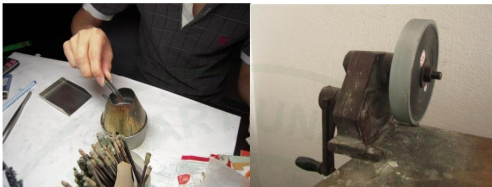
**Figure 19** Sticking sample with the sample holder bar (left) then truncated by Thai local-made trim machine (right) at Department of Earth Sciences, Faculty of Science, Kasetsart University.
