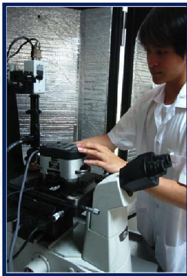
**Figure 24** Atomic Force Microscope model MFP-3D-BIO AFM from Asylum Research based at the Scientific Equipment Center, Faculty of Science Kasetsart University, Bangkok.
