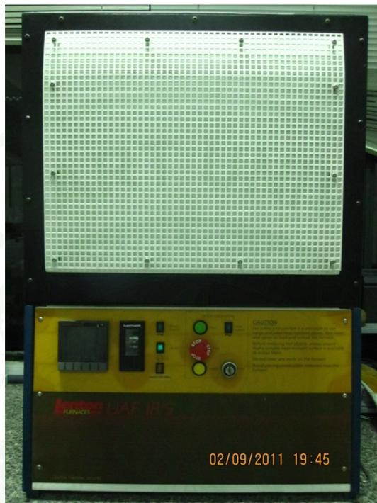
**Figure 21** The high temperature electric furnace; Lenton, model UAF18/5 at Department of Earth Sciences, Kasetsart University, Bangkok
