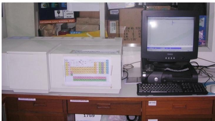
**Figure 23** UV-Vis-NIR spectroscopy Perkin Elmer model LAMDA 900 placed at Department of Earth Sciences, Faculty of Science, Kasetsart University.
