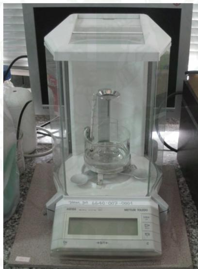
**Figure 14** An electronic balance for measuring S.G. at Department of Earth Sciences, Faculty of Science, Kasetsart University
