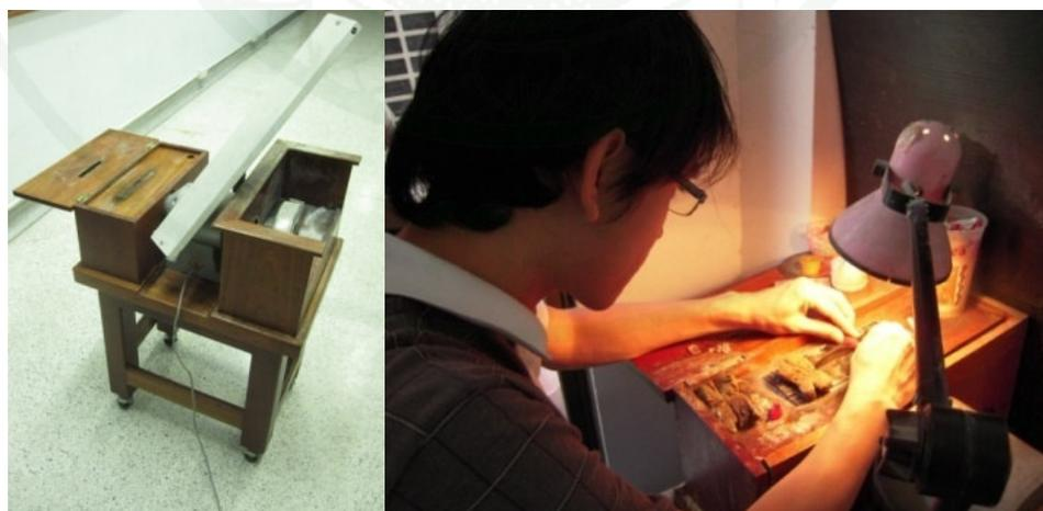
**Figure 18** Thai sawing and grinding machines for sample cutting at Department of Earth Sciences, Faculty of Science, Kasetsart University.
