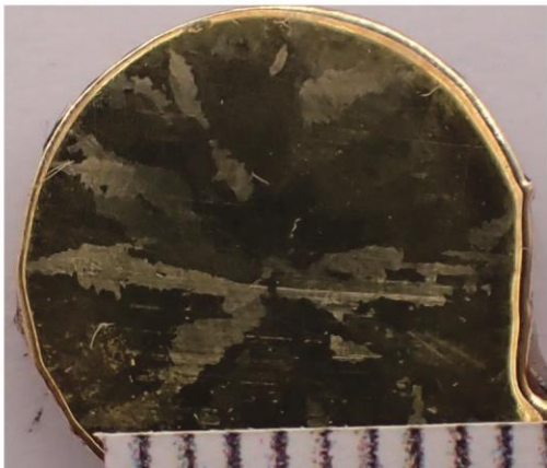
4/5)Cu15Zn3Sn-Zr grain size 1.2 mm
