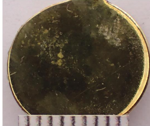
4/9)Cu15Zn3Sn-FeZr grain size 0.6 mm
