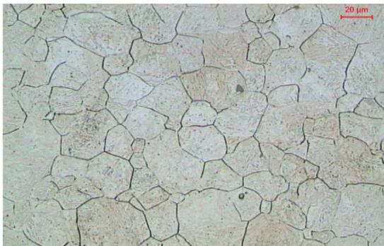
Figure 1. Revealing prior-austenite grain boundaries in an as-cast low alloy structural steel (40Cr8) with contents of micro-alloying elements, V, Nb and Ti, heat treated with austenitizing for 30 min in argon atmosphere at temperature in the range of 840-1,200 °C and quenching in water.
