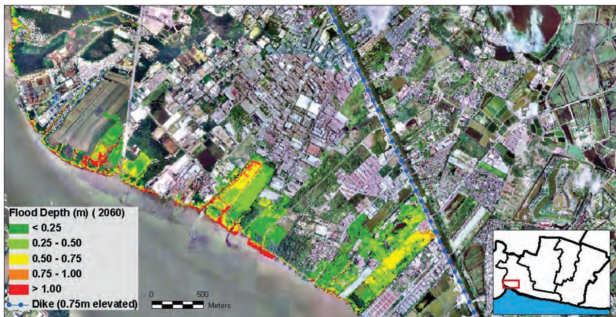
Fig.4 A sub-area enlarged here demonstrating that area behind dike (right of blue solid-dotted line) is effectively protected if the dike is elevated by 0.75 m.
