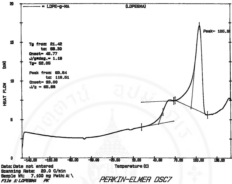
Figure A2 DSC thermogram of PE-g-MA
