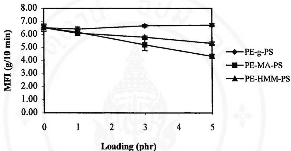
**Figure 3.42** MFI of 75:25 LDPE/PS blends filled with various loadings of PE-g-PS, PE-MA-PS and PE-HMM-PS
