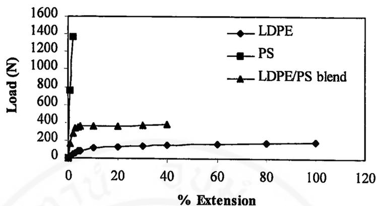
**Figure 3.24** Stress-strain behaviour of LDPE, PS and 75:25 LDPE/PS
