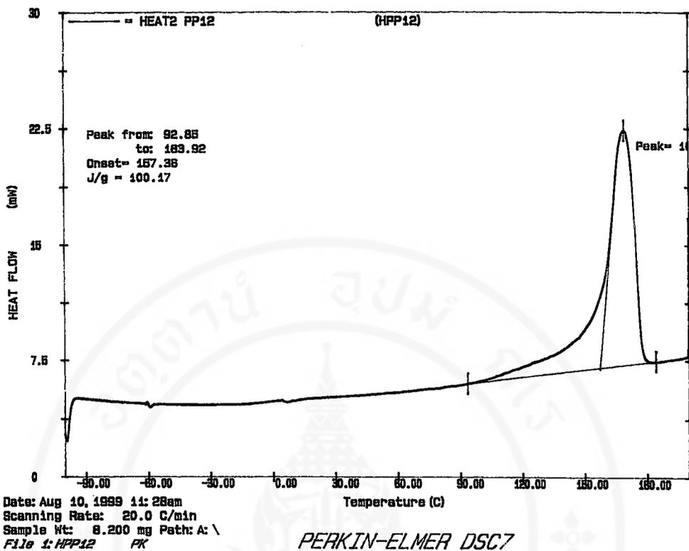
Figure A14 DSC thermogram of PP12
