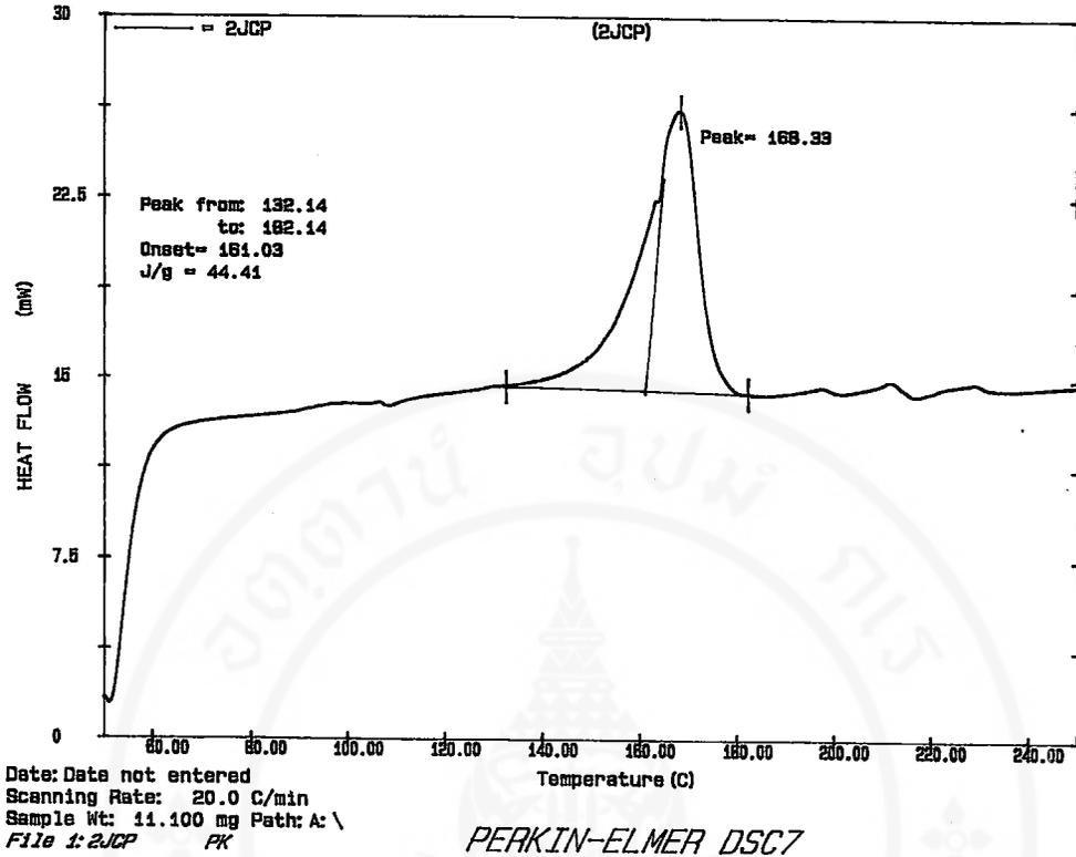
Figure A18 DSC thermogram of 2SP3.5
