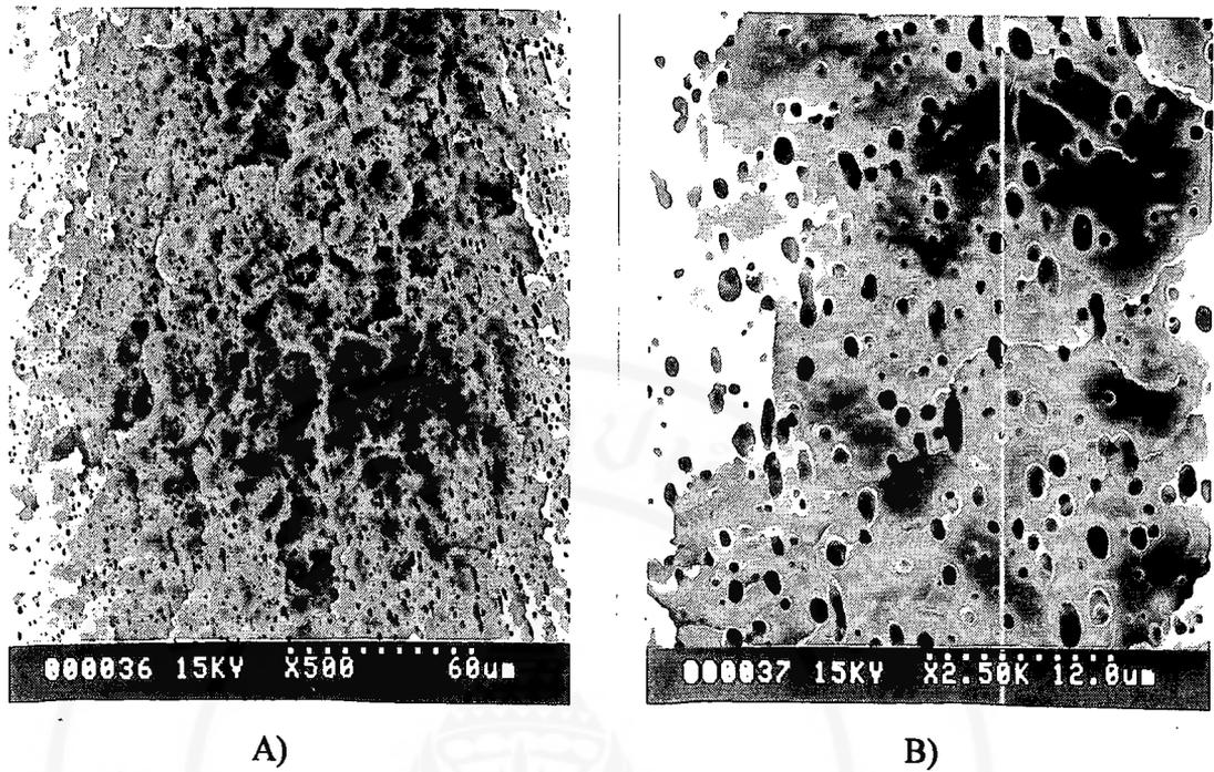
**Figure D14** SEM micrograph of 75:25 LDPE/PS blend with 2SP55 3 phr:
