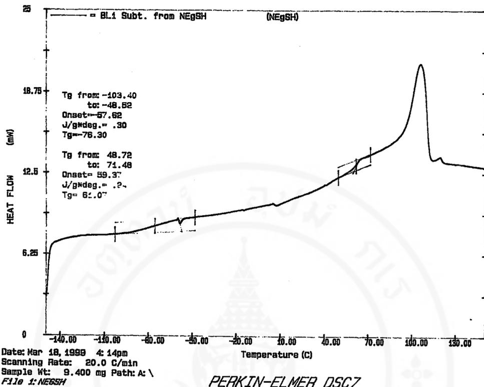
Figure A6 DSC thermogram of PE-HMM-PS
