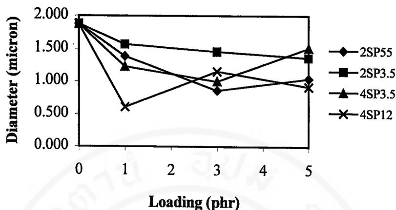
**Figure 3.39** Average particle size of blends containing PP-*co*-PS
