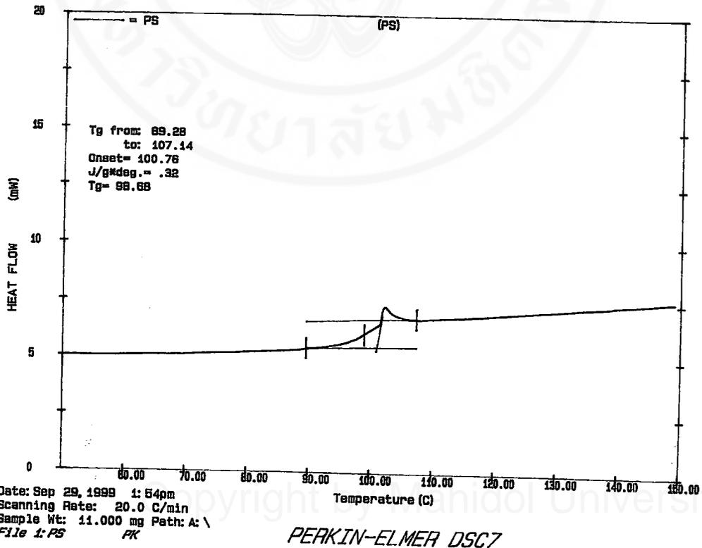
Figure A3 DSC thermogram of PS
