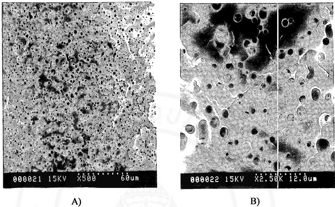
**Figure D16** SEM micrograph of 75:25 LDPE/PS blend with 2SP3.5 1 phr:
