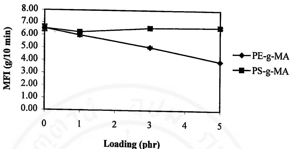
**Figure 3.41** MFI of 75:25 LDPE/PS blends filled with various loadings of PE-g-MA and PS-g-MA
