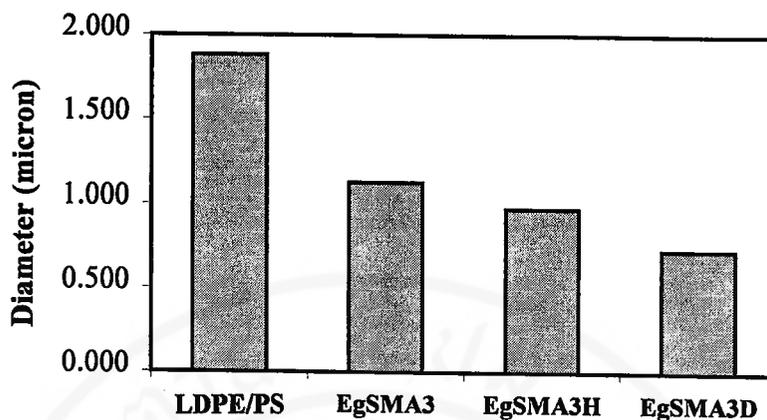
**Figure 3.40** Average particle size of the blends containing both PE-*g*-MA, PS-*g*-MA with and without diamine compounds
