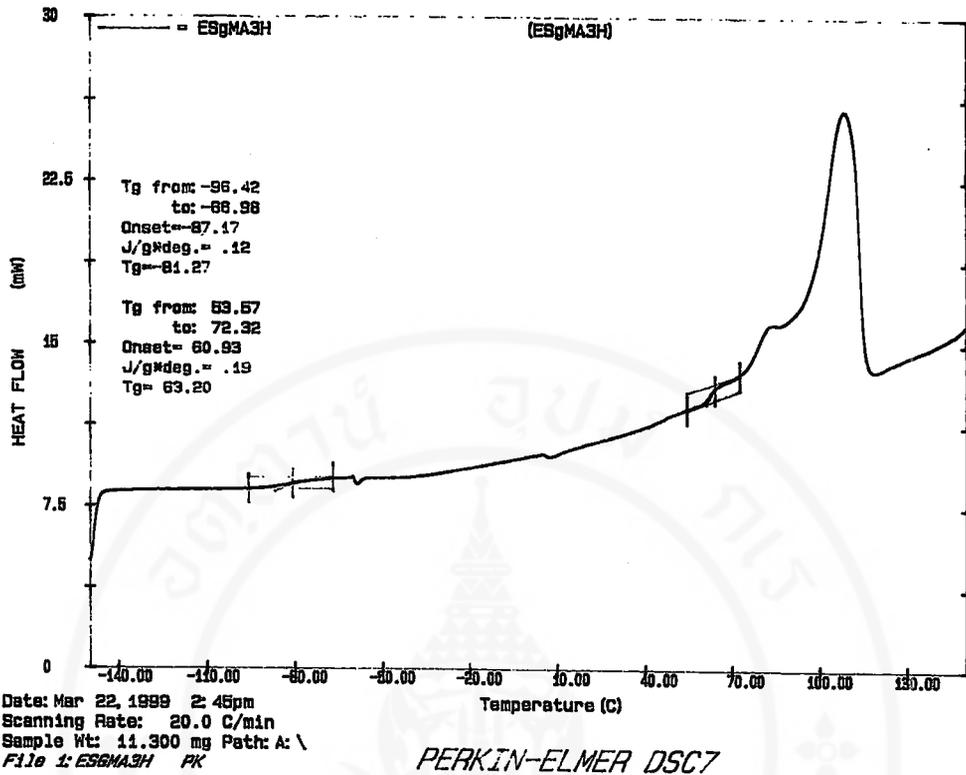
Figure A10 DSC thermogram of EgSMA3H
