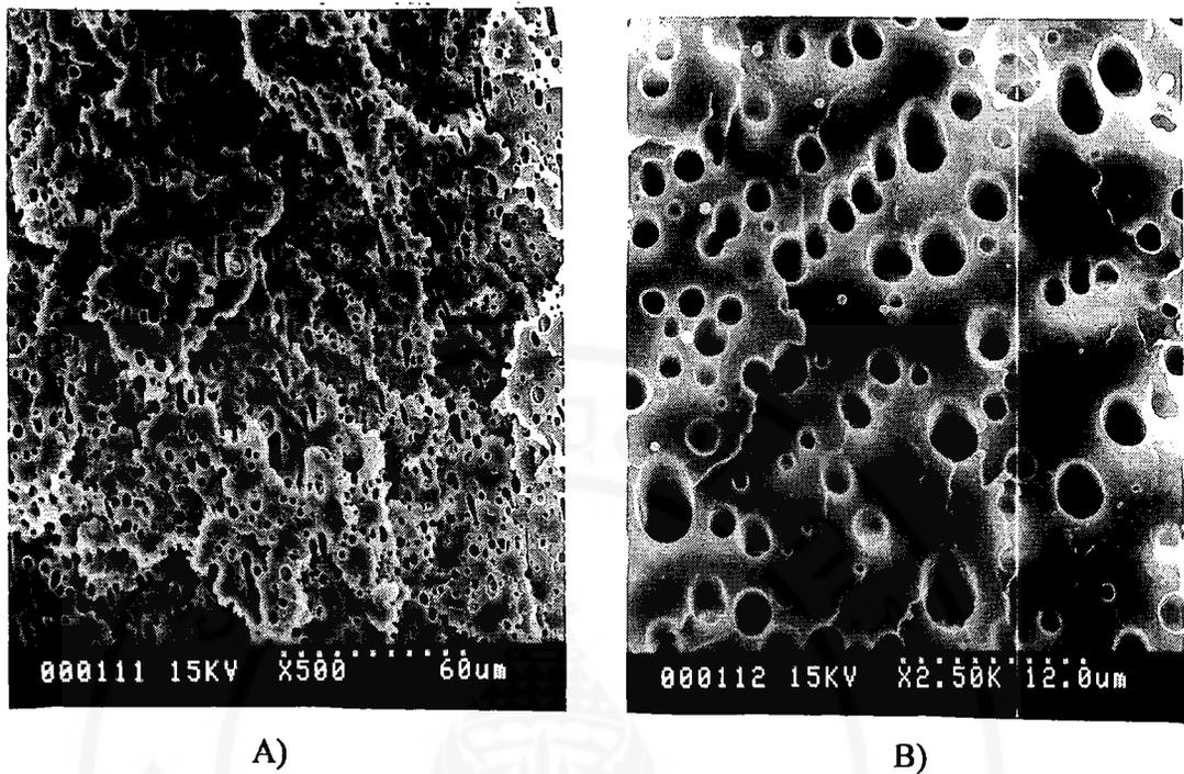
**Figure 3.36** SEM micrograph of 75:25 LDPE/PS blend: A) x 500; B) x 2500
