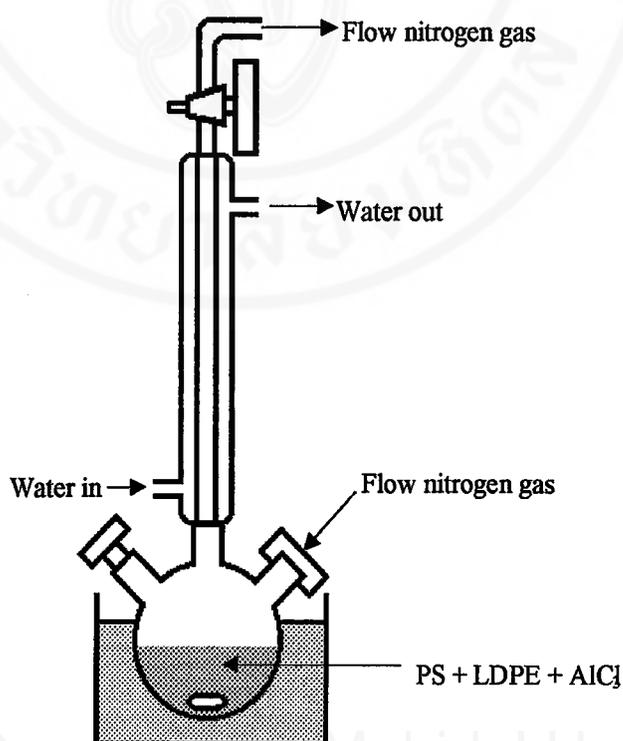
**Figure 2.1** Reaction apparatus for chemical modification of PS and LDPE by Friedel-Crafts alkylation
