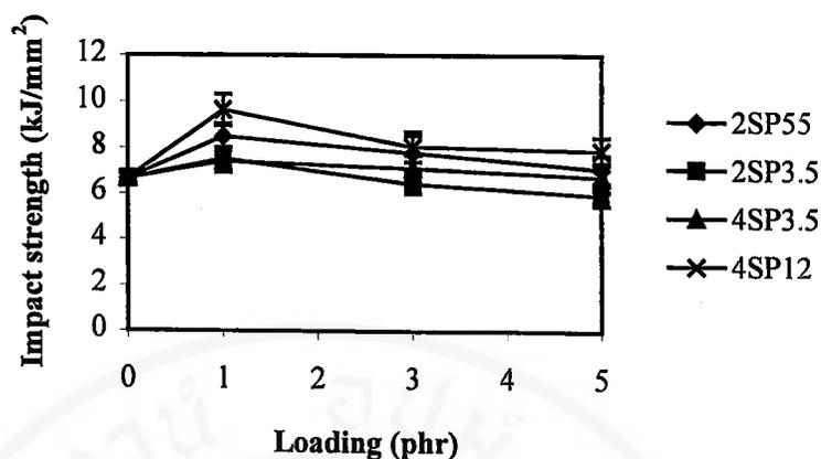
**Figure 3.31** Impact strengths of blends containing various types of PP-co-PS
