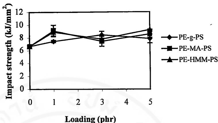
**Figure 3.29** Impact strength of blends containing various amounts of PE-g-PS, PE-MA-PS and PE-HMM-PS compatibilisers
