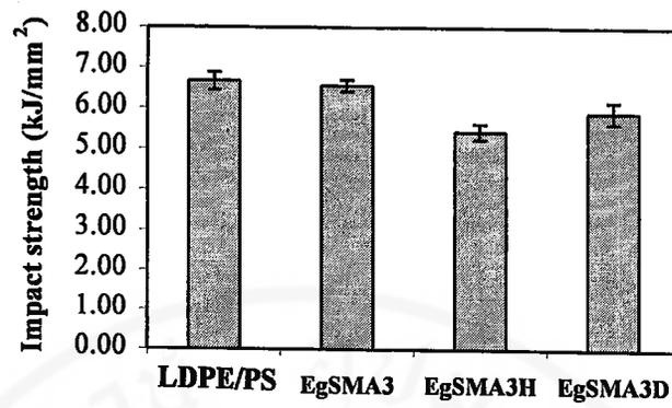
**Figure 3.35** Impact strengths of blends containing both of PE-g-MA and PS-g-MA with and without diamine compounds
