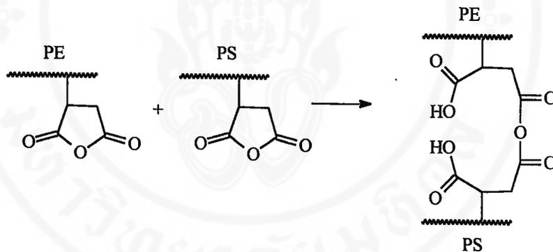
**Figure 3.33** Formation of acyclic anhydride in melt processing
