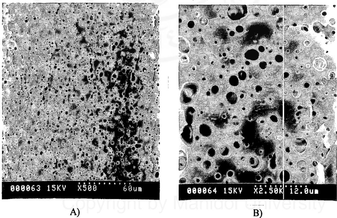
**Figure D23** SEM micrograph of 75:25 LDPE/PS blend with 4SP12 3 phr:
