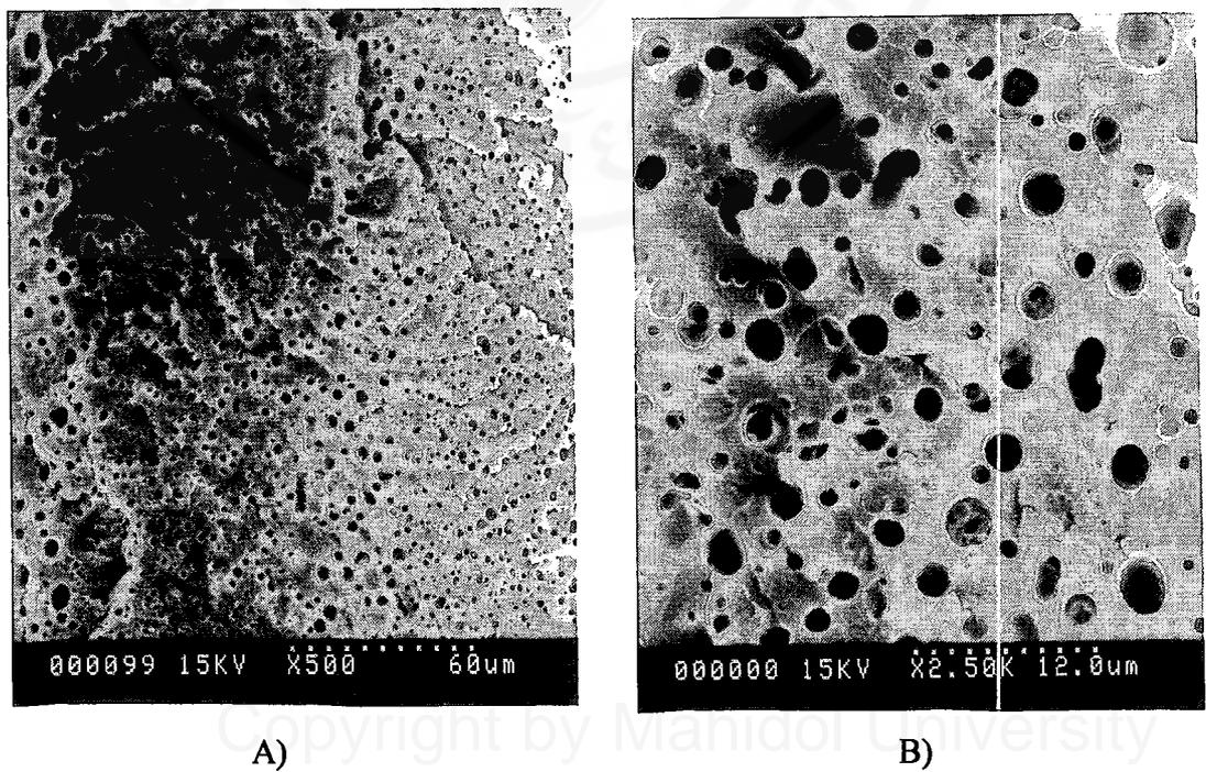
**Figure D17** SEM micrograph of 75:25 LDPE/PS blend with 2SP3.5 3 phr:
