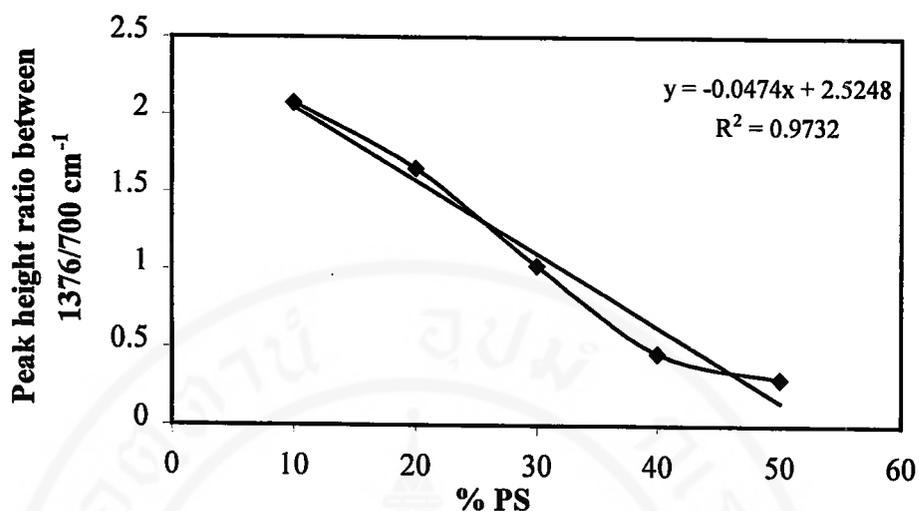
**Figure 3.22** Calibration curve of %PS versus peak height ratio between 1376 and 700 cm<sup>-1</sup> of PP/PS blends.
