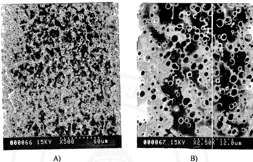
**Figure D24** SEM micrograph of 75:25 LDPE/PS blend with 4SP12 5 phr:
