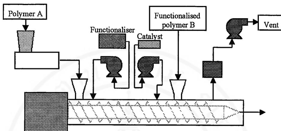
**Figure 1.3** Schematic of a sequential functionalisation/blending operation in extrusion equipment.
