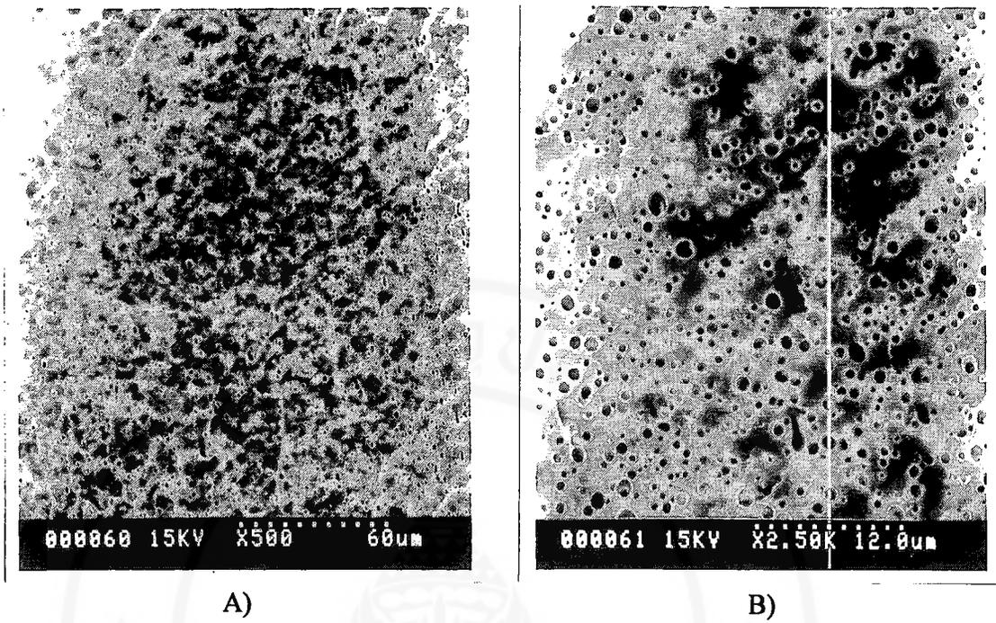
**Figure D22** SEM micrograph of 75:25 LDPE/PS blend with 4SP12 1 phr:
