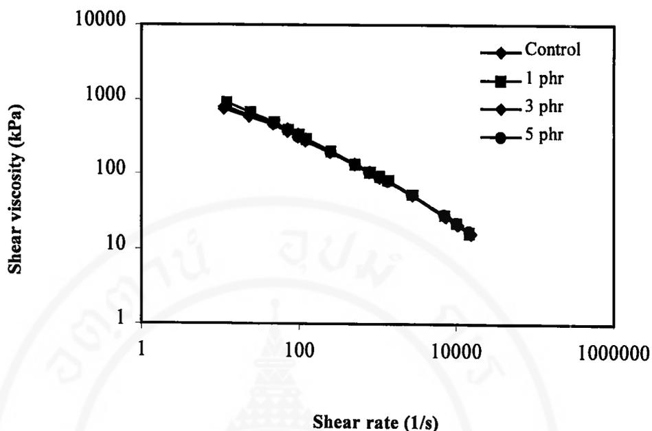
**Figure 3.50** Shear viscosity of 75:25 LDPE/PS blends with various loadings of 4SP12
