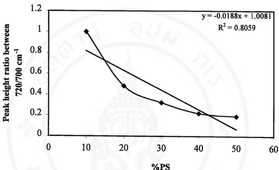
**Figure 3.15** Calibration curve of %PS versus peak height ratio between 720 and 700 cm<sup>-1</sup> in LDPE/PS blends
