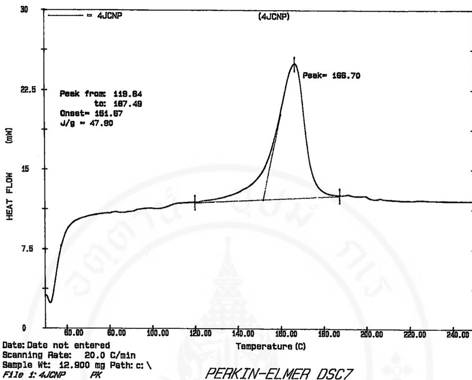
Figure A20 DSC thermogram of 4SP12
