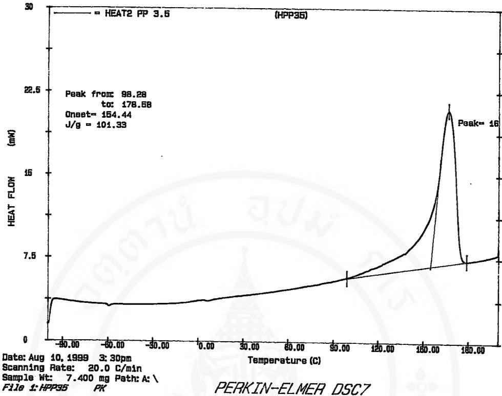
Figure A12 DSC thermogram of PP3.5
