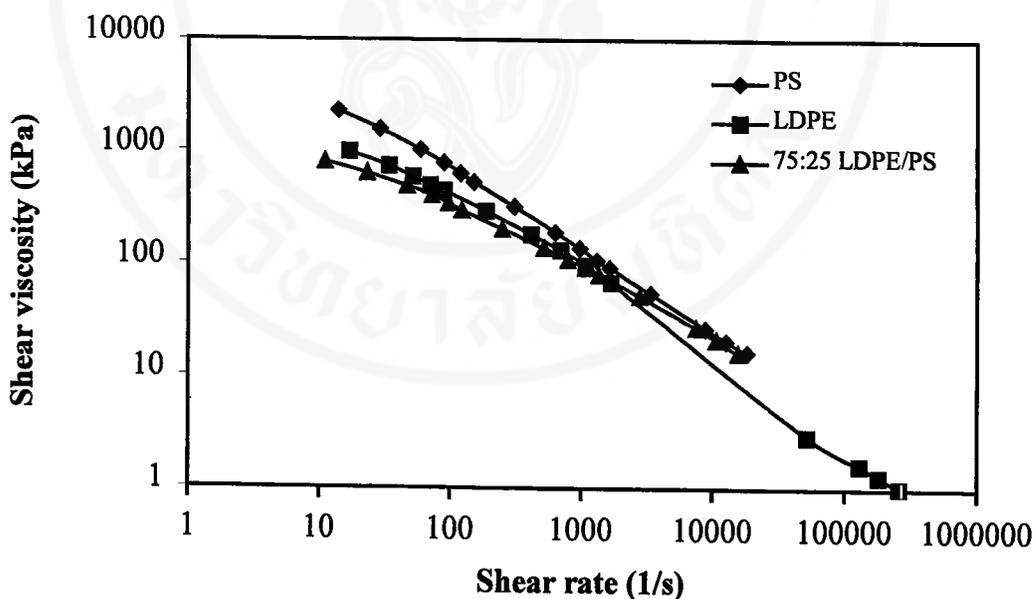
Figure 3.46 Shear viscosity of the homopolymer LDPE, PS and 75:25 LDPE/PS blends versus the shear rate
