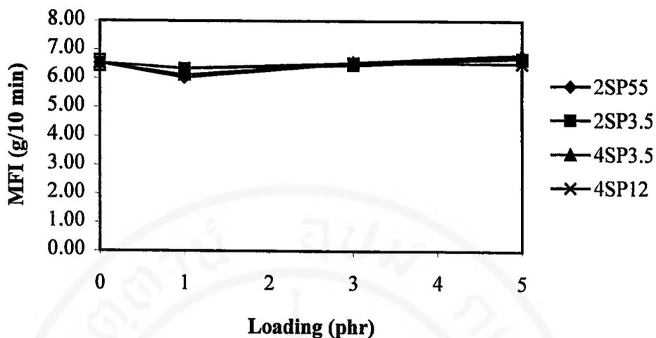
Figure 3.44 MFI of 75:25 LDPE/PS blends with various loadings of PP-co-PS
