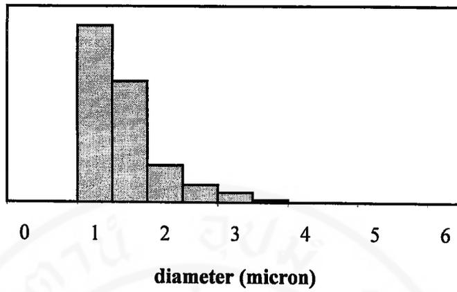
Figure C4. Particle size distribution of EgSMA3
