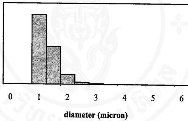
Figure C5. Particle size distribution the EgSMA3H
