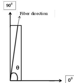
Figure 4. Fiber orientation on the mandrel.
