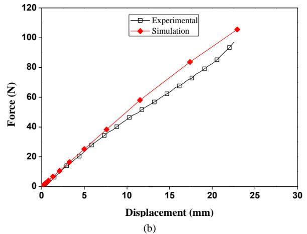
Figure 12. Load-displacement graphs of the experimental and finite element analysis for 70° fiber orientation O-shaped springs for (a) carbon and (b) glass.
