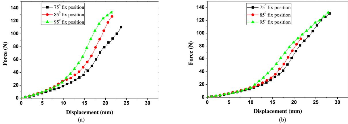
Figure 8. Different fixing positions for C-shaped springs: (a) carbon fiber springs and (b) glass fiber springs.
