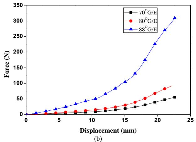
Figure 5. Three different fiber orientations for C-shaped springs: (a) carbon fiber springs and (b) glass fiber springs.
