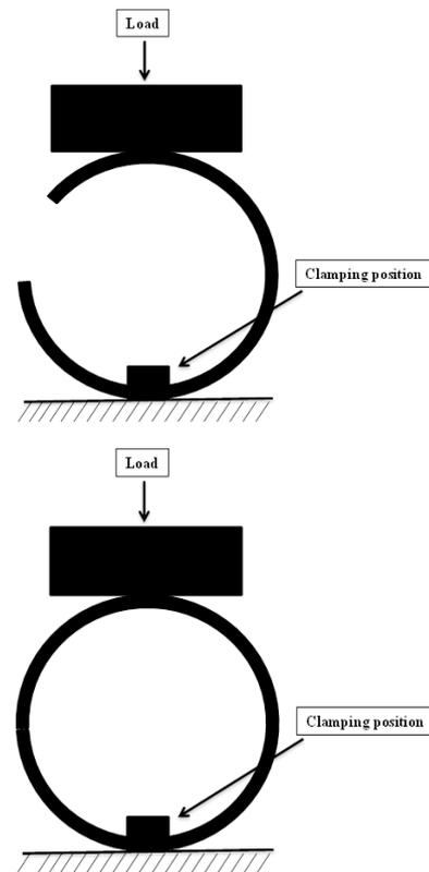
Figure 2. Experimental set up for C- and O-shaped springs.
