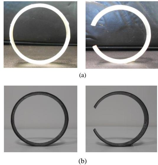
Figure 1. O-shaped and 45° cut C-shaped springs made of (a) glass fiber and (b) carbon fiber.
