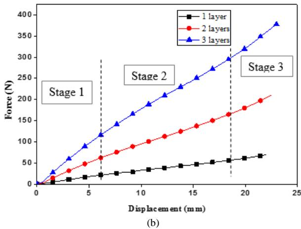
Figure 3. Graph of three different glass fiber layers: (a) C-shaped springs and (b) O-shaped springs.
