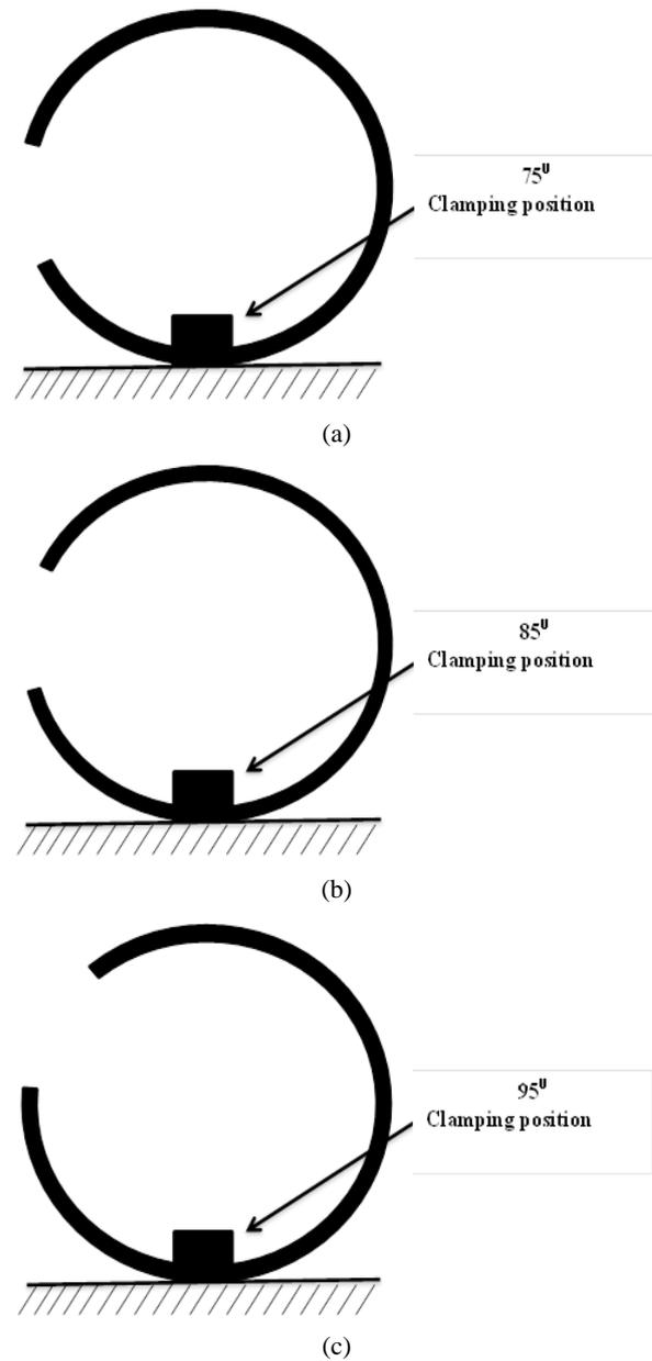
Figure 7. C-shaped springs: Clamping positions at (a) 75°, (b) 85°, and (c) 95°.
