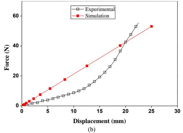
Figure 11. Load-displacement graphs of the experimental and finite element analysis for 70° fiber orientation C-shaped springs for (a) carbon and (b) glass.
