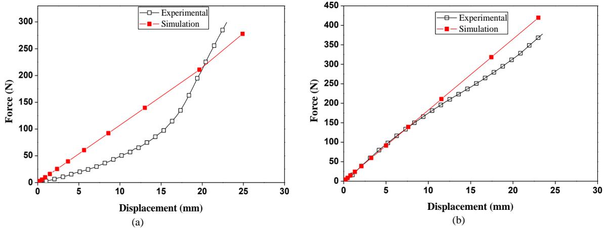
Figure 10. Load-displacement graphs for the combined experimental and finite element analysis of three layers for (a) C-shaped springs and (b) O-shaped springs.
