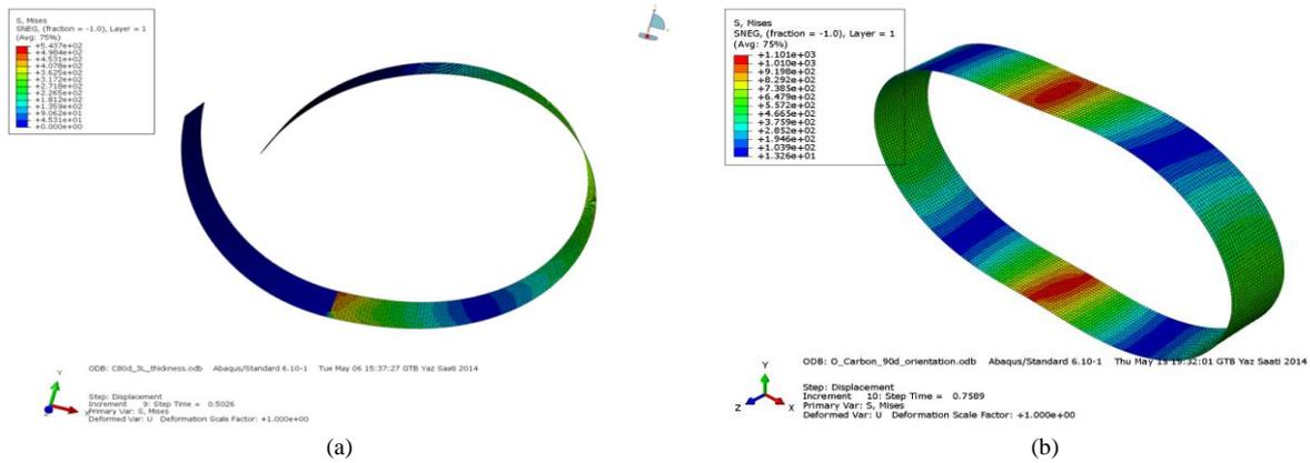
Figure 9. Von Mises equivalent stress for (a) C-shaped spring and (b) O-shaped spring.
